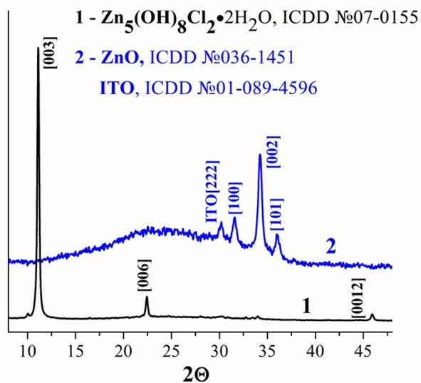
Figure S2. XRD pattern of as electrodeposited layered  $\text{Zn}_5(\text{OH})_8\text{Cl}_2 \cdot 2\text{H}_2\text{O}$  (curve 1), and  $\text{ZnO}$  (curve 2) formed after  $\text{Zn}_5(\text{OH})_8\text{Cl}_2 \cdot 2\text{H}_2\text{O}$  film calcination at  $450^\circ\text{C}$
