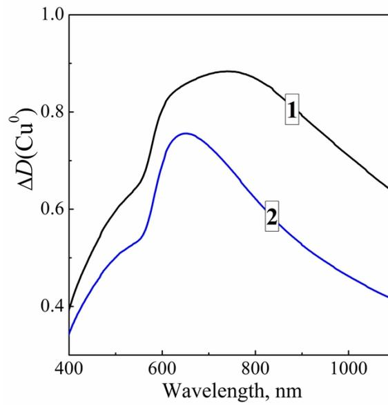
Fig. S11. Differential absorption spectra of Cu in FTO/ZnO/Cu films produced at 20% (curve 1) and 100% (2) UV light intensity. The spectra were obtained by subtracting absorption spectra of starting FTO/ZnO films.
