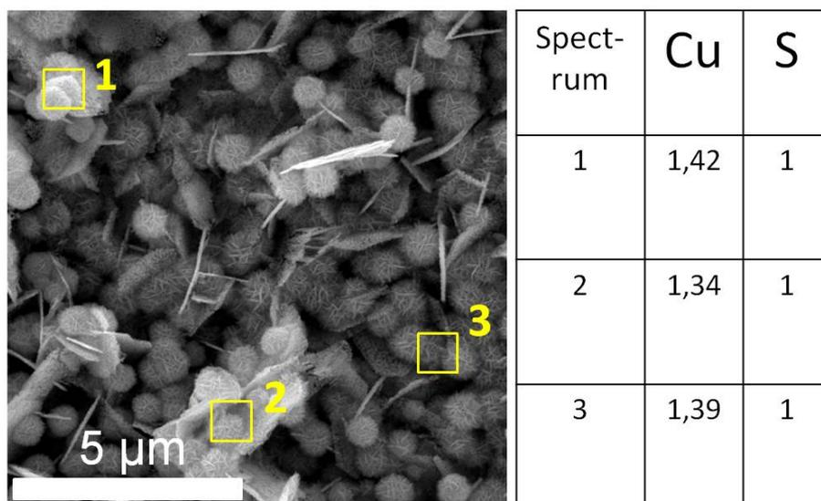
Figure S8. SEM image of FTO/ZnO/Cu<sub>x</sub>S film with three separate sections chosen for the EDX analysis (left part). Ratio of copper-to-sulfur atoms in the selected areas, according to the EDX analysis.
