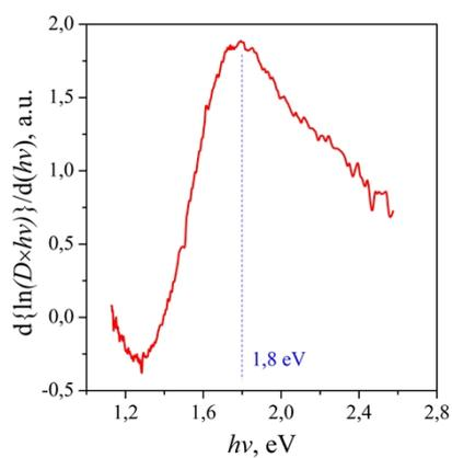
Figure S5. Absorption spectra of  $\text{Cu}_x\text{S}$  NPs in the film FTO/ZnO/ $\text{Cu}_x\text{S}$  in coordinates of differential form of Tauc equation for  $\text{Cu}_x\text{S}$  band gap determination.
