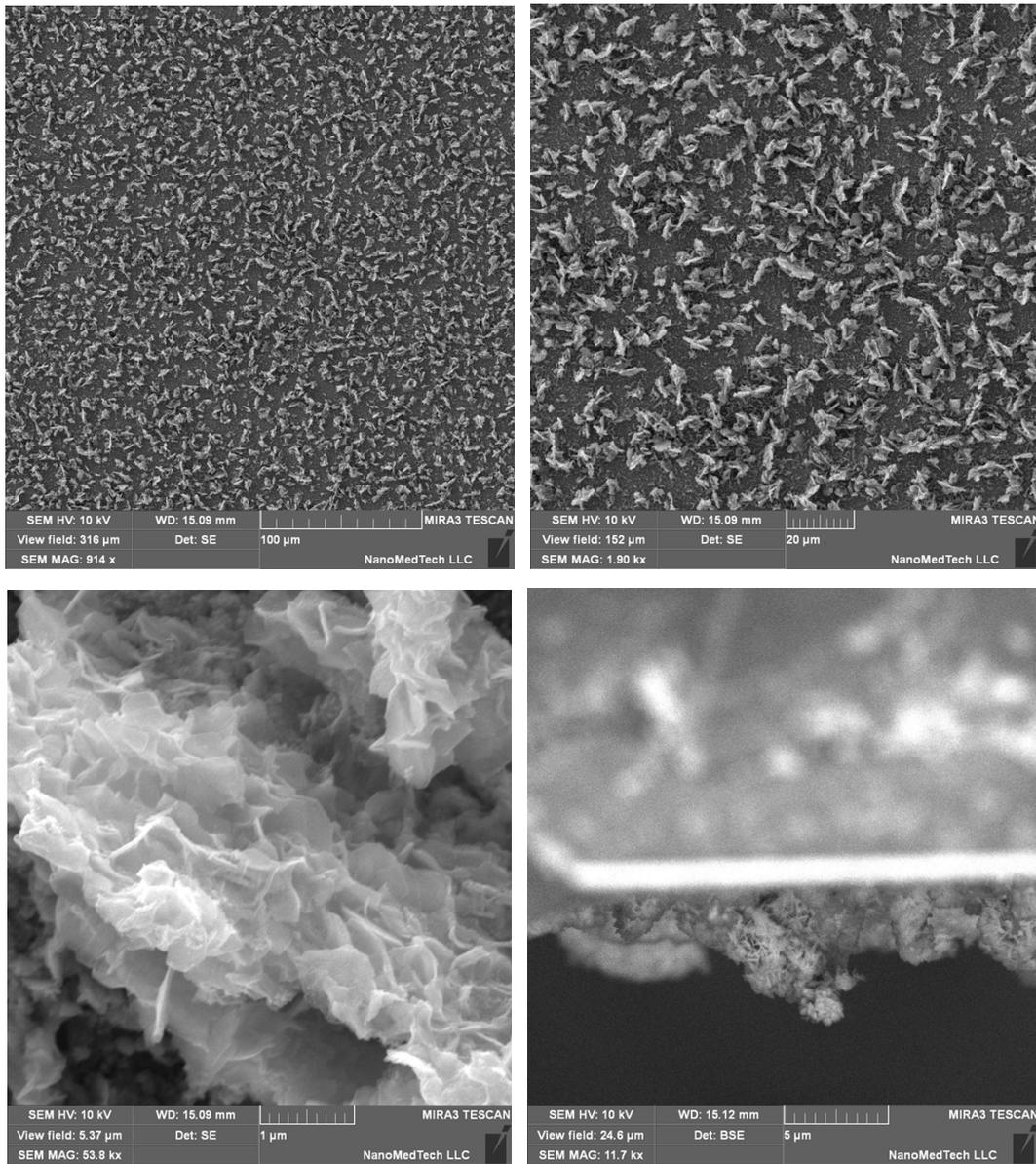
Figure S7. SEM images of FTO/ZnO/Cu<sub>x</sub>S films produced by partial sulfidation of zinc oxide followed with substitution of Zn(II) in ZnS with copper ions (see in more details in [23]).
