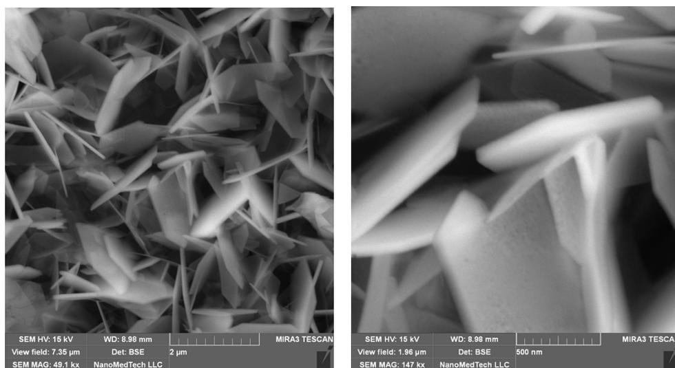
Figure S3. SEM images of FTO/ $\text{Zn}_5(\text{OH})_8\text{Cl}_2$  films
