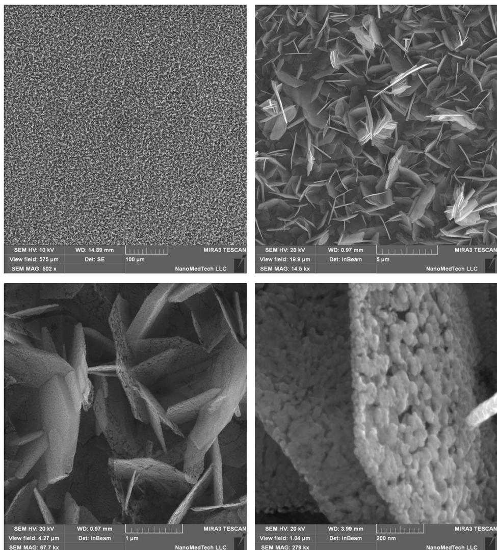
Figure S4. SEM images of electrodeposited and annealed FTO/ZnO film.
