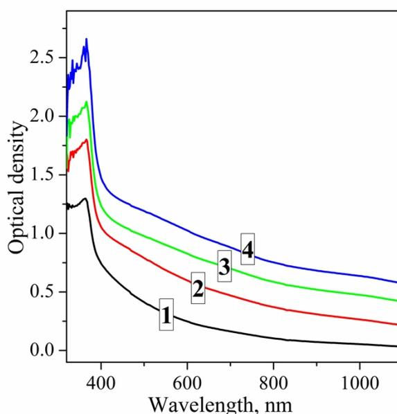
Fig. S10. Absorption spectra of ZnO films obtained at different electrodeposition duration – 2 min (curve 1), 4 min (2), 6 min (3), and 8 min (4). FTO spectrum is subtracted from curves 1–4.
