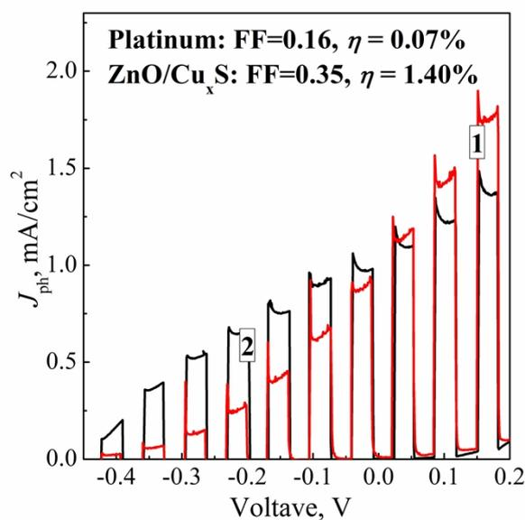
Figure S9. Illumination-modulated photocurrent–voltage dependences for ZnO/CdS photoanode coupled with platinum (curve 1) and ZnO/Cu<sub>x</sub>S heterostructure (curve 2). The ZnO/Cu<sub>x</sub>S film was produced by by partial sulfidation of zinc oxide followed with substitution of Zn(II) in ZnS with copper ions (see in more details in [23]).
