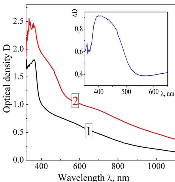
Figure S1. Extinction spectra of ZnO (curve 1) and ZnO/CdS (curve 2) films. Insert: differential CdS absorption spectrum obtained by subtracting curve 1 from curve 2.
