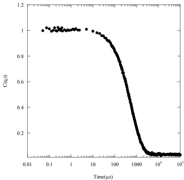
*Representative autocorrelation function  $C(q,t)$  at scattering angle of 90°.*
