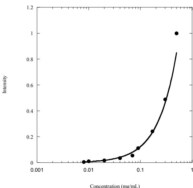
*Static light scattering variation of the graft-copolymer aqueous solutions with the concentration.*
