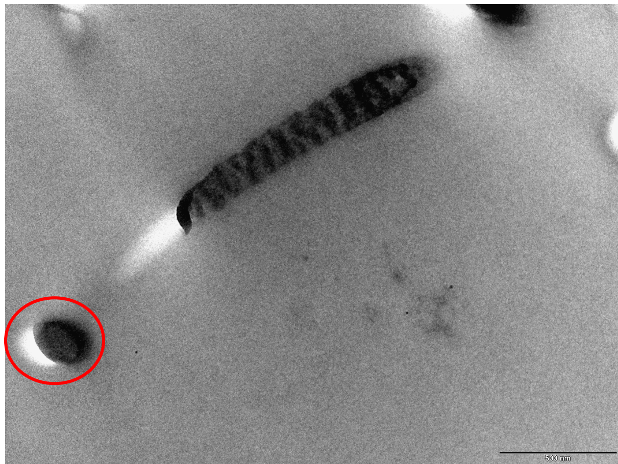
Figure S5: TEM image of electrospun PI- b -PDMAEMA/PUMVS nanocomposite fibers including perpendicular fiber axis cut.
