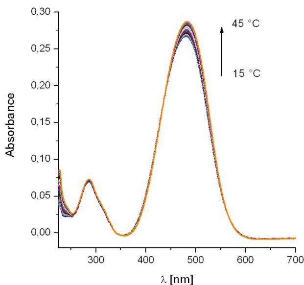
**Figure S1.** UV-vis spectra at different temperatures to demonstrate the temperature dependence of **1a**, DR1 in ethanol ( $2.4 \cdot 10^{-4} \text{ mol L}^{-1}$ ).
