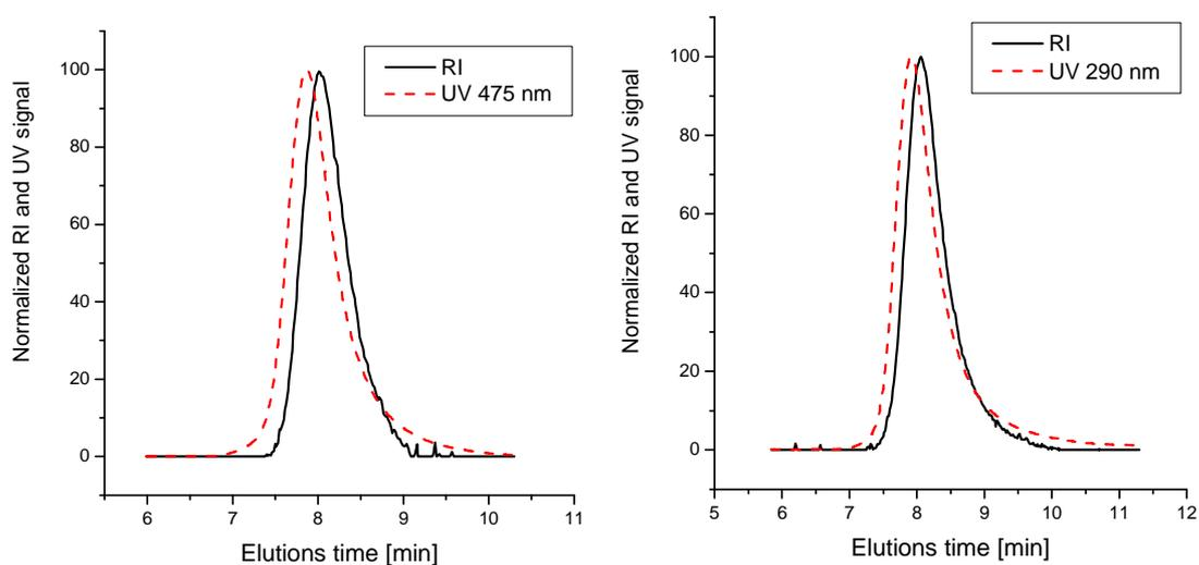
**Figure S2.** SEC traces of copolymers **5a** (left) and **5b** (right). The  $M_n$  and PDI values were determined from the RI traces with PMMA standards
