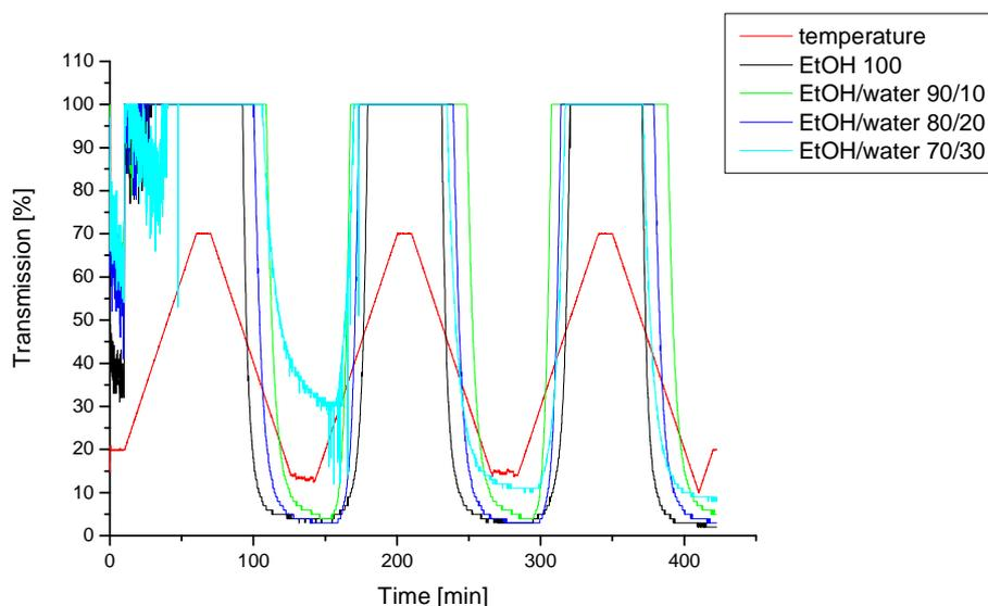
**Figure S3.** Cloud point measurements for the identification of the UCST behavior of copolymer **5a** ( $1.0 \text{ mg mL}^{-1}$ ).
