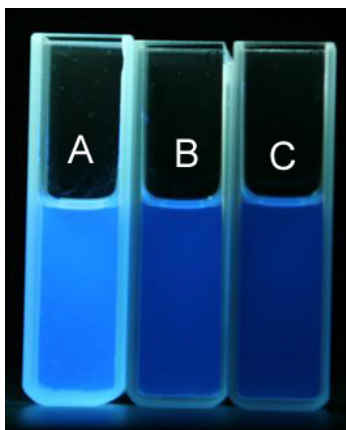
Fig S3. The illumination photograph of PDMAEMA- b -PS nanoparticles in CHCl 3 with different concentrations under a mixture of 254 nm and 365 nm irradiation (A: 0.005g/mL, B: 0.001g/mL, C: 0.0002g/mL).
