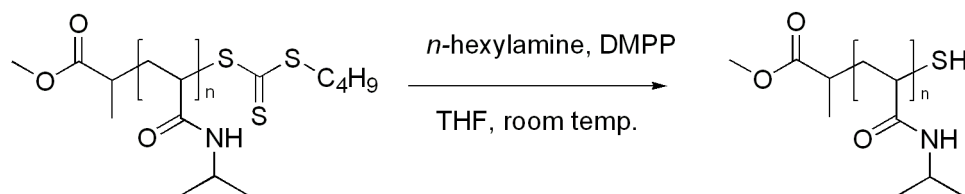
Figure SS4: Aminolysis of PNIPAM-CTA to PNIPAM-SH in the presence of DMPP.
