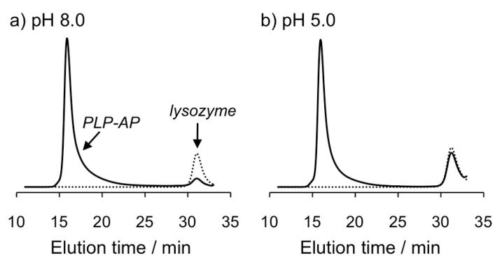
**Fig. S6.** HPLC elution profiles of lysozyme (0.15 mM, as a concentration of lysine residues in lysozyme) in the presence (solid line) or absence (dashed line) of PLPP (0.2 mM, as a molar concentration of pullulan-conjugated PLPP) at pH 8.0 (a) or pH 5.0 (b).
