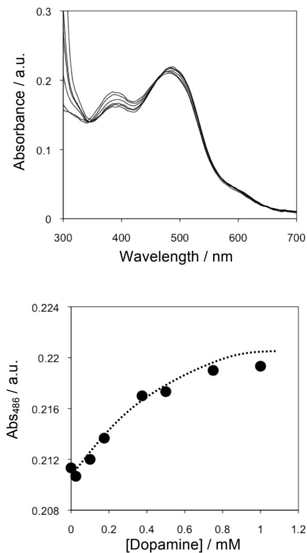
**Fig. S4.** a) Change in the UV spectra of PLPP (0.2 mM, as a molar concentration of pullulan-conjugated PLP) after the addition of dopamine in 100 mM HEPES buffer (pH 8.0) containing 100 mM NaCl and 50 mM Na<sub>2</sub>S<sub>2</sub>O<sub>3</sub> at 25°C. b) Changes in the absorbance of PLPP at 486 nm following dopamine titration.
