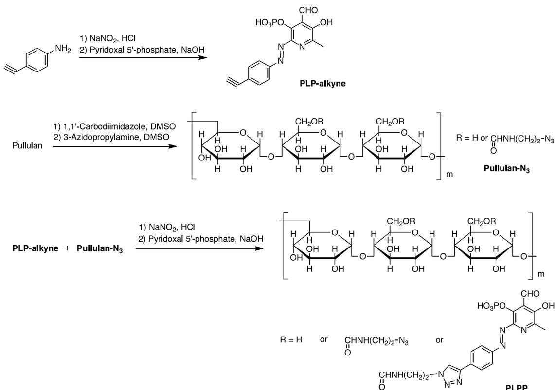
**Scheme S1.** Synthesis of pyridoxal 5'-phosphate-bearing polysaccharides.
