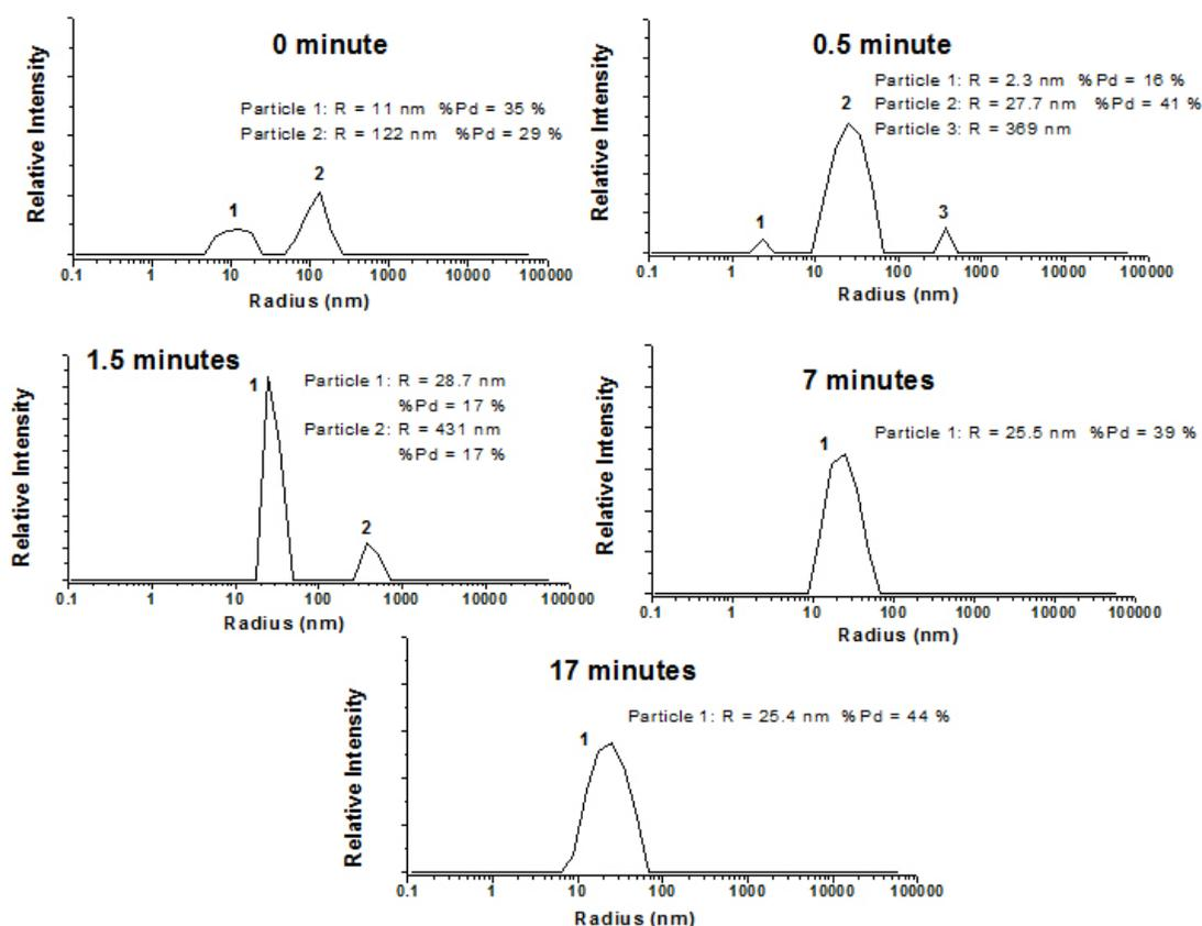
**Figure S3.** DLS monitoring of UV irradiated cross-linking of the micelle in  $\text{CH}_2\text{Cl}_2$ .
