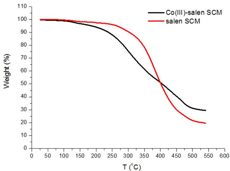
**Figure S2.** Thermograms of the SCMs **i** with salen ligand functionalized core (red line) and SCMs **i** with Co(III)-salen complex functionalized core (black line).
