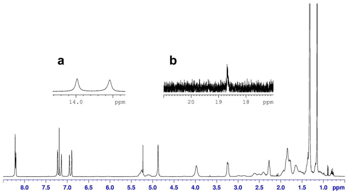
**Figure 1S.** <sup>1</sup>H NMR monitoring of the polymerization of monomer **1** ( $[M]/[I] = 40/1$ ). **Poly140** was synthesized in 1.5 hour without losing the initiated carbene signal (18.64 ppm). Inset **a**: Ar-OH signals; inset **b**: carbene signal.
