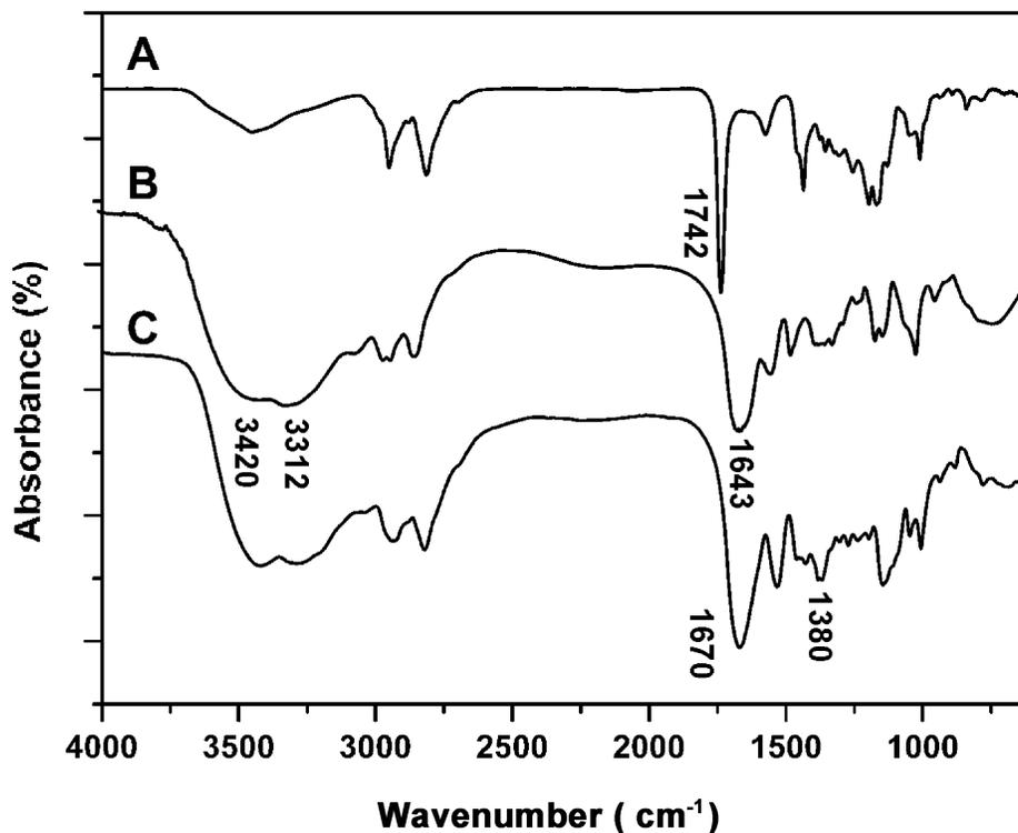
**Fig. S1** FTIR spectra of (A) AEP-ester; (B) AEP-NHNH<sub>2</sub>; and (C) HPAH.
