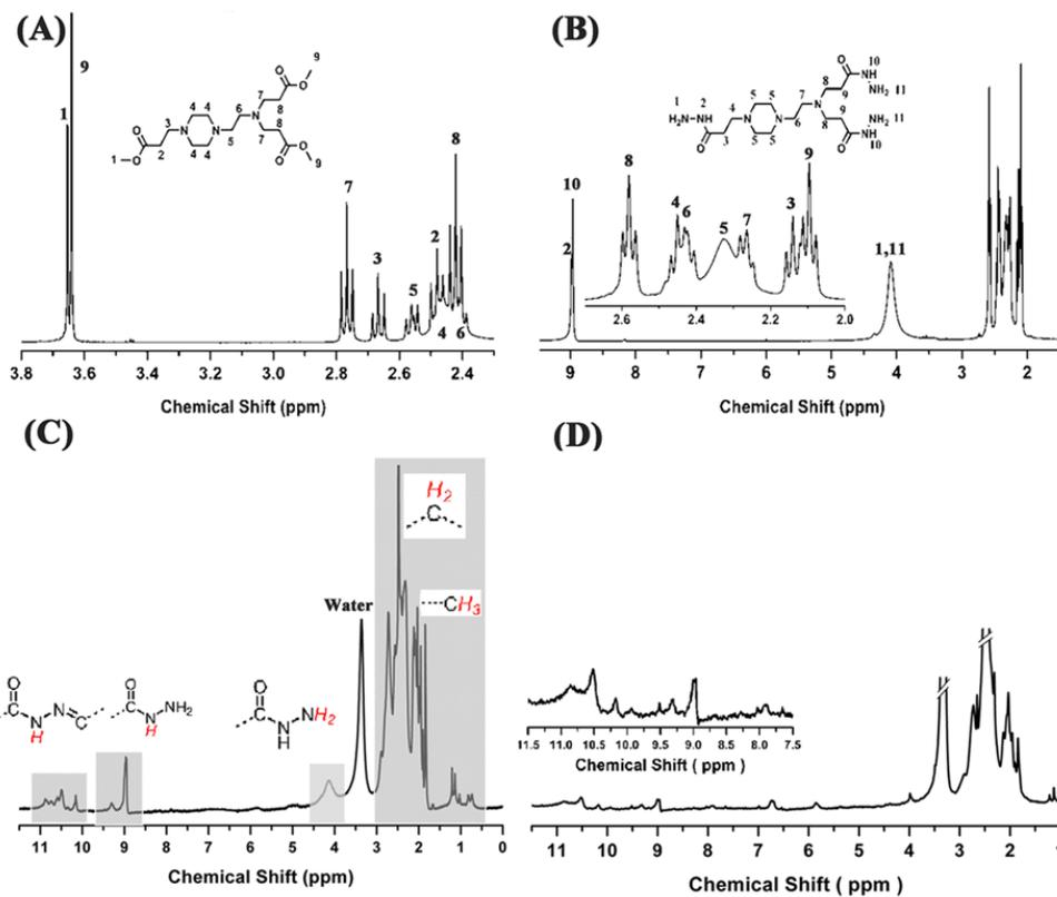
**Fig. S2** <sup>1</sup>H NMR spectra of: (A) AEP-ester in CDCl<sub>3</sub>; (B) AEP-NHNH<sub>2</sub> in DMSO-d<sub>6</sub>; (C) HPAH in DMSO-d<sub>6</sub>; and (D) HPAH-DOX in and DMSO-d<sub>6</sub> (400 MHz, 298 K).
