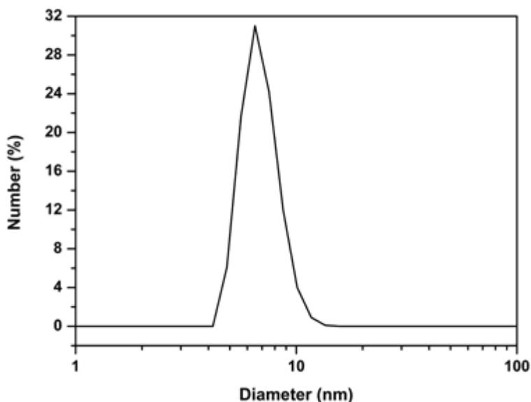
**Fig. S5** Dynamic light scattering (DLS) measurements of the hydrodynamic diameter of HPAH.
