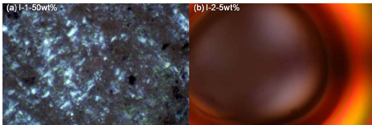
**Figure S6.** Photomicrographs of (a) **I-1-50 wt %**, and (b) **I-2-5 wt %** taken under crossed polarizers at room temperature exhibiting lyotropic solutions (magnification 400×).
