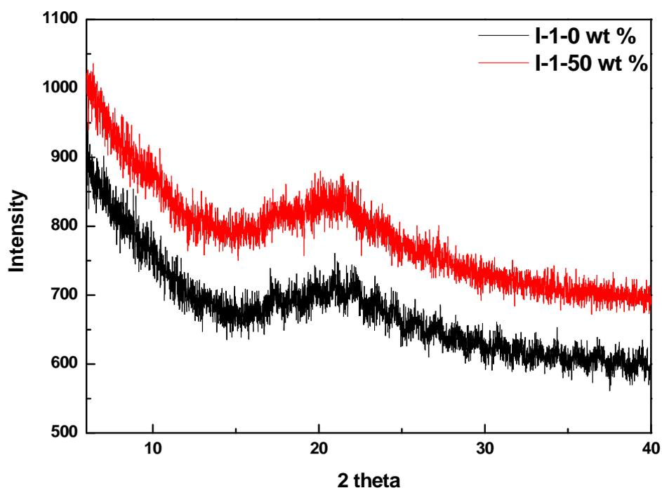
**Figure S7.** XRD plots of **I-1-0 wt %** and (b) **I-1-50 wt %** in 30 wt % DMSO taken at room temperature.
