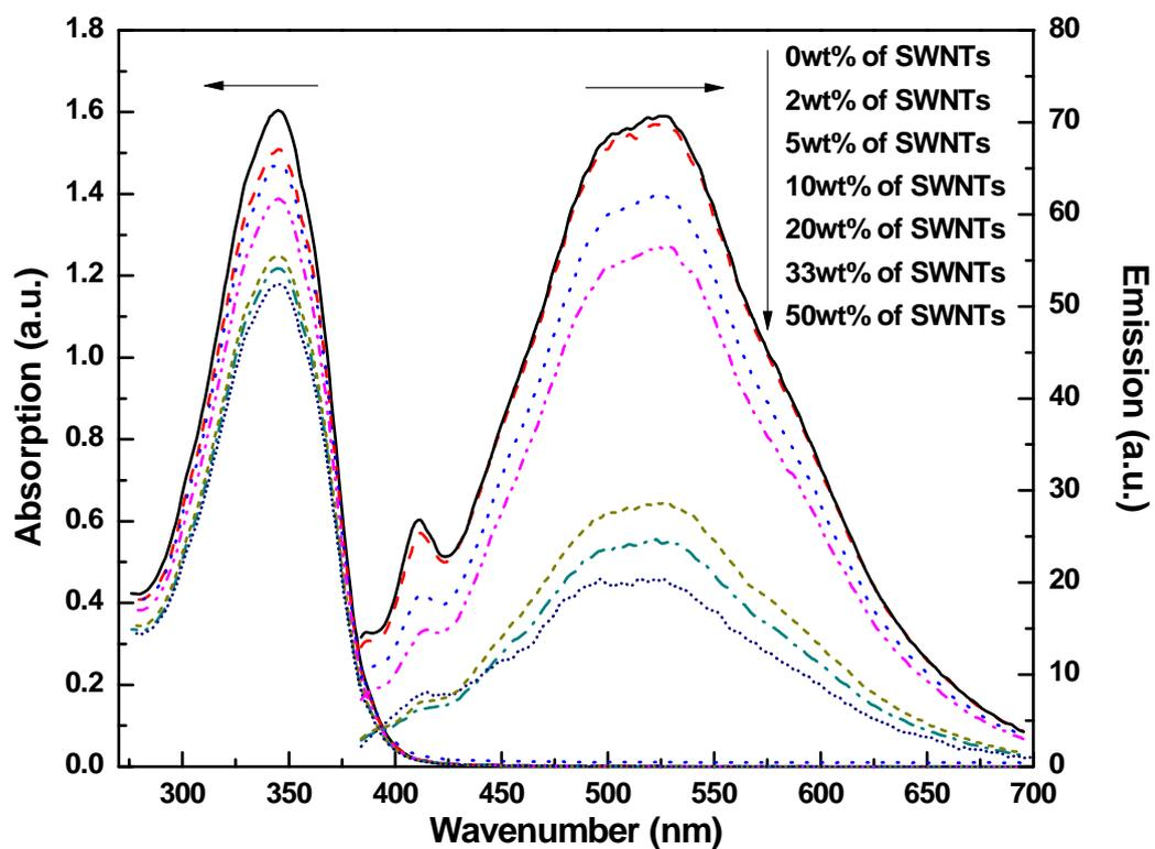
**Figure S1.** UV-Vis absorption spectra of I-2/SWNT composites in DMSO (left arrow) and emission spectra of I-2/SWNT composites at excitation wavelength of 364 nm in DMSO (right arrow).
