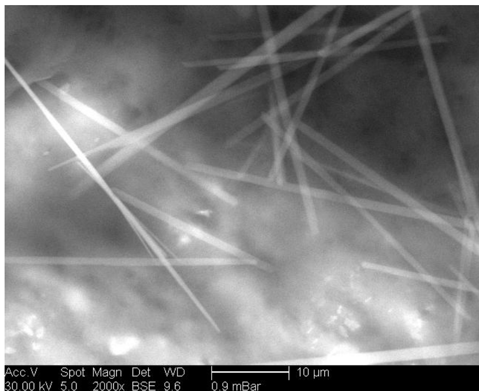
Figure S13. SEM image of fibers resulting from the self-assembly of conjugate 5 in water at lower magnification.
