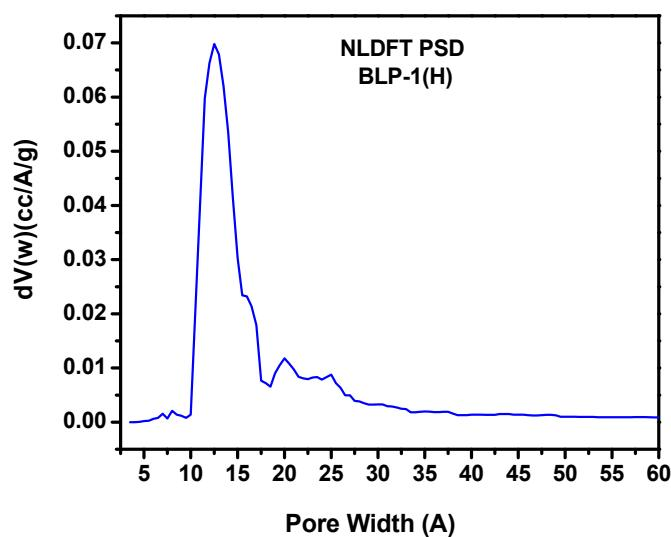
**Figure S19:** NLDFT Pore Size Distribution for BLP-12(H)
