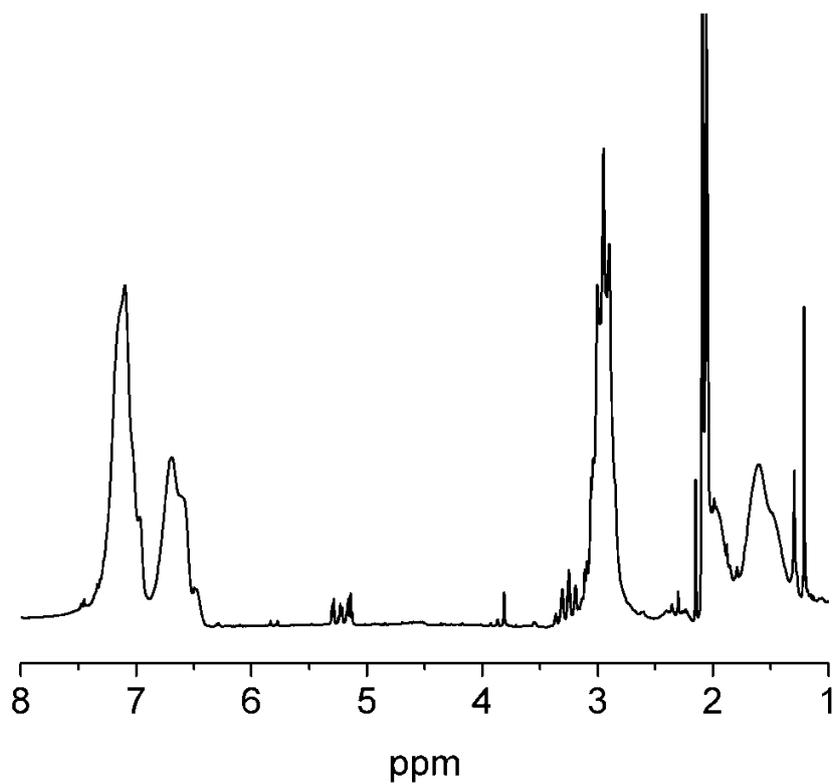
**Figure S1.**  $^1\text{H-NMR}$  spectrum of the PVDF-*b*-PS copolymer obtained from the reaction of azide-terminated PVDF with  $M_n = 2200 \text{ g}\cdot\text{mol}^{-1}$  and alkyne-terminated PS with  $M_n = 3500 \text{ g}\cdot\text{mol}^{-1}$ .
