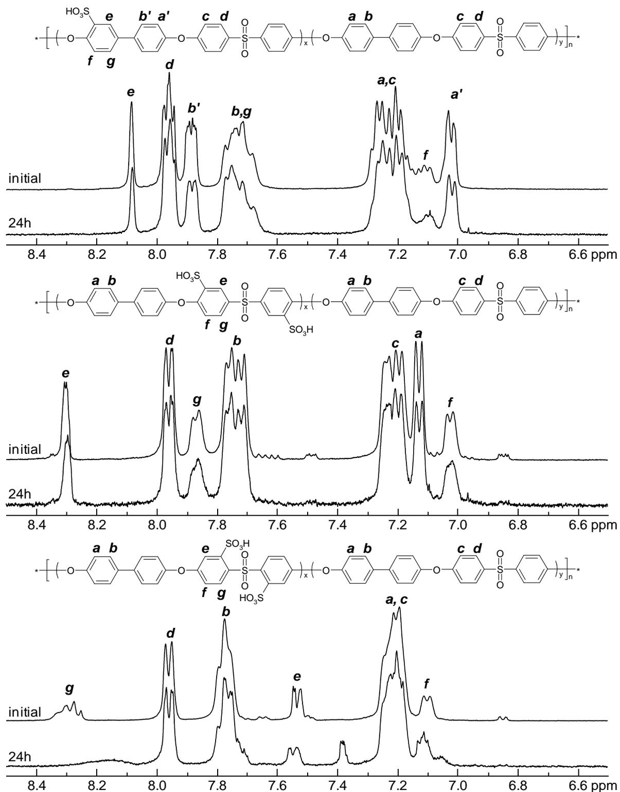
**Figure S4.**  $^1\text{H}$  NMR spectra of (a) the *oeSPAESm*, (b) the *msSPAESm*, and (c) the *osSPAESm* copolymers before and after a hydrolysis test where the membranes were treated in neutral deionized water at 200 °C for 24 h in a sealed vessel.
