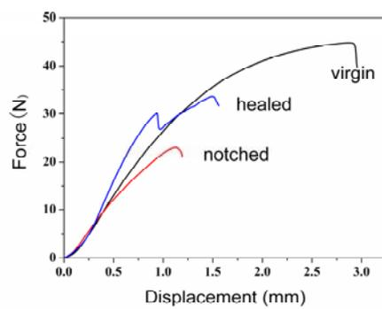
Fig. S7 Force vs displacement curves for the virgin, damaged and healed state of PPDO-PTMEG co-network.
