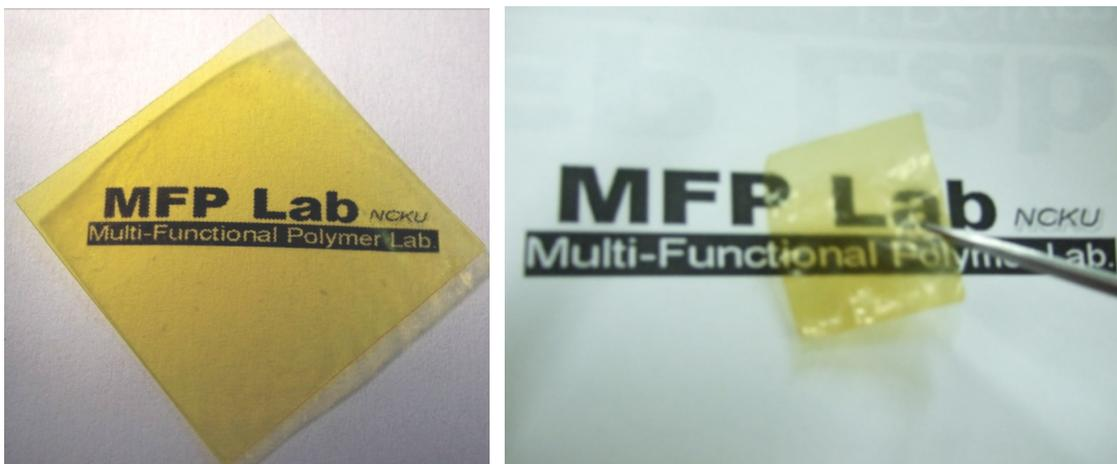
**Fig. S5** The membrane  $M(VI)_6$  before (left) and after (right) the oxidative stability test.
