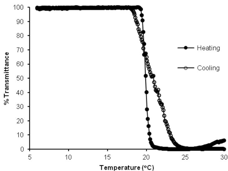
**Figure S12.** Percentage transmittance *versus* temperature plot for poly(6<sub>13</sub>-co-5<sub>4</sub>-graft-NiPAm<sub>40</sub>) at 1 mg mL<sup>-1</sup> in nanopure water (heating/cooling rate 1 °C min<sup>-1</sup>).
