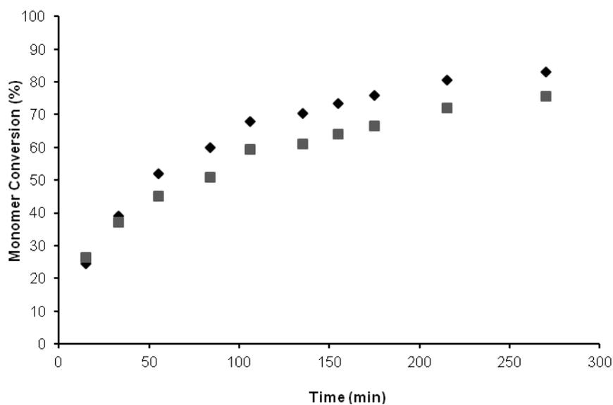
**Figure S4.** Monomer conversion *versus* time for monomer **5** (diamonds) and **6** (squares) during a 1:1 copolymerization (**5**:**6**) (monomer conversion determined by  $^1\text{H}$  NMR spectroscopy).
