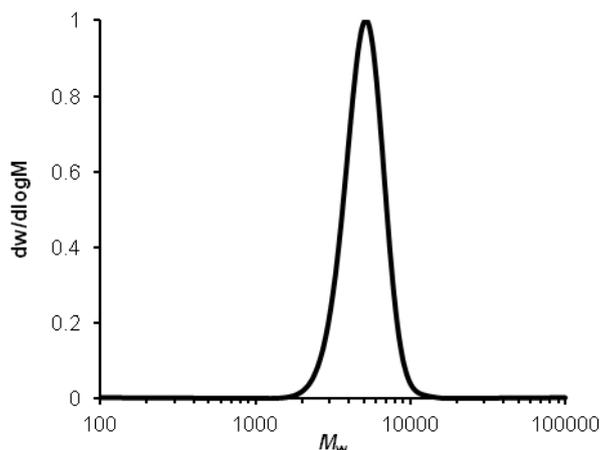
**Figure S3.** SEC trace of poly(**5**) ( $M_n = 4.8$  kDa,  $D = 1.09$ ) ( $[M]_0/[I]_0 = 20$ ,  $[5] = 0.25$  M, using 5 mol% DBU and 4-methoxybenzyl alcohol as an initiator).
