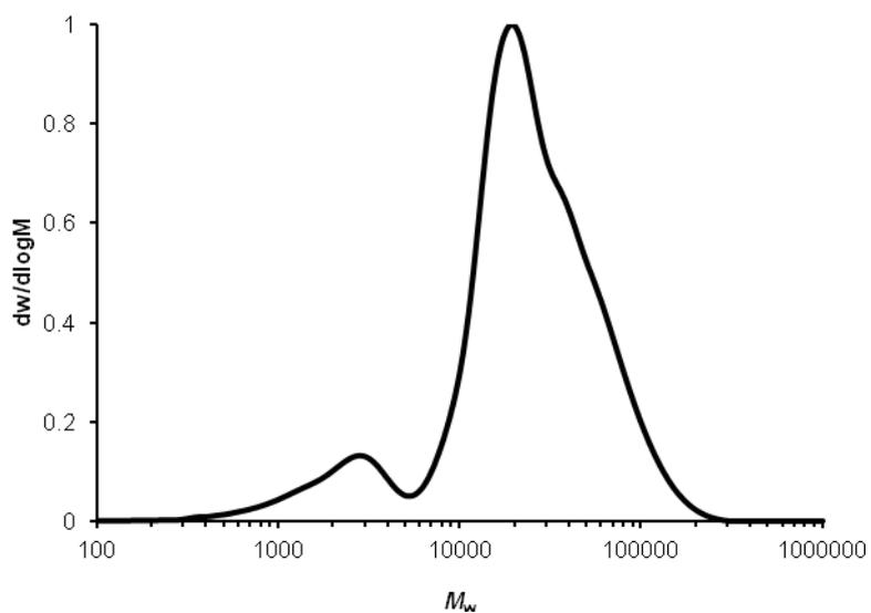
**Figure S6.** SEC trace of poly(**6-co-5-graft-styrene**) ( $M_n = 9.6$  kDa,  $\mathcal{D} = 3.28$ ) (polymerization performed in  $\text{CHCl}_3$  at  $65^\circ\text{C}$ ,  $[\text{CTA}]:[\text{AIBN}]:[\text{styrene}] = 1:0.1:50$ ,  $[\text{starting polymer}] = 0.01$  M).
