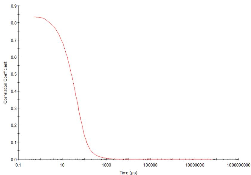
**Figure S10.** Correlation function for poly( $6_{13}\text{-co-}5_4\text{-graft-NiPAm}_{40}$ ) micelles at  $1 \text{ mg mL}^{-1}$  in nanopure water.
