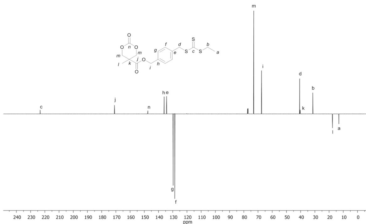
**Figure S1.**  $^{13}\text{C}$  NMR spectrum of RAFT CTA functional carbonate monomer **5** in  $\text{CDCl}_3$  (100 MHz, 298 K).
