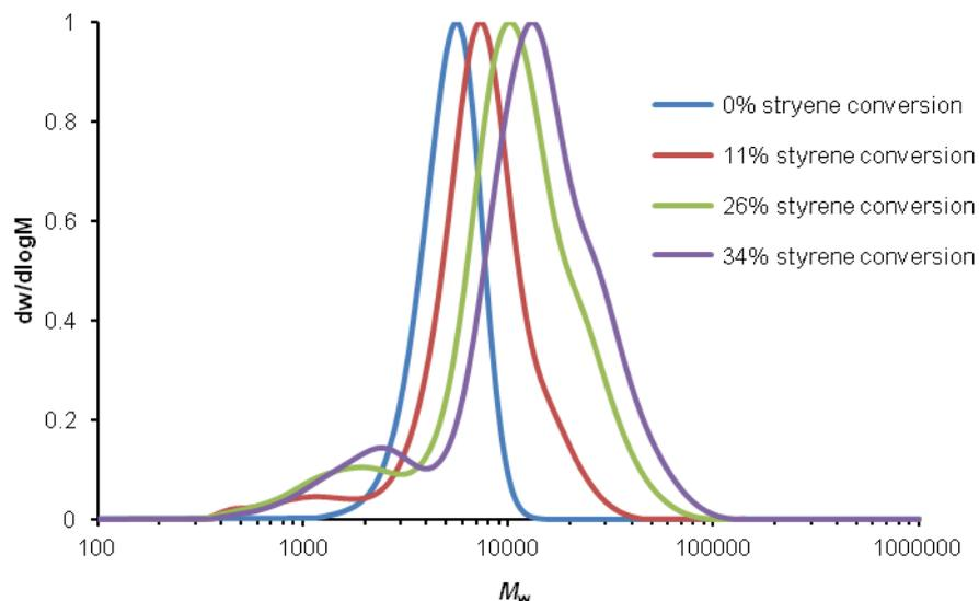
**Figure S7.** Evolution of SEC traces during preparation of poly(6-co-5-graft-styrene) (polymerization performed in CHCl<sub>3</sub> at 65 °C, [CTA]:[AIBN]:[styrene] = 1:0.1:50, [starting polymer] = 0.003 M).
