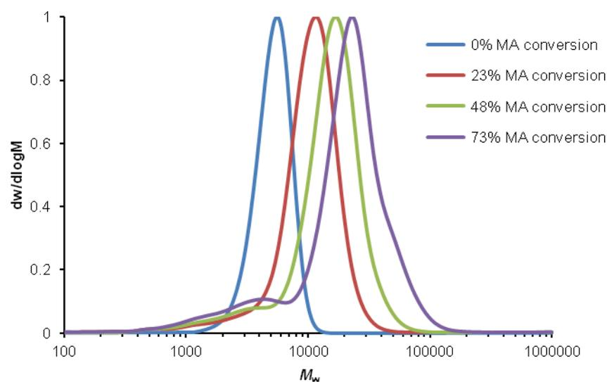
**Figure S8.** Evolution of SEC traces during preparation of poly(6-co-5-graft-MA) (polymerization performed in CHCl<sub>3</sub> at 65 °C, [CTA]:[AIBN]:[MA] = 1:0.1:50, [starting polymer] = 0.003 M).
