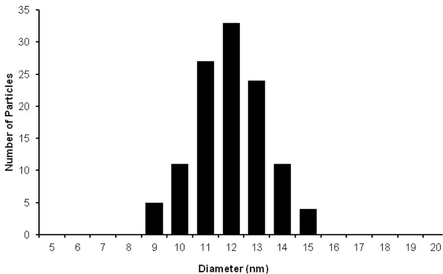
**Figure S11.** TEM size distribution histogram for poly(6<sub>13</sub>-co-5<sub>4</sub>-graft-NiPAm<sub>40</sub>) micelles.
