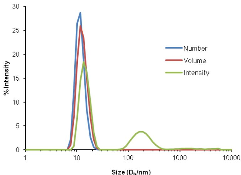
**Figure S13.** DLS data for micelles prepared from poly(**6**<sub>13</sub>-*co*-**5**<sub>4</sub>-*graft*-NiPAM<sub>40</sub>) formed after a heating/cooling cycle.
