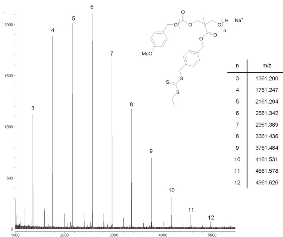
**Figure S2.** MALDI-ToF MS of RAFT CTA functionalized polycarbonate (reflectron mode).
