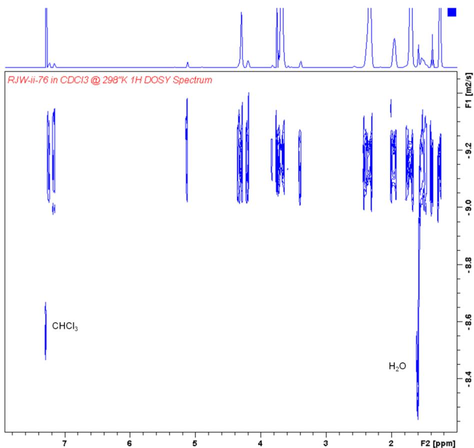
**Figure S9.**  $^1\text{H}$  DOSY spectrum of poly( $6_{13}\text{-co-}5_7\text{-graft-MA}_{39}$ ) in  $\text{CDCl}_3$  (500 MHz, 298 K).
