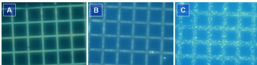
**Fig. S16** Negative-tone photoresist patterns generated by photo-crosslinking of thin films of (A) **1**, (B) **2** and (C) **3**. The photographs were taken under UV illumination from a hand-held UV lamp.
