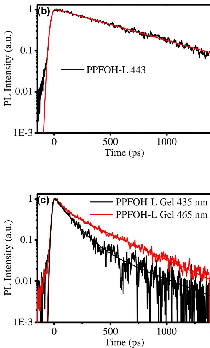
**Figure S9.** PL decays of PPFOH-L in solution and gel. (a) PPFOH-L in THF solution. (b) PPFOH-L in toluene solution. (c) PPFOH-L/toluene gel.
