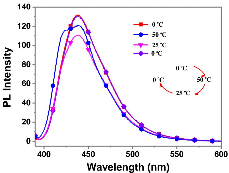
**Figure S5.** Emission spectra of PPFOH-L in toluene at 0, 25 and 50 °C. (Excited at 390 nm)
