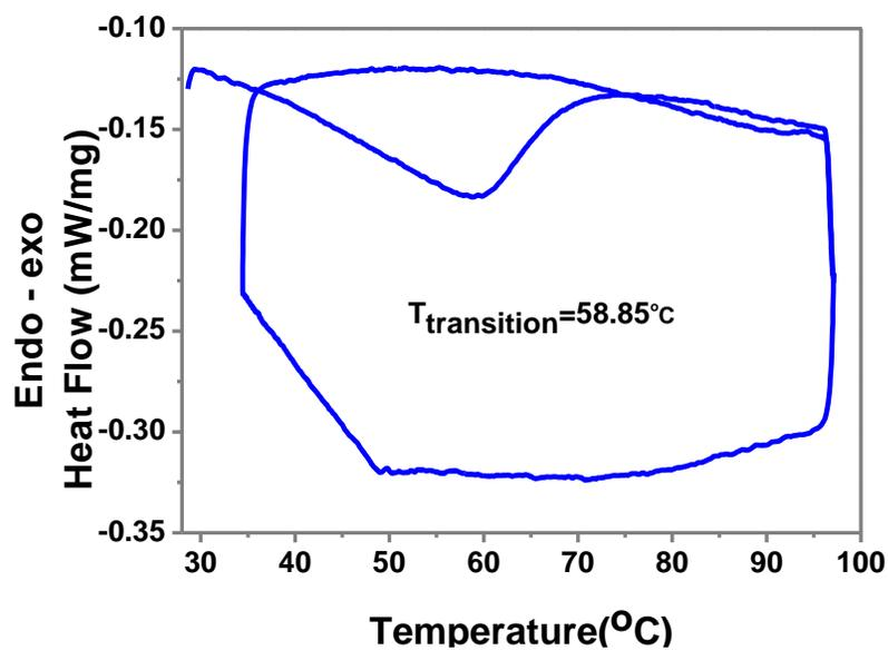
**Figure S3.** Cooling-heating cycles for DSC measurement of PPFOH-L/toluene gel from 30 to 100 °C .
