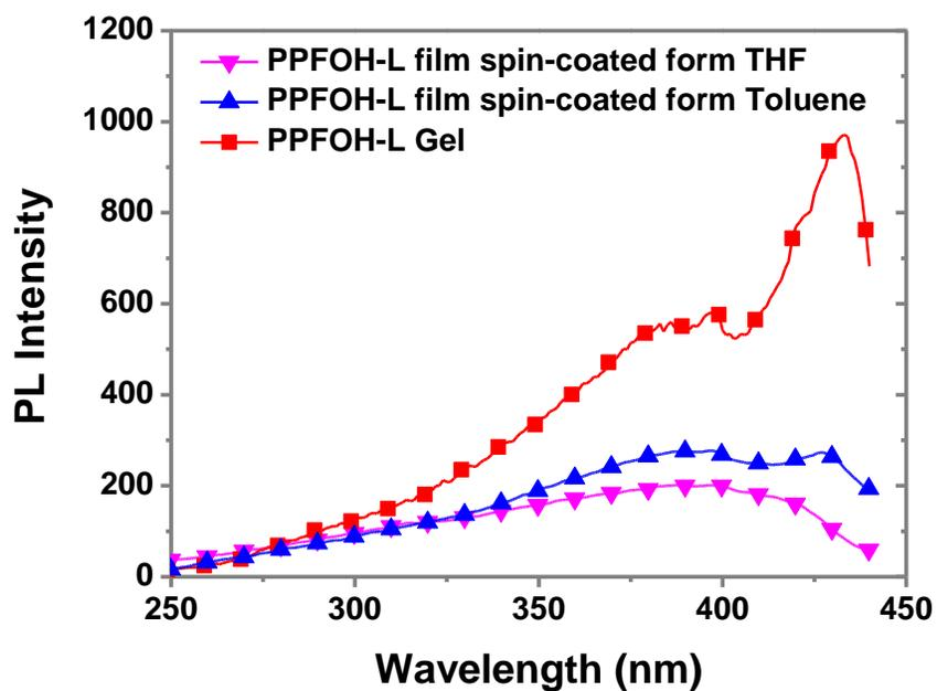
**Figure S8.** PLE spectra of PPFOH-L/toluene gel and films spin-coated from THF and toluene solution. (Emission at 460 nm)
