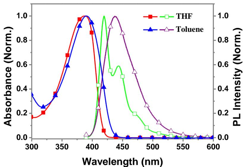
**Figure S7.** The UV-*vis* and PL spectra of PPFOH-L in THF and toluene. (Excited at 390 nm)
