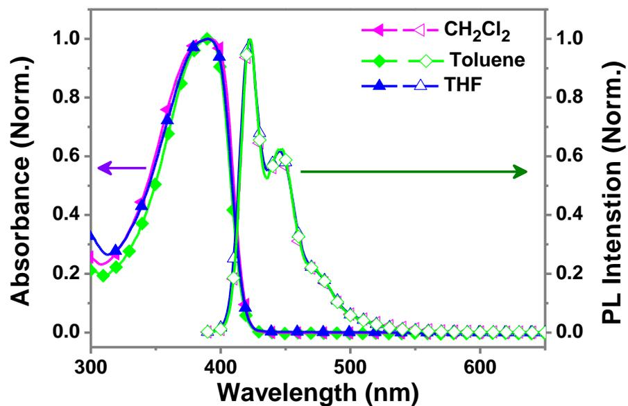
**Figure S4.** Absorbance and PL spectra of PPFO8 in various solution (concentration: 0.01 mg/ml). (Excited at 390 nm)
