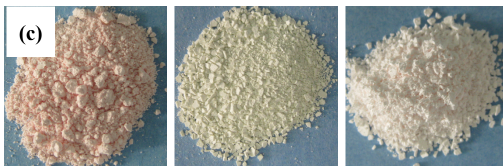
Figure S11. Original PS: [\text{St}]_0/[\text{CPDB}]_0/[\text{AIBN}]_0 = 500/5/1 , time = 71 h, Conversion = 56.7 %, temperature = 60 °C, St = 2.0 mL, toluene = 1.0 mL; Treated conditions: PS treated by Cu(0) powder/PMDETA: [\text{PS}]_0/[\text{Cu}(0) \text{ powder}]_0/[\text{PMDETA}]_0/[\text{TEMPO}]_0 = 0.39/1/1/1 , time = 72 h, PS = 0.2334 g, DMF = 5 mL, 25 °C; PS treated by Fe(0) powder: [\text{PS}]_0/[\text{Fe}(0) \text{ powder}]_0/[\text{TEMPO}]_0 = 0.39/1/1 , time = 72 h, PS = 0.2334 g, DMF = 5.0 mL, 25 °C; (a) SEC evolutions of the original PS and treated PS. (b) Enlarged ^1\text{H} NMR spectra of the original PS and treated PS. (c) Photographs of PS before and after treatment.
