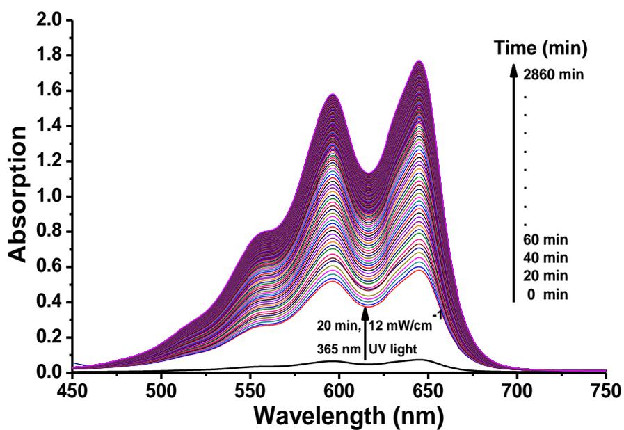
**Figure S5.** Release of the dye (solvent blue 35) from microcapsules in hexane solution monitored by changes in the dye absorbance at 597 and 645 nm. Figure shows the absorption of hexane solution before UV-irradiation and after 20 min UV-irradiation which was then followed for the next 48 hours.
