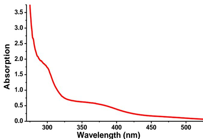
**Figure S4.** UV spectrum of the NVOC-based diisocyanate oligomer in d-DMSO ( $10 \text{ mg mL}^{-1}$ ) after 4 hours of UV irradiation.
