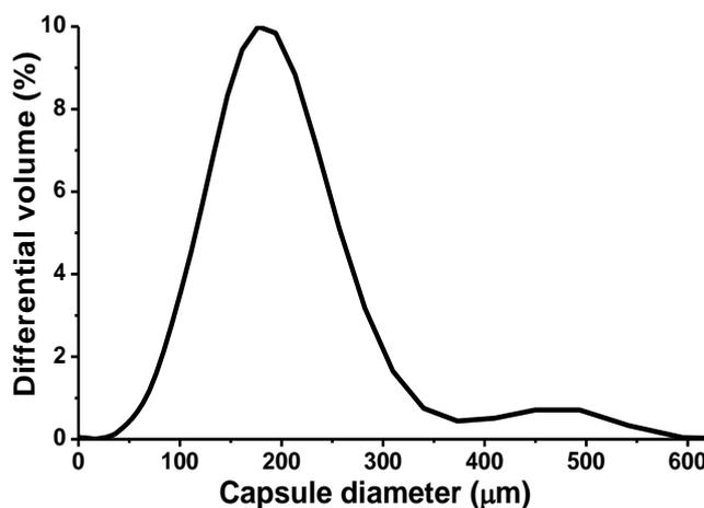
**Figure S1.** Differential volume distribution curve of particle diameter of microcapsules. ( $d_{10}$ : 94  $\mu\text{m}$ ,  $d_{50}$ : 175  $\mu\text{m}$ ,  $d_{90}$ : 273  $\mu\text{m}$ )
