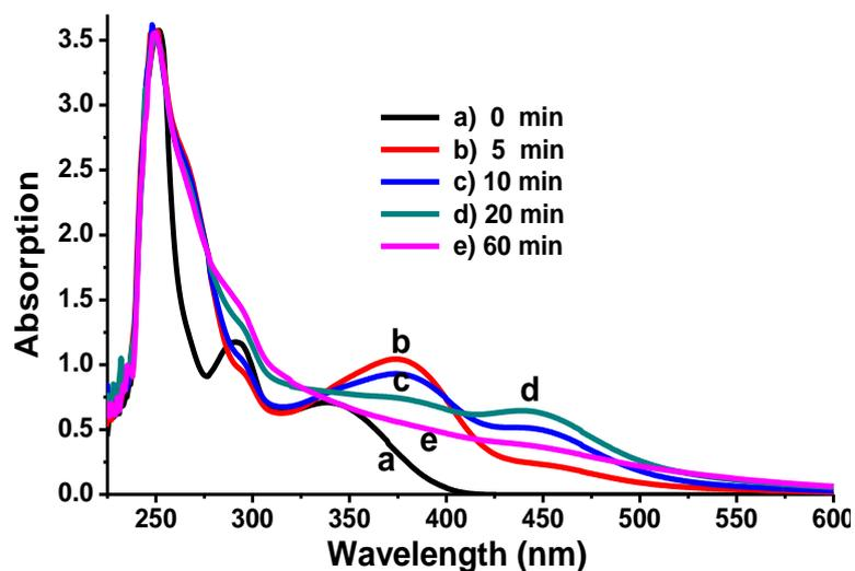
**Figure S2.** A) UV spectra of the NVOC-based diisocyanate oligomer in DMSO ( $1 \text{ mg mL}^{-1}$ ) after different UV irradiation times (0-60 min).
