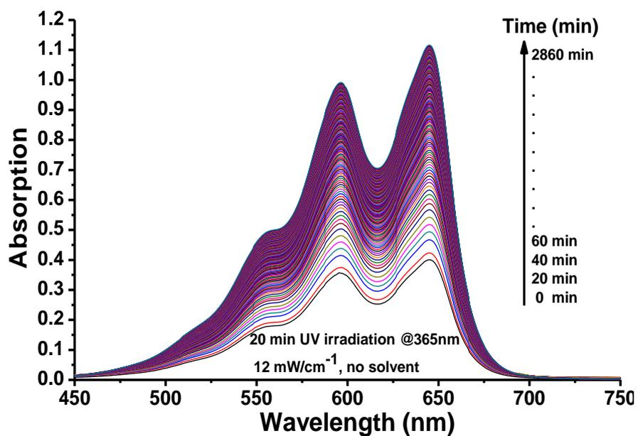
**Figure S6.** Release of the dye (solvent blue 35) from microcapsules in hexane solution monitored by changes in the dye absorbance at 597 and 645 nm after 20 min UV-irradiation on the solid microcapsules. After UV-irradiation on solid microcapsules, microcapsules were dispersed in hexane and the absorption of hexane solution was monitored for 48 hours.
