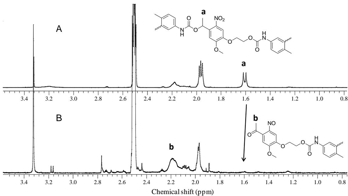
**Figure S3.**  $^1\text{H}$  NMR spectrum of NVOC-based diisocyanate oligomer in d-DMSO ( $10 \text{ mg mL}^{-1}$ ) A) before UV-irradiation, B) after 4 hours of UV-irradiation.
