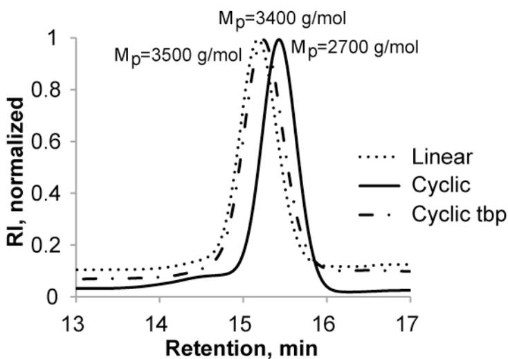
**Figure S6.** SEC profiles of *l*-PS (**6**), *c*-PS (**7a**) and *c*-PS after the reaction with tri-*n*-butylphosphine.
