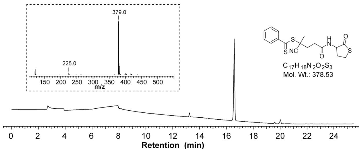
**Figure S3.** LC-MS analysis of TLa-CTA (Scheme 1, 5). Insert: ESI-MS spectrum (positive mode) of the main peak.
