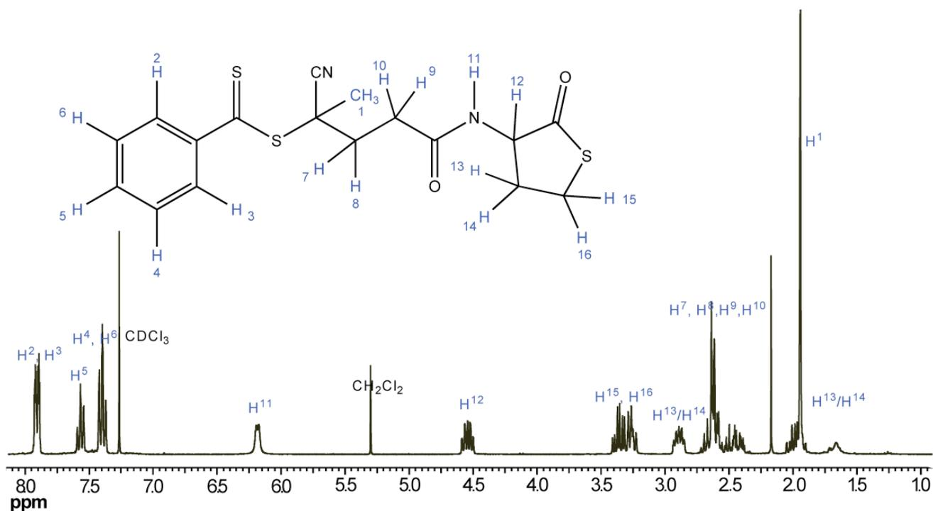
**Figure S2.**  $^1\text{H-NMR}$  (300 MHz,  $\text{CDCl}_3$ ) analysis of purified **TLa-CTA** (Scheme 1, **5**) with corresponding signal assignment.
