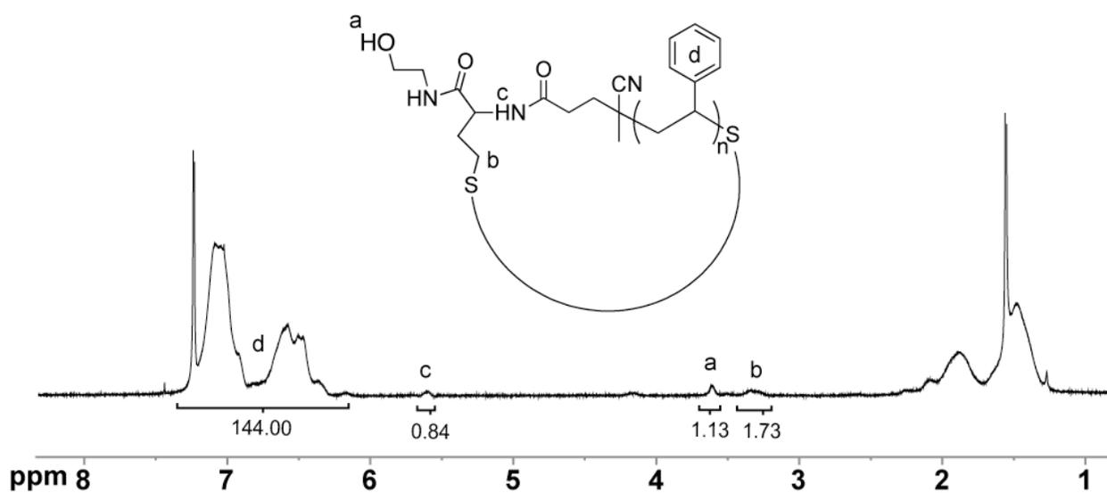
**Figure S7.** <sup>1</sup>H-NMR (500 MHz, CDCl<sub>3</sub>) spectra of cyclic PS (*c*-PS, **7b**) with corresponding signal assignment.
