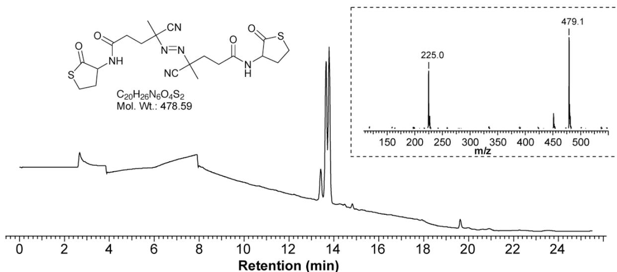
**Figure S1.** LC-MS analysis of purified azo-compound **3** (Scheme 1). Insert: ESI-MS spectrum (positive mode) of the main peaks.
