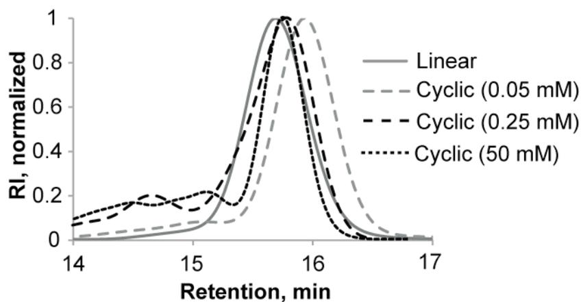
**Figure S5.** SEC profiles of: *l*-PS (**6**), *c*-PS (**7a**) prepared at 0.05 mM concentration and cyclization attempts at higher polymer concentrations (0.25 mM and 50 mM) with high MW tailing (lower retention), indicating intermolecular disulfide formation.
