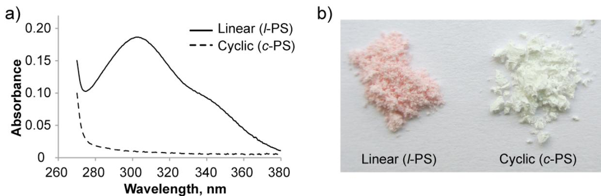
**Figure S4.** a) UV-vis spectrum of *l*-PS showing absorbance at ca. 303 nm (presence of dithiobenzoate group) and *c*-PS (no absorbance after removing dithiobenzoate group); b) visual inspection of *l*-PS (light-pink) and *c*-PS (white) indicating successful removal of dithiobenzoate group evidenced in a clear color change.
