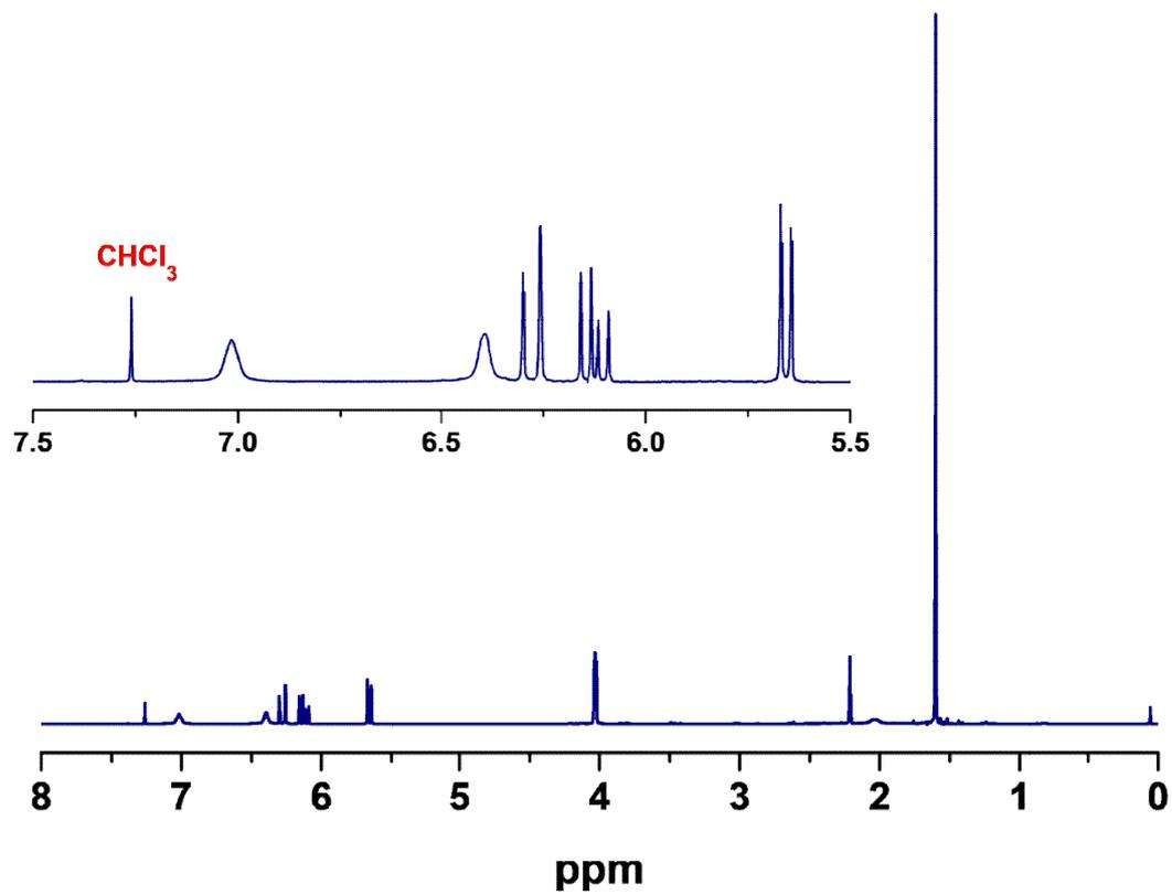
Figure S2. NMR analysis of the ring opened product upon treatment of VDMA with propargyl amine.
