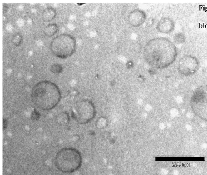
**Figure S6:** TEM image of polymersomes formed from block copolymer **6**. The black bar represents 200 nm.
