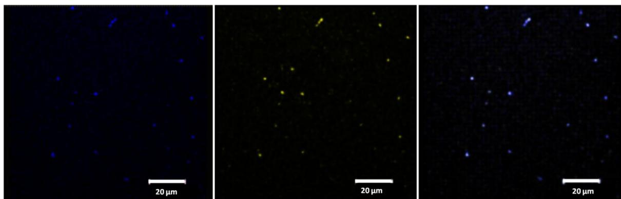
**Figure S7:** Left, selective detection of rhodamine emission after 24 hours of catalyzed exchange. Middle, selective detection of fluorescein emission and right, the overlay of both images showing the presence of both fluorophores at the same polymeric vesicles after 24 hours of equilibration.
