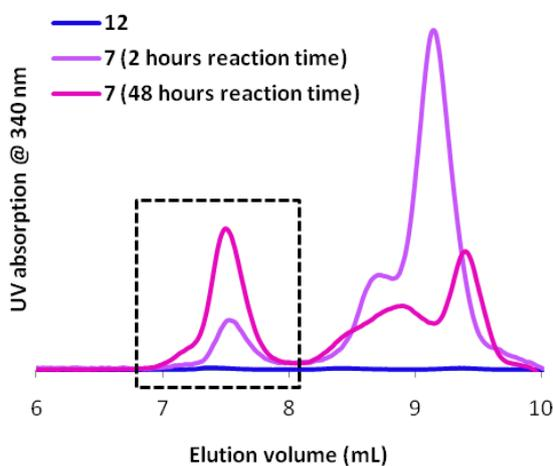
**Figure S4:** SEC (THF) analysis of block copolymer **12**, which does not absorb at 340 nm before the addition of rhodamine B isothiocyanate. After 2 hours the labeled polymer (top ~7.5 mL) does absorb at 340 nm, which increases over the next 46 hours. The dashed box indicates the volume, containing product **7**, that was collected by preparative SEC in THF.
