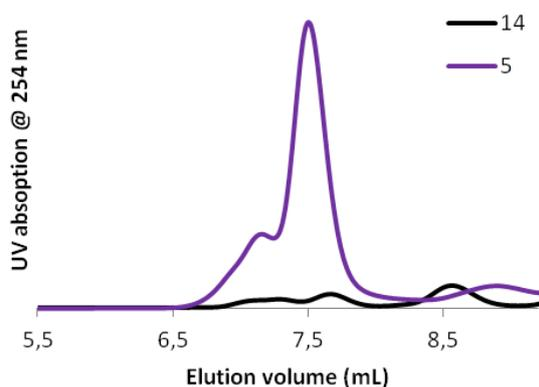
**Figure S3:** Using equal polymer concentrations for SEC (THF) analysis. UV absorption at 254 nm can be detected for polymer **5**, due to the presence of triazoles and a maleimide, whereas only limited absorption is observed before the introduction of a maleimide (**14**).
