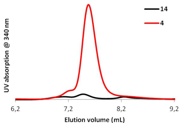
**Figure S2:** Using equal polymer concentrations for SEC (THF) analysis. UV absorption at 340 nm can be detected for polymer **4**, due to the presence of SX-1031, whereas only limited absorption is observed before the coupling (**14**).
