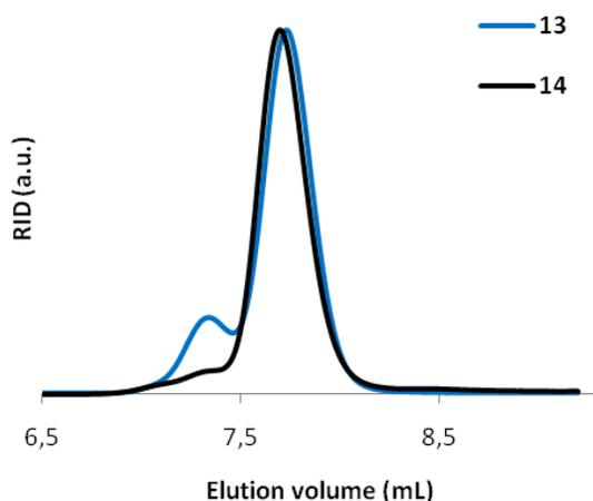
**Figure S5:** Synthesis of  $\omega$ -azido-polybutadiene-hydrazone-poly(ethylene glycol) (**14**) from polymers **10** and **13**. Due to an increase in molecular weight the GPC trace shifts to shorter elution time.
