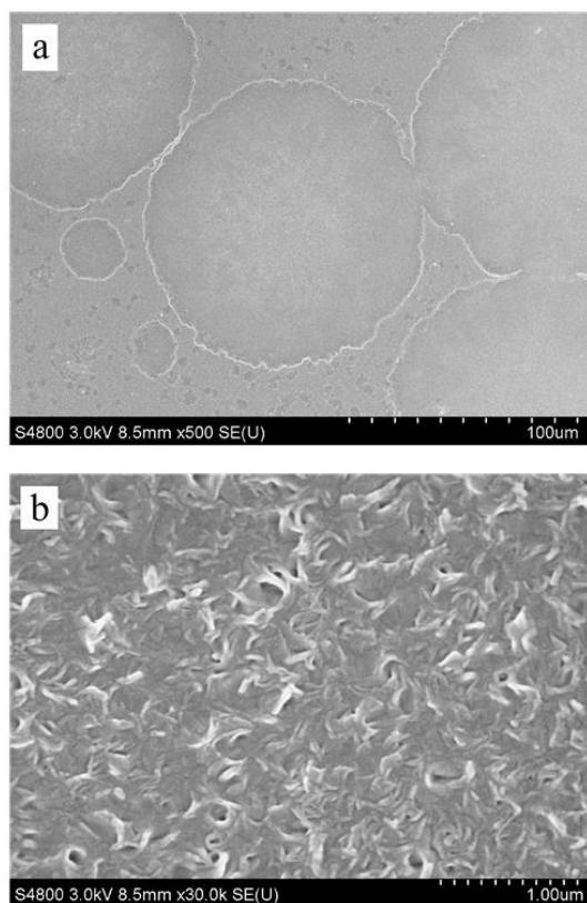
**Fig. S4** SEM images of catalyzed LT-CBT polymerized in hot stage at 190 °C for 90 min.
