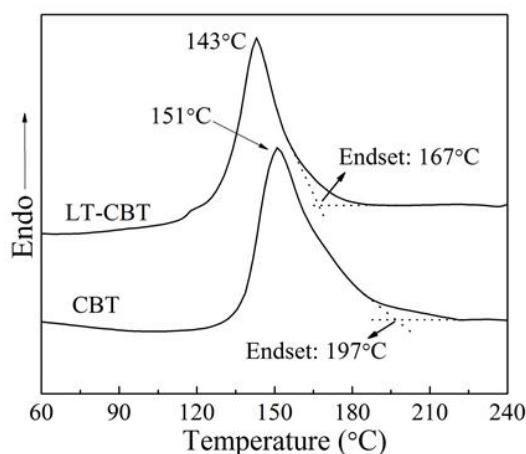
**Fig. S1** DSC thermograms of CBT and LT-CBT, heating at 100 °C/min.
