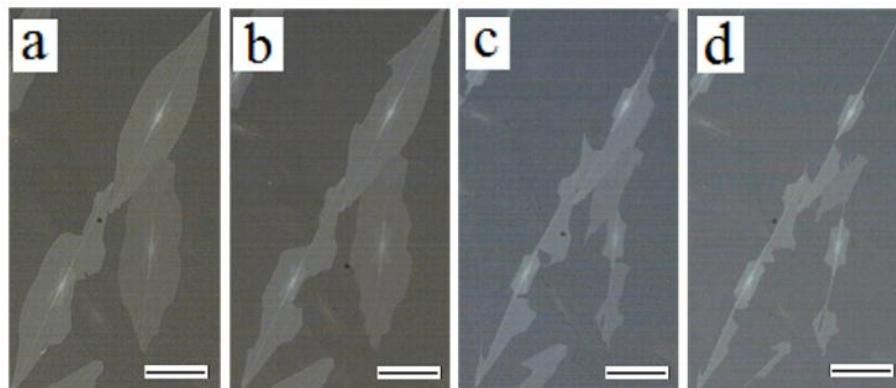
**Fig. S2** In situ POM images of un-melted CBT in catalyzed CBT at 190 °C for 30 min in hot stage and then in situ heating. (a) 190 °C; (b) 192 °C; (c) 194 °C; (d) 196 °C. Scale bars: 20μm
