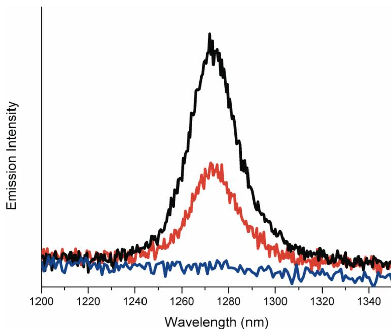
**Figure S10.** Emission spectra of singlet oxygen generated by dendritic porphyrin photosensitizer (**10**) ( $2.7 \times 10^{-6}$  M) in  $D_2O$  (black), in presence of  $^1O_2$  quencher DABCO: 1eq (red) and 0.1M (blue). Excitation at 560 nm.
