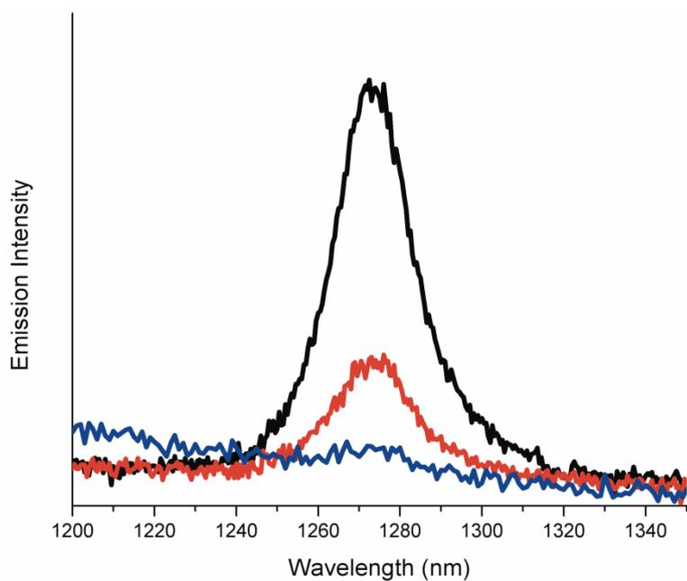
**Figure S9.** Emission spectra of singlet oxygen generated by dendritic porphyrin photosensitizer (**7**) ( $8.7 \times 10^{-6}$  M) in  $D_2O$  (black), in presence of  $^1O_2$  quencher DABCO: 1eq (red) and 0.1M (blue). Excitation at 560 nm.
