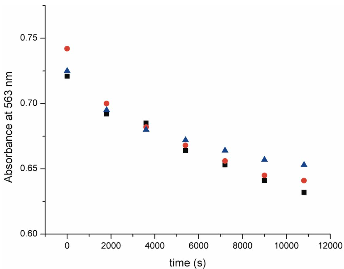
**Figure S11.** Advancement of photodegradation of (4 ■) , (7 ●) and (10▲) in air-equilibrated D<sub>2</sub>O on a long timescale ( in seconds) upon irradiation at 532 nm. (Laser power = 3.7mW)
