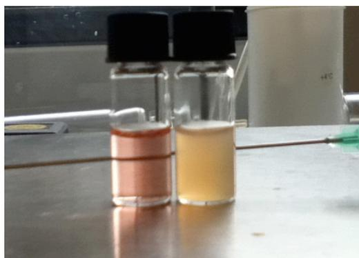
Figure S2. Photos for PPFPA (A) and PPFPA-ONB (ONB ratio, 10%) (B) after photo-crosslinking.
