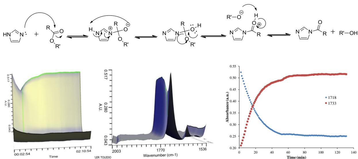
**Figure S2.** *In situ* FTIR of DEGMEMA in imidazole at 100 °C to probe possible reactions occurring during annealing of triblock copolymer films. Imidazole catalyzed the hydrolysis of DEGMEMA (1718 cm<sup>-1</sup>) into an amide bond (1733 cm<sup>-1</sup>) and di(ethylene glycol) methyl ether as evidenced in the *in situ* FTIR plots. The proposed mechanism is shown above.
