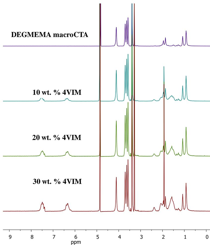
**Figure S4.** <sup>1</sup>H NMR spectroscopy of the DEGMEMMA macroCTA and the various 4VIM-containing triblock copolymers in CD<sub>3</sub>OD.
