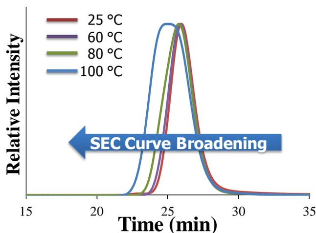
**Figure S1.** Aqueous SEC of poly(4VIM-*b*-DEGMEMA-*b*-4VIM) triblock copolymers after annealing for 24 h at various temperatures. SEC curve broadening occurred suggesting a post-polymerization reaction for extended times at elevated temperatures.
