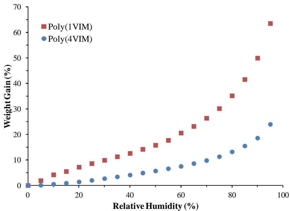
**Figure S5.** Water sorption analysis of poly(1VIM) and poly(4VIM) at various relative humidities.
