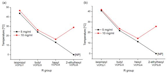
Cloud point (CP) in ethanol as a function amide moiety at 50% transmittance. (a) Cloud point upon heating and (b) Cloud point upon cooling. NP (No precipitation)
