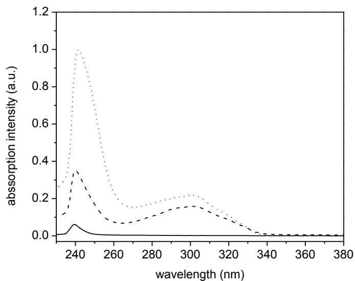
**Figure S7.** UV-Vis spectra of polymers **4** (solid line), **7** (dash line), and **10** (dot line).
