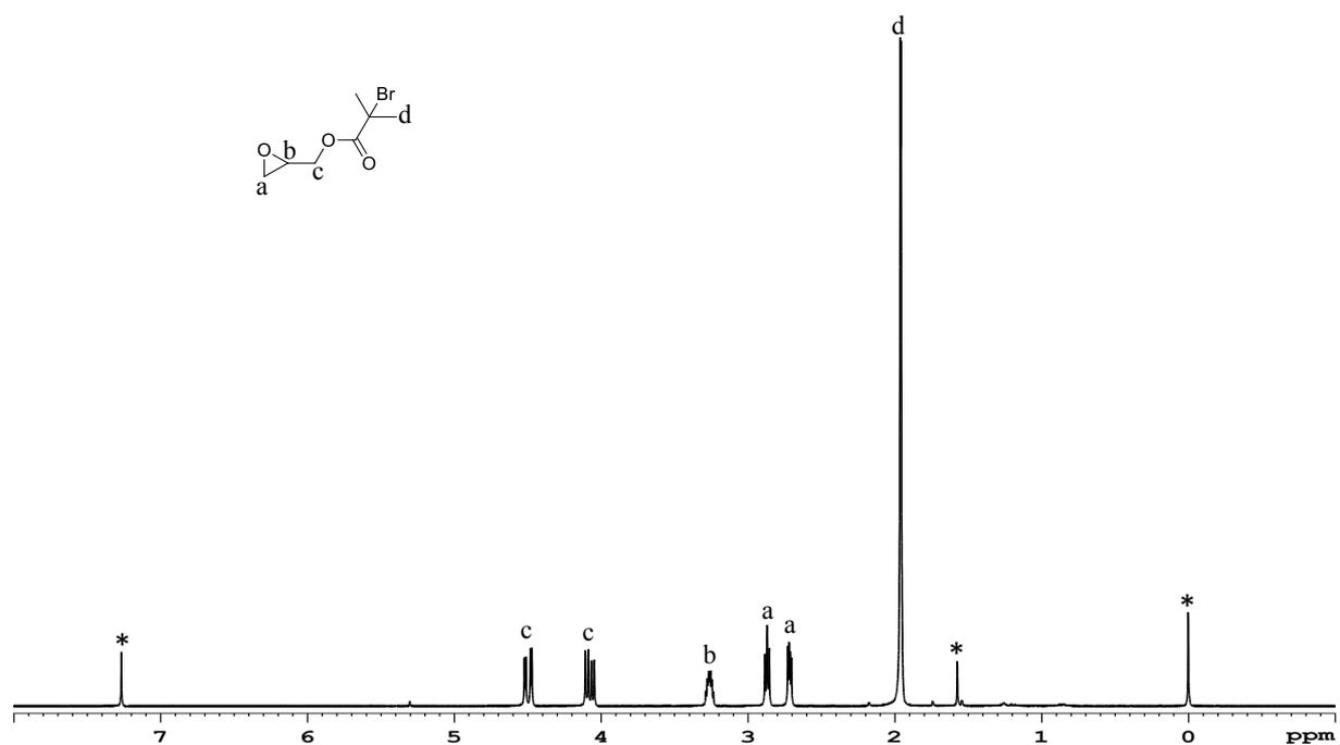
**Figure S1.** Chemical structure and <sup>1</sup>H NMR spectrum of **1** in CDCl<sub>3</sub>. TMS, water, and CHCl<sub>3</sub> signals are shown with an asterisk.
