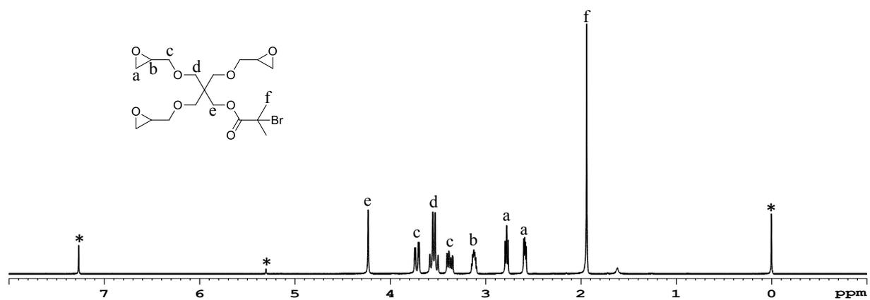
**Figure S3.** Chemical structure and  $^1\text{H}$  NMR spectrum of **3** in  $\text{CDCl}_3$ . TMS, DCM, and  $\text{CHCl}_3$  signals are shown with an asterisk.
