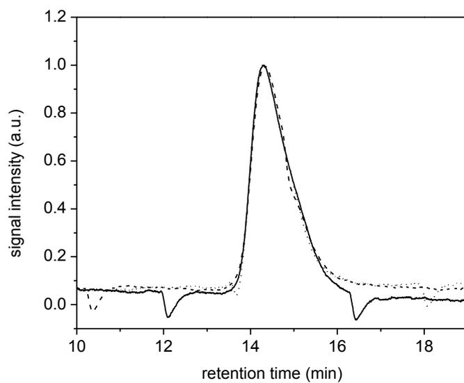
**Figure S5.** GPC chromatograms of polymer **5** (solid line), **8** (dash line), and **11** (dot line).
