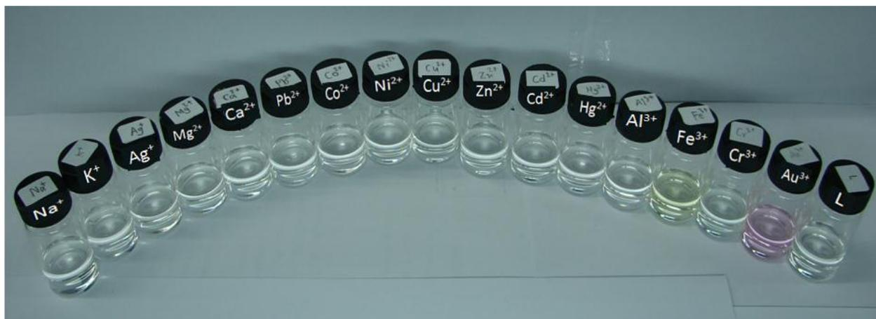
**Figure S3.** Color change and fluorescence changes of **PAA-Rho2** (0.1 g/L) in the presence of various cations.
