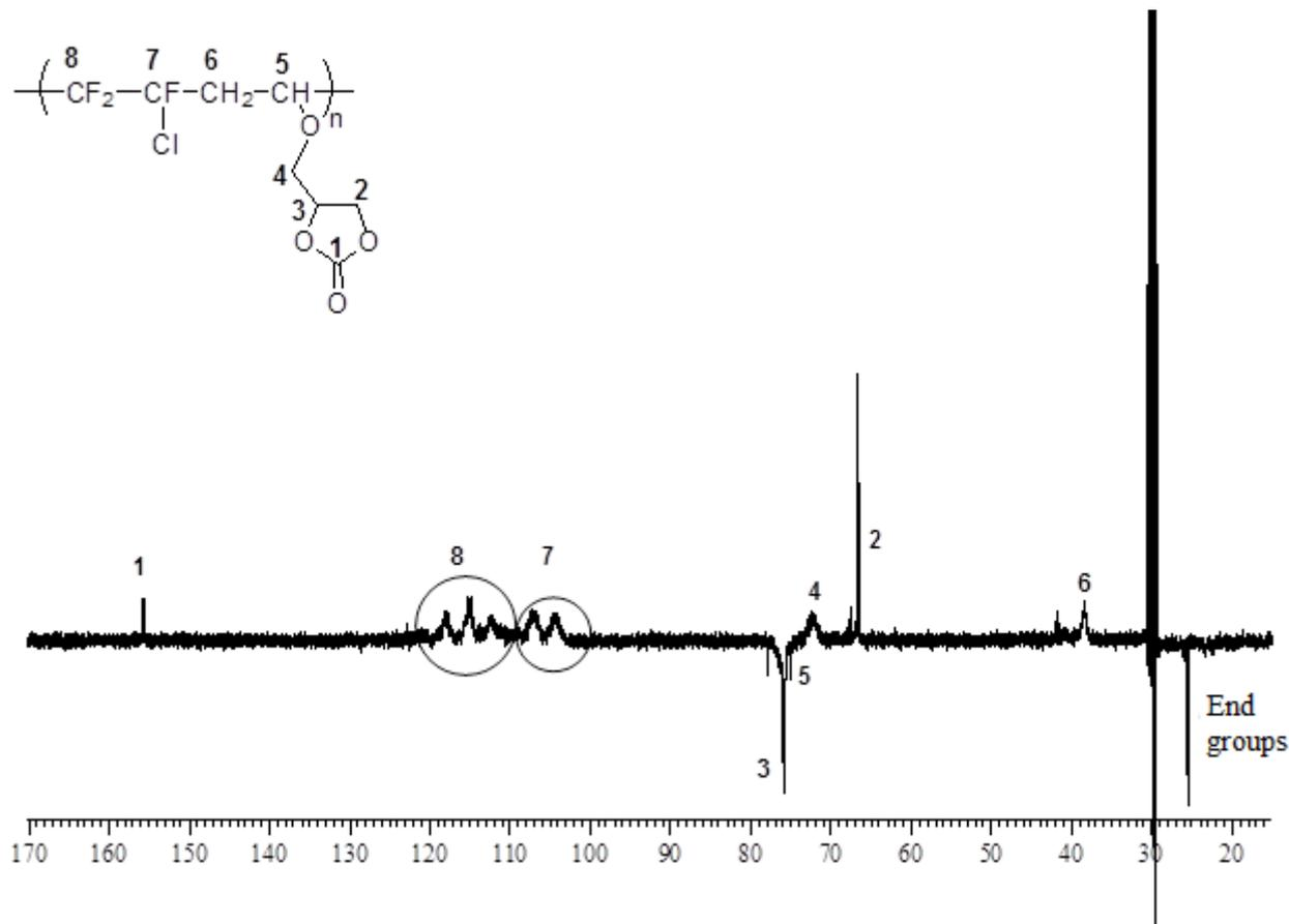
Figure S20:  $^{13}\text{C}$  NMR spectrum of poly(CTFE-*alt*-VE6) (**P5**) copolymer ( $\text{CDCl}_3$  at  $20^\circ\text{C}$ , 400 MHz).
