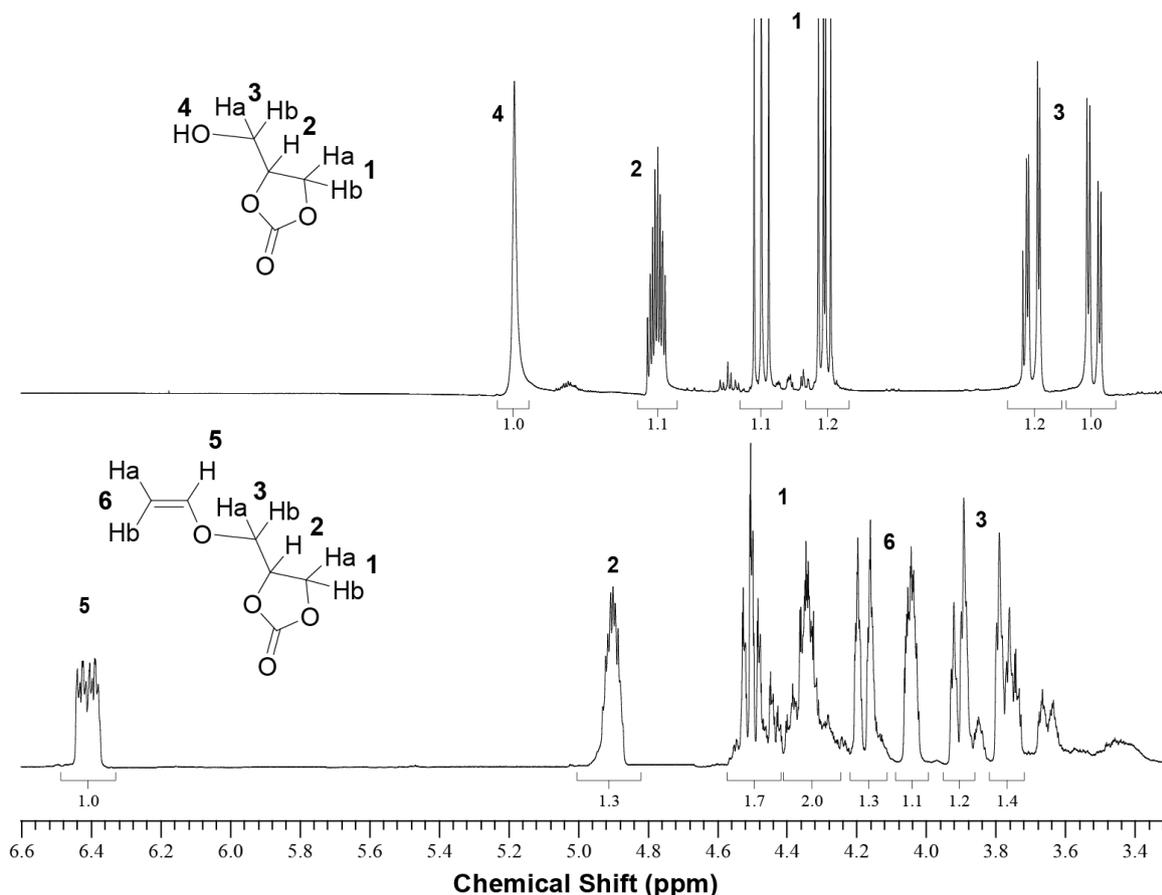
Figure S6: <sup>1</sup>H NMR spectra of glycerol carbonate vinyl ether (GCVE) (6) monomer (CDCl<sub>3</sub>, 20 °C, 400 MHz, lower spectrum) and glycerol carbonate (DMSO, 20 °C, 400 MHz, upper spectrum).
