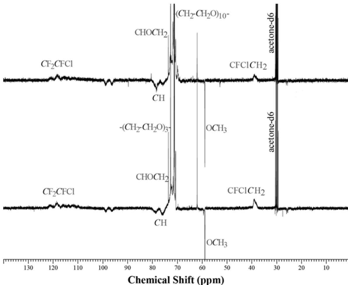
Figure S23:  $^{13}\text{C}$  NMR spectrum of poly(CTFE-*alt*-PEOVE3) copolymer (**P6**) (lower spectrum) and poly(CTFE-*alt*-PEOVE10) copolymer (**P7**) (upper spectrum) recorded in acetone- $\text{d}_6$  at room temperature.
