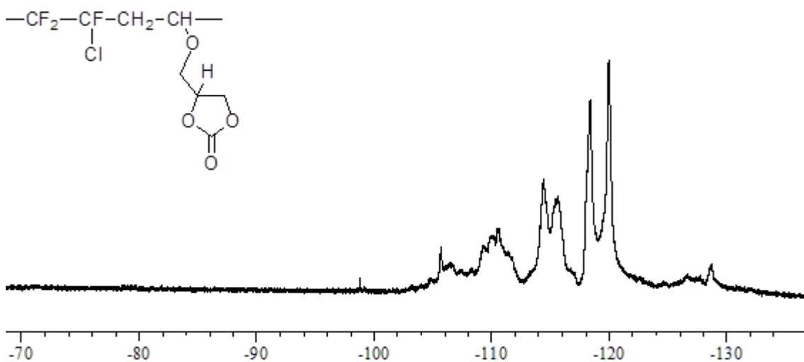
Figure S19: <sup>19</sup>F NMR spectrum of poly(CTFE-*alt*-VE6) copolymer (P5) (CDCl<sub>3</sub> at 20 °C, 400 MHz).
