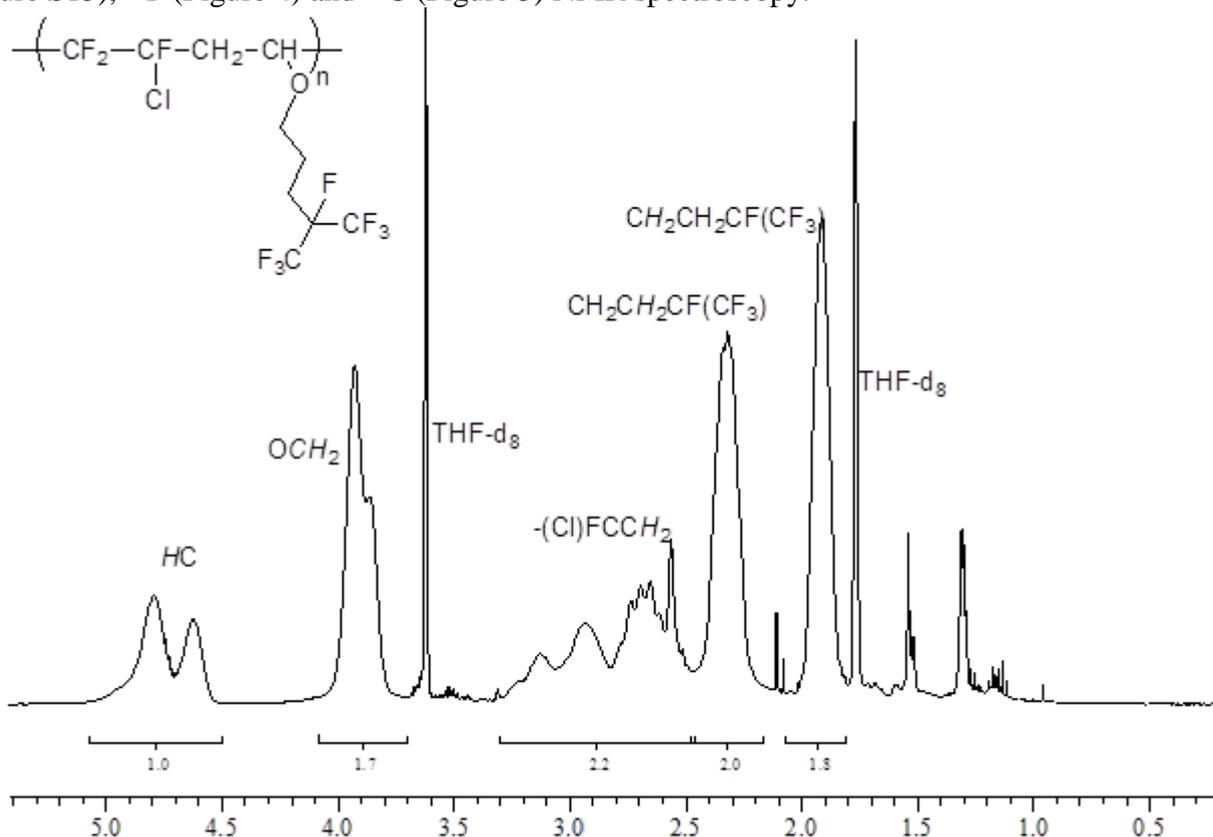
Figure S15: <sup>1</sup>H NMR spectrum of poly(CTFE-*alt*-VE4) (P3) copolymer (THF-*d*<sub>8</sub> at 20 °C, 400 MHz).
