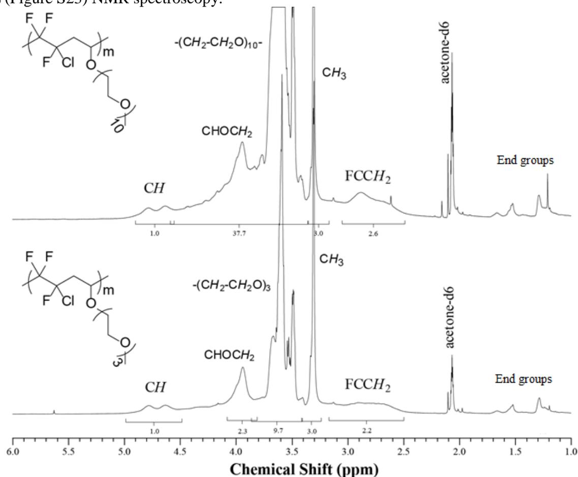
Figure S21:  $^1\text{H}$  NMR spectra of poly(CTFE-*alt*-PEOVE3) (**P6**) copolymer (lower spectrum) and poly(CTFE-*alt*-PEOVE10) (**P7**) copolymer (upper spectrum) recorded in acetone- $d_6$ .
