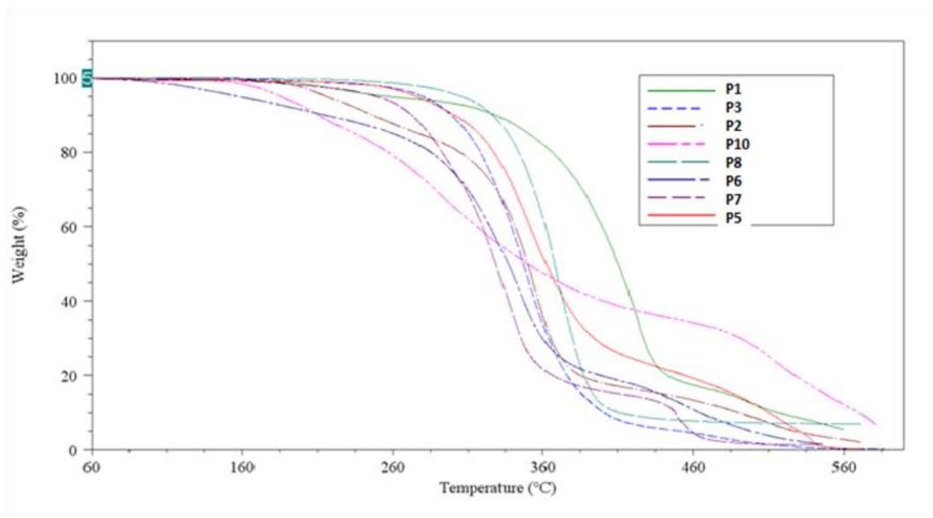
Figure S25: TGA thermograms of poly(CTFE-*alt*-VE) copolymers (**P1-3, 5-8, 10**) recorded under air at 10 °C.min<sup>-1</sup>.
