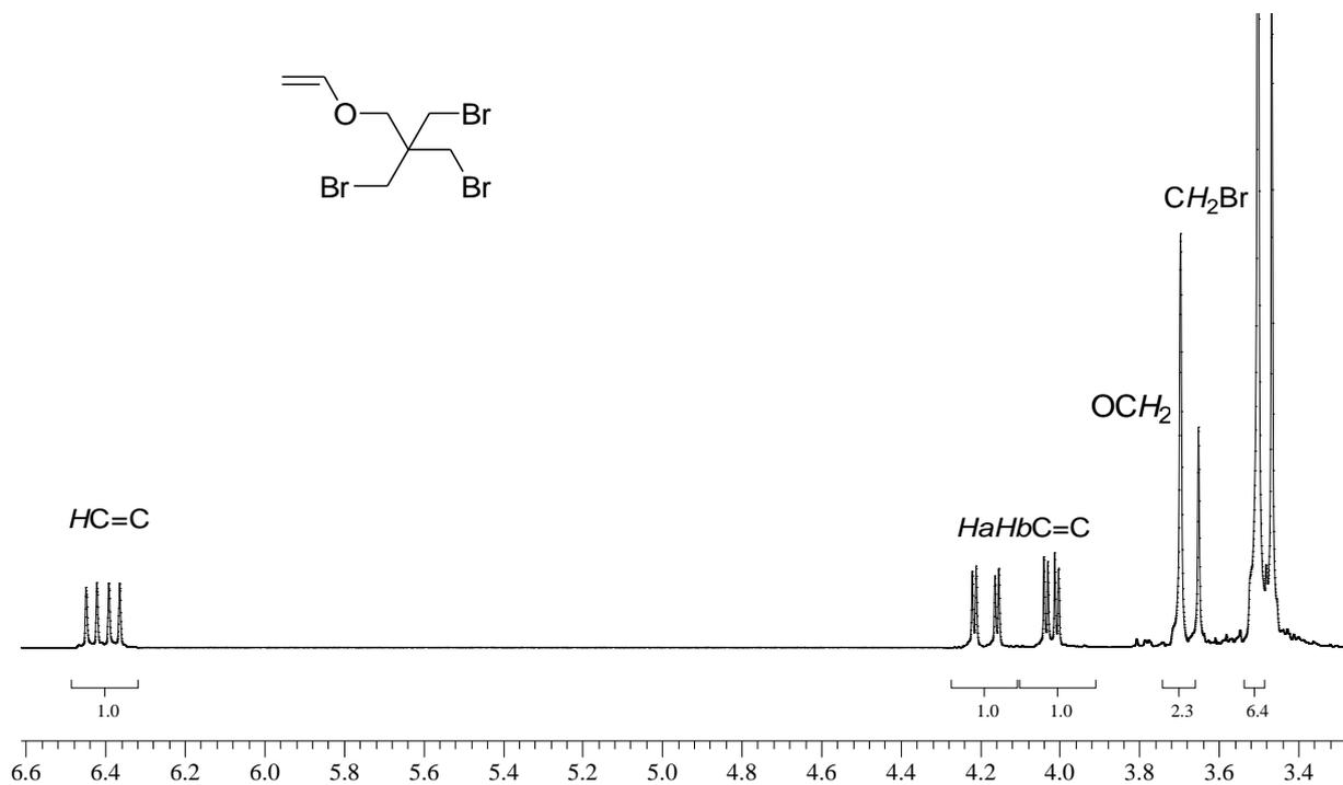
Figure S2: <sup>1</sup>H NMR spectrum of (3-bromo, 2,2-bis(bromomethyl) propyl vinyl ether (3) recorded in CDCl<sub>3</sub>.
