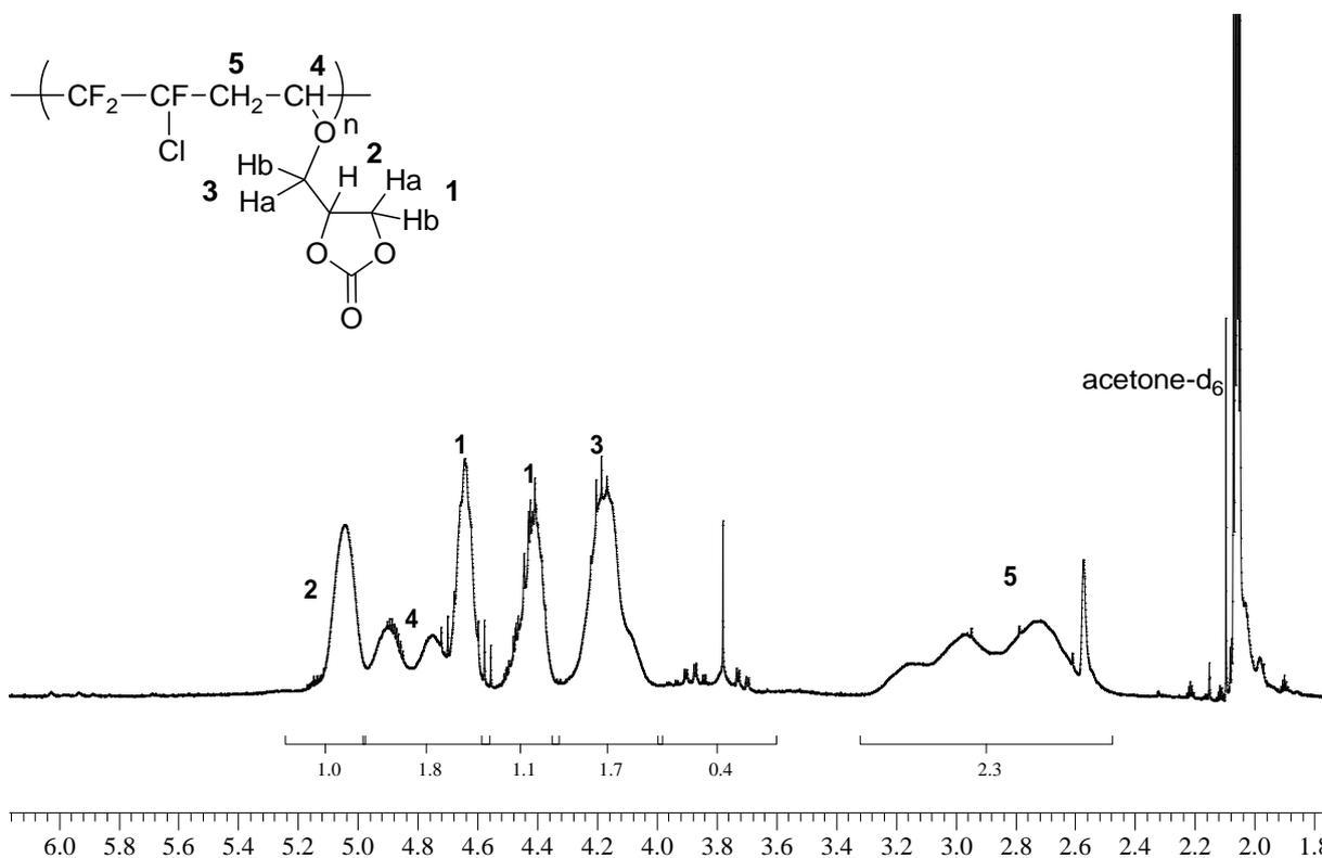
Figure S18: <sup>1</sup>H NMR spectrum of poly(CTFE-*alt*-VE6) (P5) copolymer (CDCl<sub>3</sub> at 20 °C, 400 MHz).
