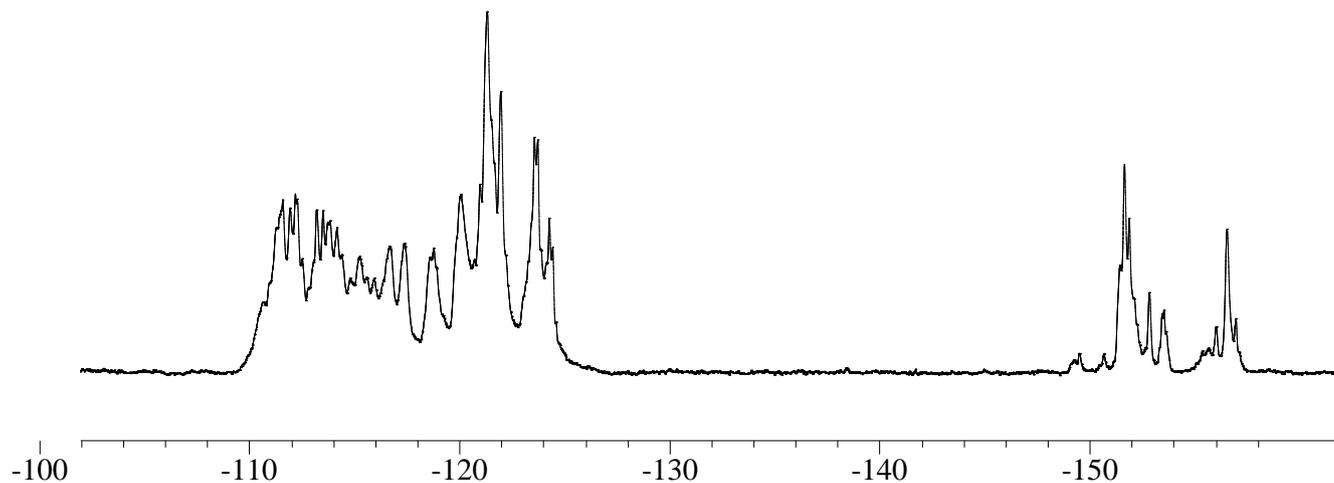
Figure S17:  $^{19}\text{F}$  NMR spectrum of poly(CTFE-*alt*-VE5) (**P4**) copolymer ( $\text{CDCl}_3$  at  $20^\circ\text{C}$ , 400 MHz).
