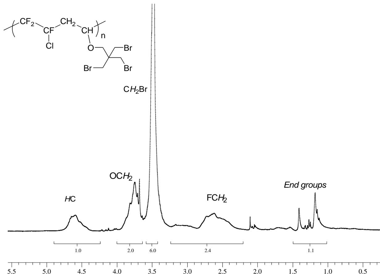
Figure S13: <sup>1</sup>H NMR spectrum of poly(CTFE-*alt*-VE3) (P2) copolymer (CDCl<sub>3</sub> at 20 °C, 400 MHz).
