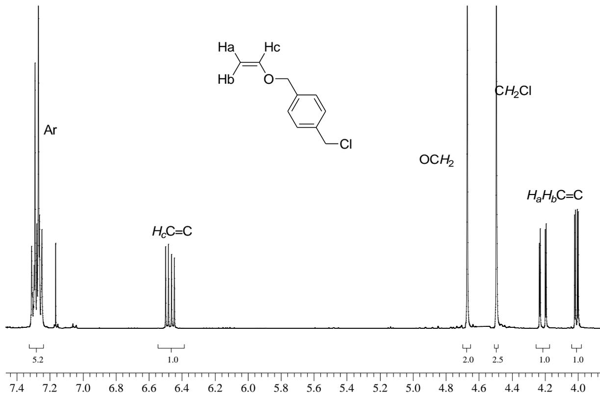
Figure S10: <sup>1</sup>H NMR spectrum of (*p*-methylchlorobenzyl) vinyl ether (**10**) recorded in CDCl<sub>3</sub>.
