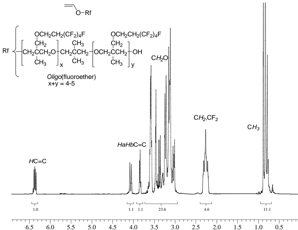
Figure S8: <sup>1</sup>H NMR spectrum of oligo(fluoroether) vinyl ether (**9**) recorded in CDCl<sub>3</sub>.
