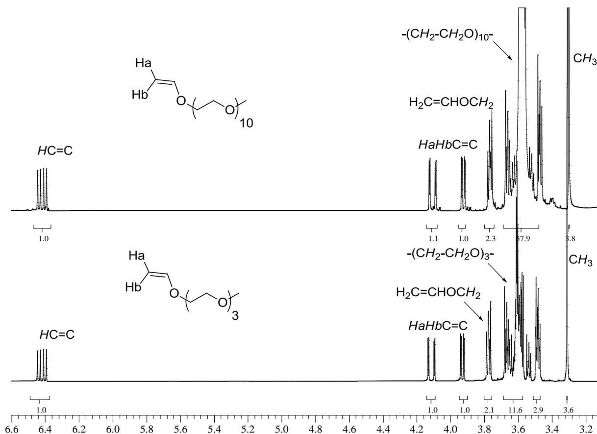
10 Figure S7: <sup>1</sup>H NMR spectra of PEOVE3 (**7**) (lower spectrum) and PEOVE10 (**8**) (upper spectrum) recorded in CDCl<sub>3</sub>.
