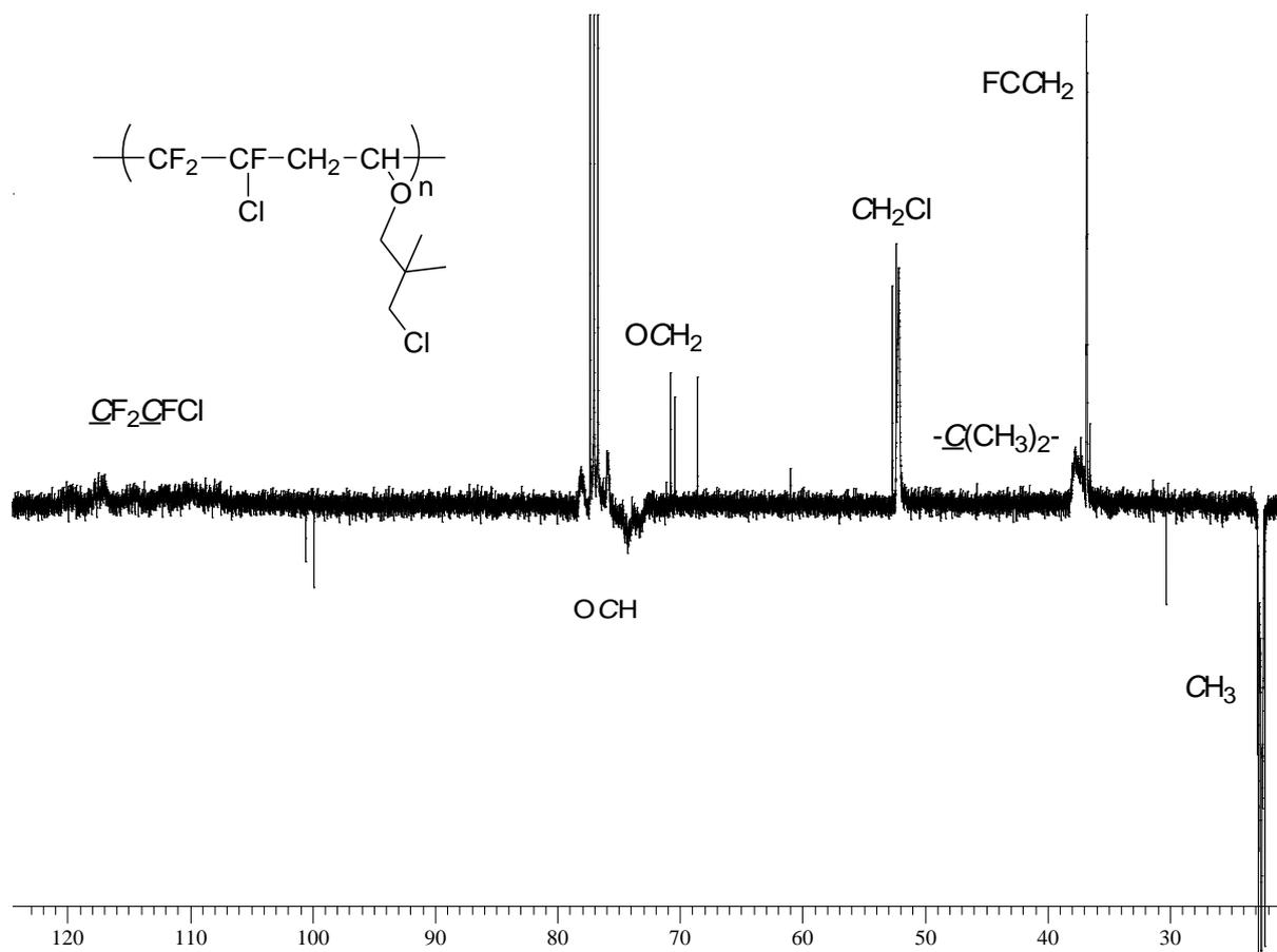
Figure S12: APT  $^{13}\text{C}$  NMR spectrum of poly(CTFE-*alt*-VE1) (P1) copolymer ( $\text{CDCl}_3$  at 20 °C, 400 MHz).
