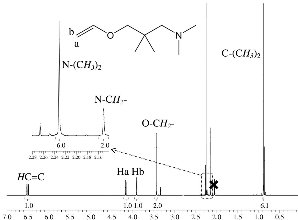
Figure S5:  $^1\text{H}$  NMR spectrum of 3-dimethylamino-(2,2-dimethylpropyl) vinyl ether MMPVE (**5**) recorded in  $\text{CDCl}_3$ .
