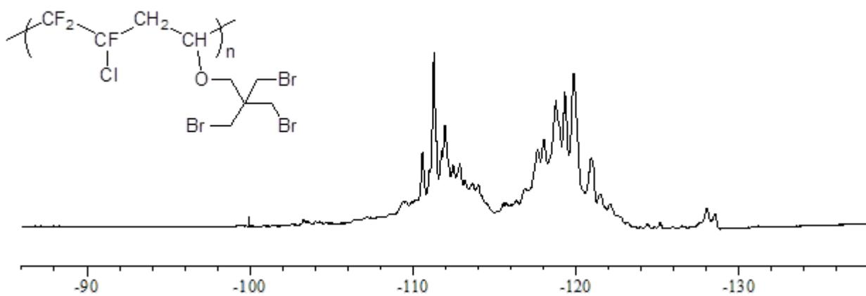
Figure S14: <sup>19</sup>F NMR spectrum of poly(CTFE-*alt*-VE3) (P2) copolymer (CDCl<sub>3</sub> at 20 °C, 400 MHz).
