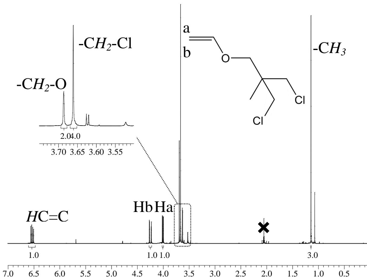
15 Figure S1: <sup>1</sup>H NMR spectrum of 3-chloro-2-chloromethyl-2-methyl-propyl vinyl ether (2) recorded in acetone d<sub>6</sub>.
