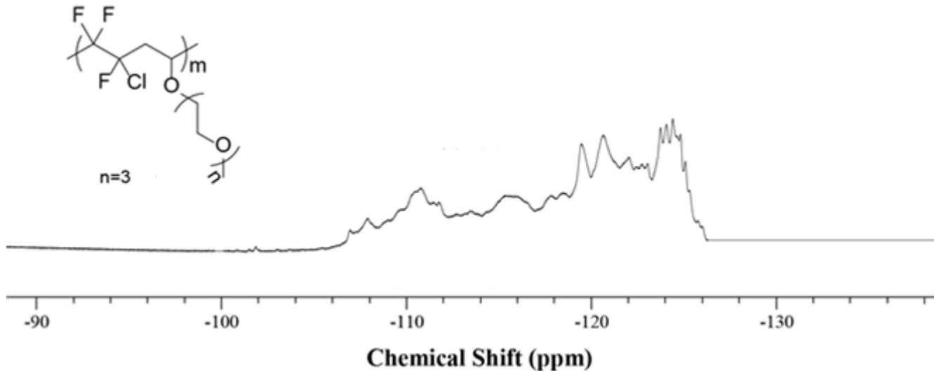
5 Figure S22:  $^{19}\text{F}$  NMR spectrum of poly(CTFE-*alt*-PEOVE3) copolymer (**P6**) recorded in acetone- $d_6$  at room temperature.
