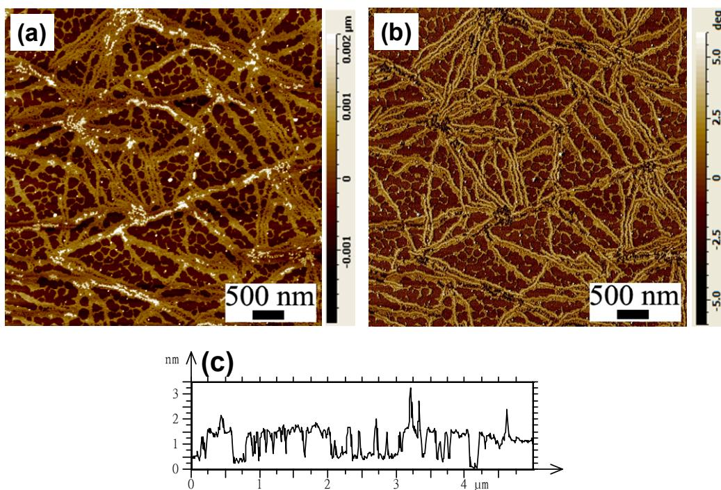
**Figure S4.** AFM topography (a) and phase (b) images of the P3HT monolayer nanowhiskers collected on Si wafer and dried without rinsing with chloroform. Nanocrystals can be distinguished from disordered P3HT molecules due to their different viscoelastic responses in the phase image. (c) Typical
