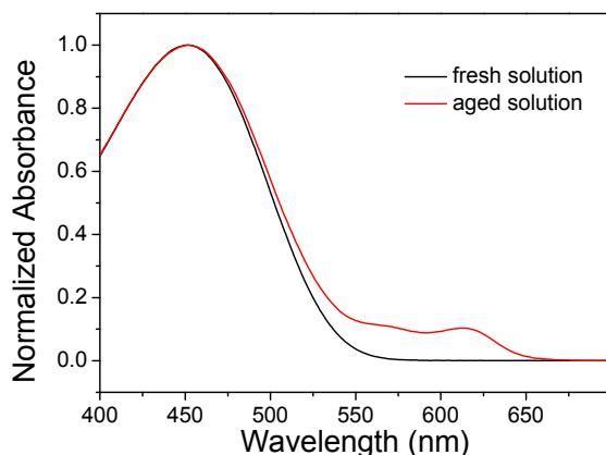
**Figure S1.** UV-vis spectra of fresh and aged P3HT/chloroform solution.
