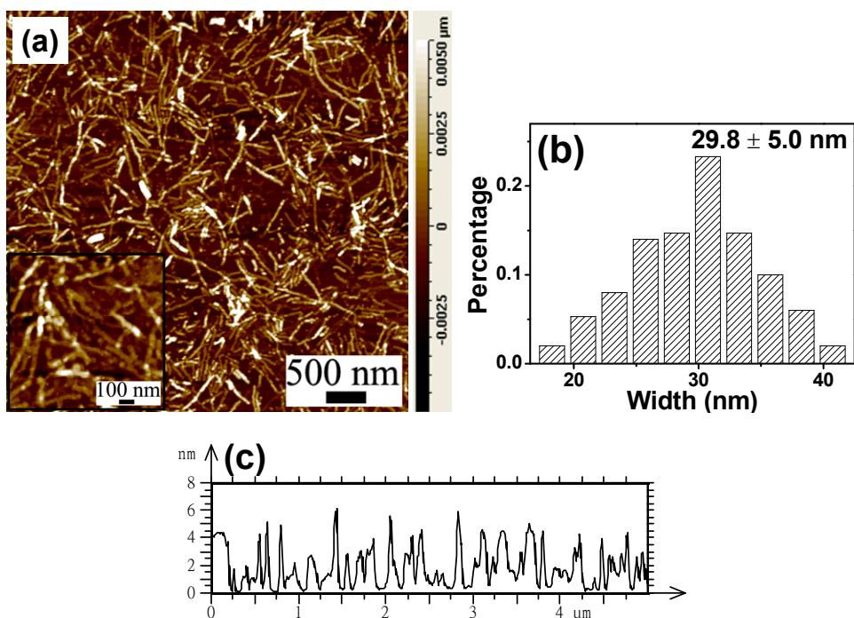
**Figure S3.** (a) AFM topography image of normal nanowhiskers prepared by the “whisker methods” from the same P3HT sample (inset is an enlarged view), and (b) width distribution and (c) typical cross section profile of (a).
