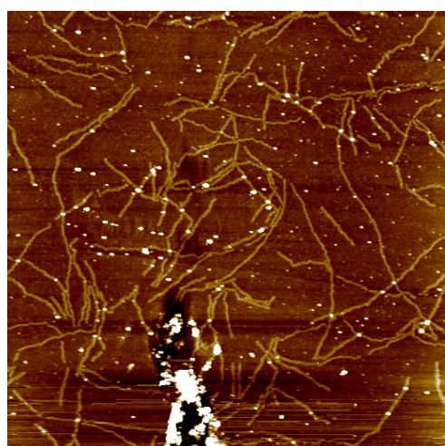
**Figure S5.** AFM topography image ( $10 \times 10 \mu\text{m}^2$ ) of the P3HT monolayer nanowhiskers collected on Si wafer from solution aged for 1 day.
