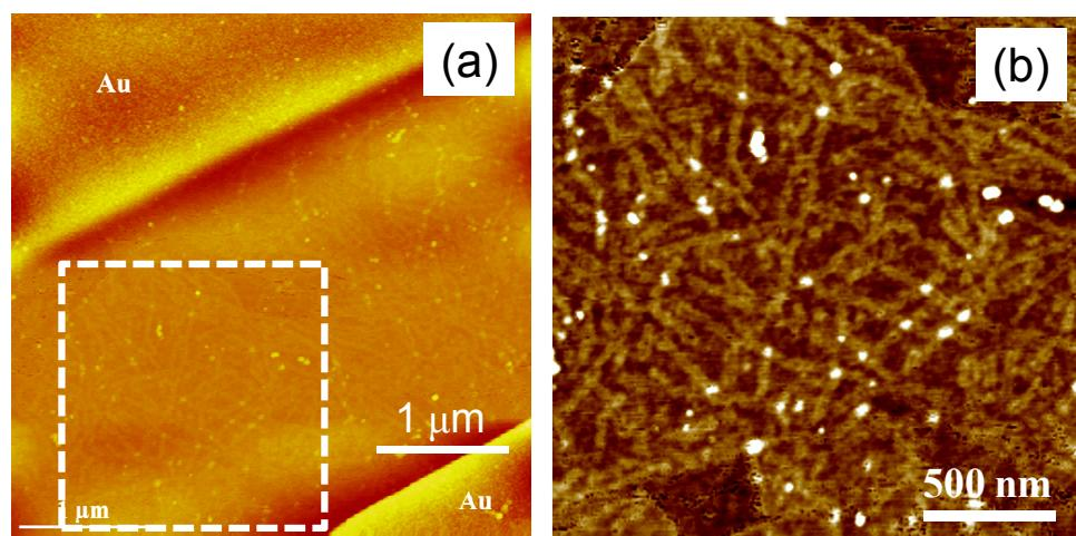
**Figure S6.** (a) AFM topography image of the P3HT monolayer nanowhiskers collected on a Si wafer used for FET measurements with Au electrodes. (b) An enlarged view of the area in the square marked by the dashed lines in (a).
