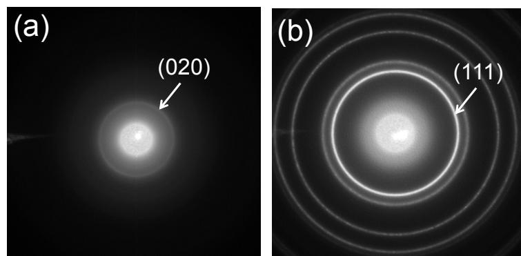
**Figure S2.** SAED patterns of (a) P3HT monolayer nanowhiskers and (b) thin gold film obtained under the same condition and shown in the same scale. The crystal plane distance  $d_{P3HT(020)}$  can be obtained by  $d_{P3HT} \cdot R_{P3HT} = d_{Au} \cdot R_{Au}$ , where  $R$  is the distance between the diffraction ring and central spot, and  $d_{Au(111)} = 0.2355$  nm.
