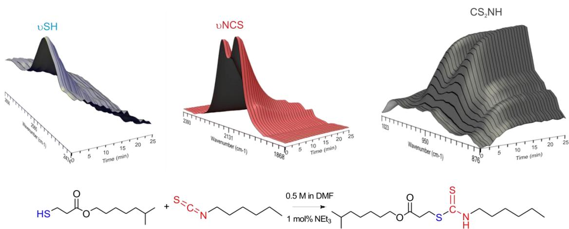
Fig. S1. Illustration of the online FT-IR waterfall plots for the thiol-isothiocyanate reaction.
