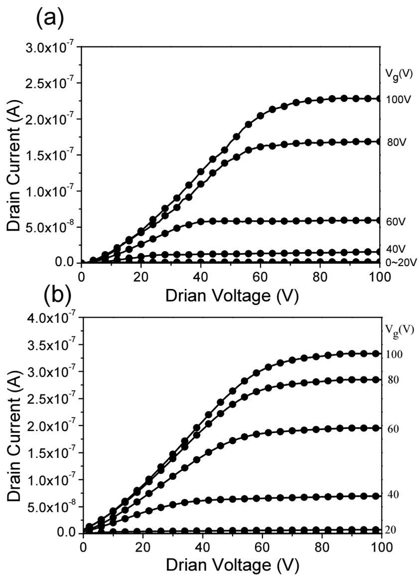
Figure S5. Output characteristics of the OFET device with (a) PVT and (b) PVTT as electret.
