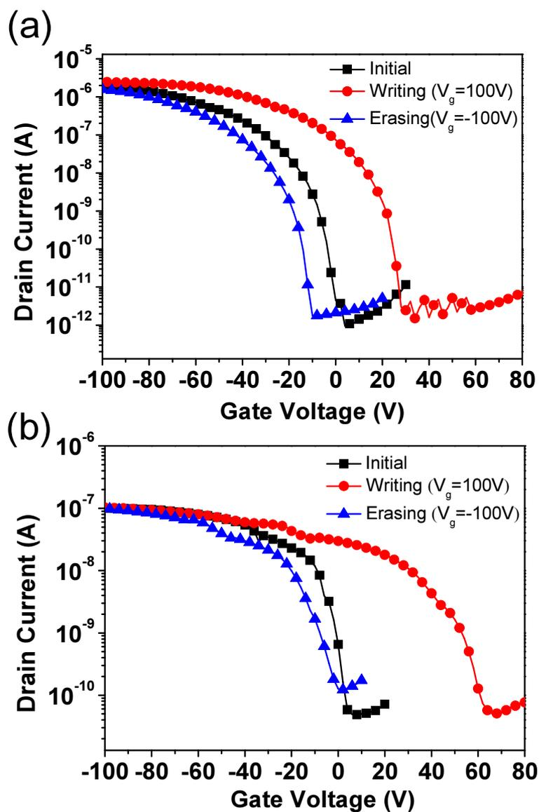
Figure S6. Shifts in transfer curves for pentacene OFET memory device with (a) PVT and (b) PVTT as polymer electrets.
