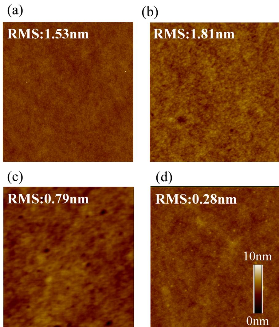
Figure S4. Atomic force microscopy (AFM) topographies of (a) PVT, (b) PVTT, (c) PStFl, and (d) PS spin-coated on bare  $\text{SiO}_2$  substrates on  $1 \mu\text{m} \times 1 \mu\text{m}$  areas.
