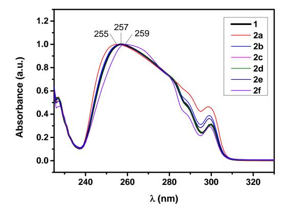
**SI. Figure 1.** Noarmalized UV-vis absorption spectra of monomer **1** (50 ppm) and polymers **2a-f** (100 ppm) in CHCl<sub>3</sub>
