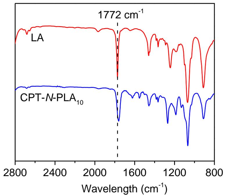
**Figure S1:** FT-IR spectra of lactide (LA, red) and CPT-N-PLA<sub>10</sub> conjugates (blue).
