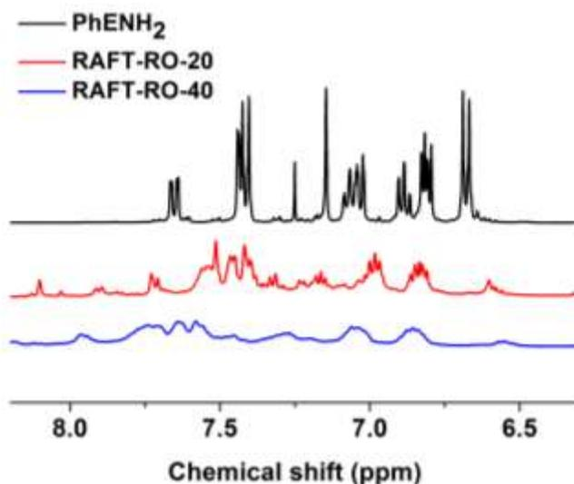
Fig. S3  $^1\text{H}$  NMR spectra of **PhENH<sub>2</sub>**, **RAFT-RO-20** and **RAFT-RO-40** dissolved in  $\text{d}_6$ -DMSO.
