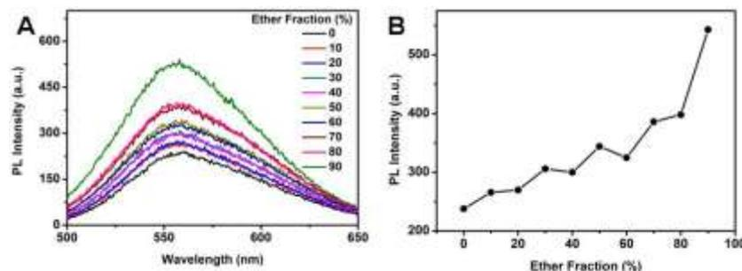
**Fig. S2** The AIE characteristic of **PhENH<sub>2</sub>** ( $\lambda_{\text{Ex}} = 490$  nm): (A) PL spectra of **PhENH<sub>2</sub>** in DMF-ether mixtures with different ether fractions; (B) the changes in PL peak intensity of the compound in different ether fraction mixtures.
