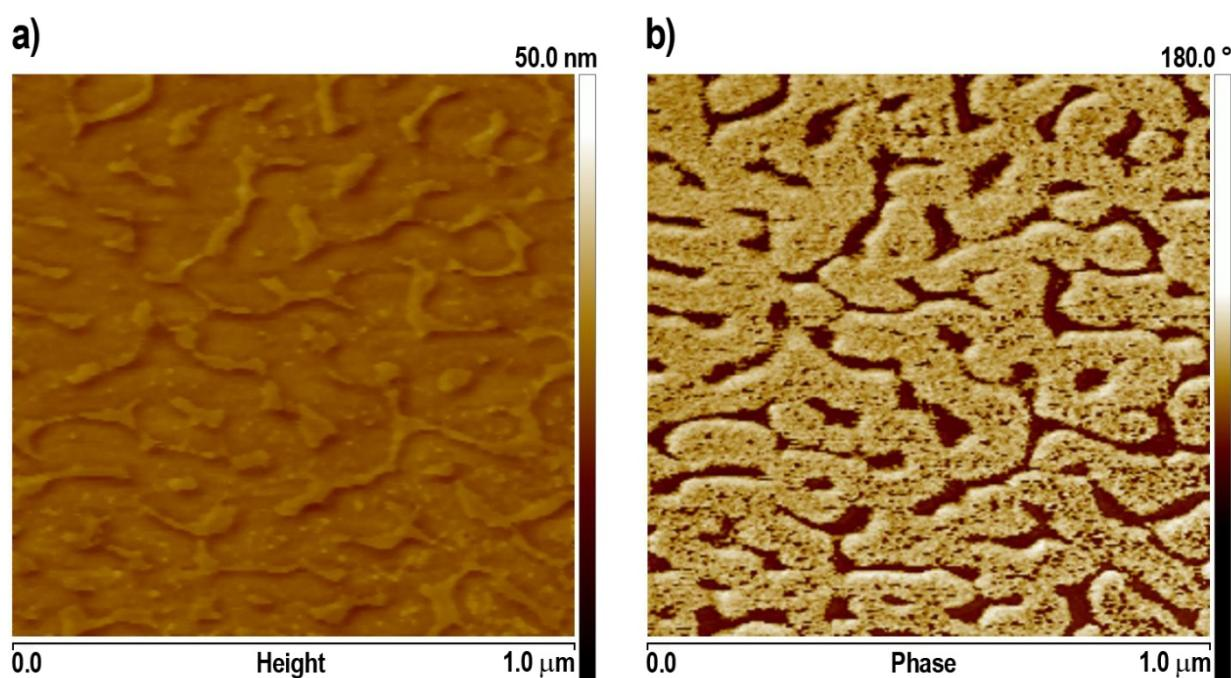
**Fig. S7.** Height (a) and phase (b) 2D TM-AFM micrographs of sample 3 of Table 1 corresponding to the 3D micrographs in Figure 5c.
