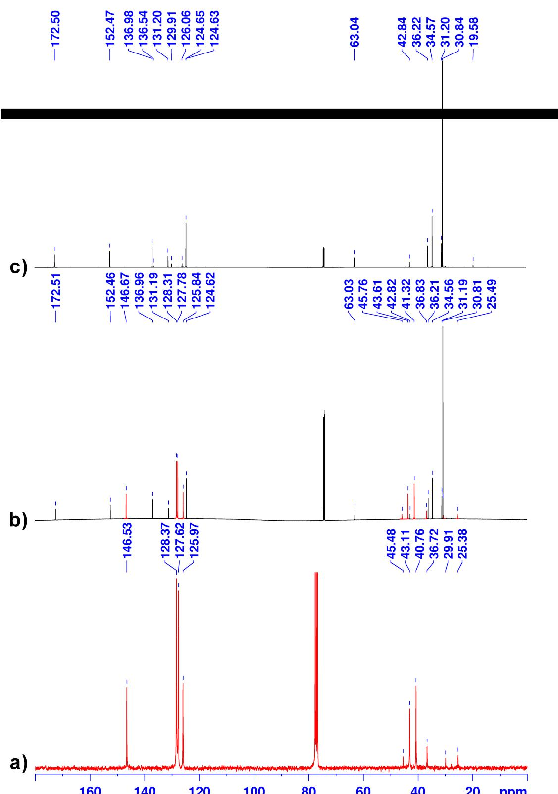
**Fig. S3.**  $^{13}\text{C}$  NMR spectra of: a) sample 6; b) TREF fraction collected at 30 °C containing the sample 6 (signals highlighted in red) and pentaerythritol tetrakis(3-(3,5-di-tert-butyl-4-hydroxyphenyl)propionate) (added to the eluent as stabilizer); c) TREF fraction collected at 130 °C containing pentaerythritol tetrakis(3-(3,5-di-tert-butyl-4-hydroxyphenyl)propionate).
