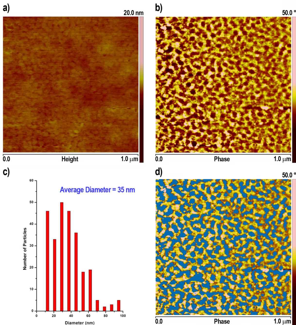
**Fig. S10.** Height (a) and phase (b) 2D TM-AFM micrographs of sample 6 of Table 1 corresponding to the 3D micrographs in Figure 5e. c) Dimension distribution analysis of iP(E-*alt*-S) domains in Figure (b) performed with Nanoscope Analysis v1.40 r2sr1 software from Bruker as shown in Figure d.
