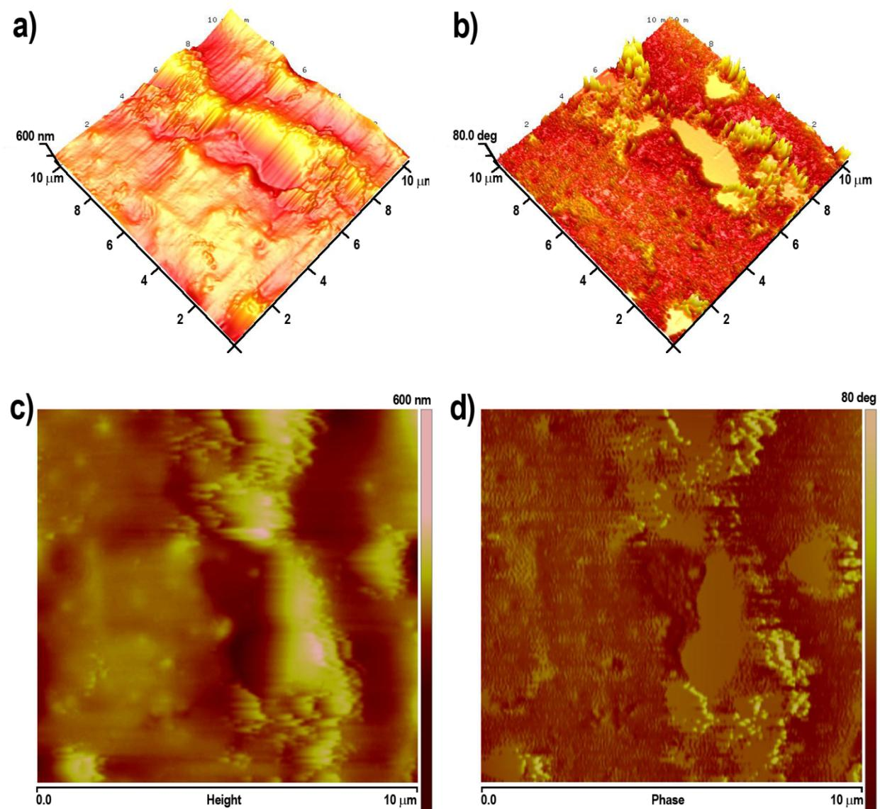
**Fig. S12.** Height (a and c) and phase (b and d) TM-AFM micrographs of a solution blend of iPS homopolymer and iP(E-*alt*-S) alternate copolymer sample 1 (50:50 by weight), illustrating the large scale raw phase separation.
