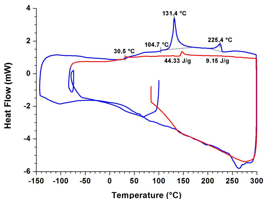
**Fig. S4.** DSC trace of sample 2 annealed at 100 °C for 5 min: 1<sup>st</sup> run (blue curve) and 2<sup>nd</sup> run (red curve).
