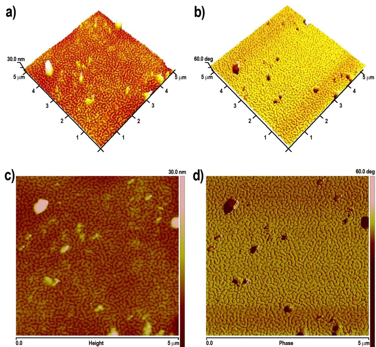
**Fig. S9.** Height (a and c) and phase (b and d) TM-AFM micrographs a iPS-*b*-iP(E-*alt*-S) diblock copolymer sample 4, illustrating the large scale formation of bicontinuous phases.
