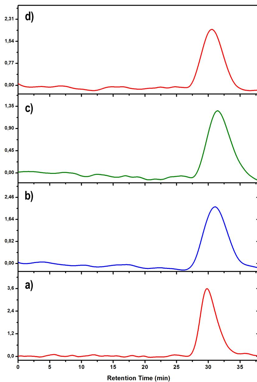
**Fig. S1.** GPC chromatograms at 135 °C of: a) sample 2, b) sample 3, c) sample 4 and d) sample 5 of Table 1.
