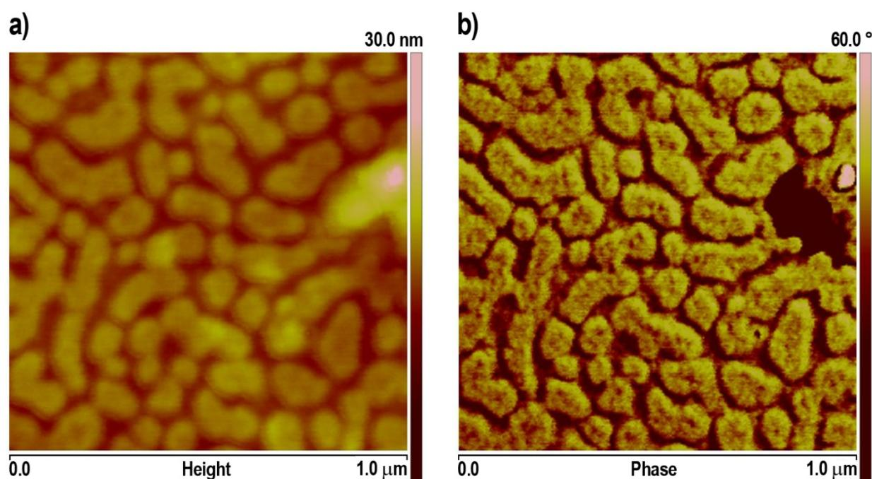
**Fig. S8.** Height (a) and phase (b) 2D TM-AFM micrographs of sample 4 of Table 1 corresponding to the 3D micrographs in Figure 5d.
