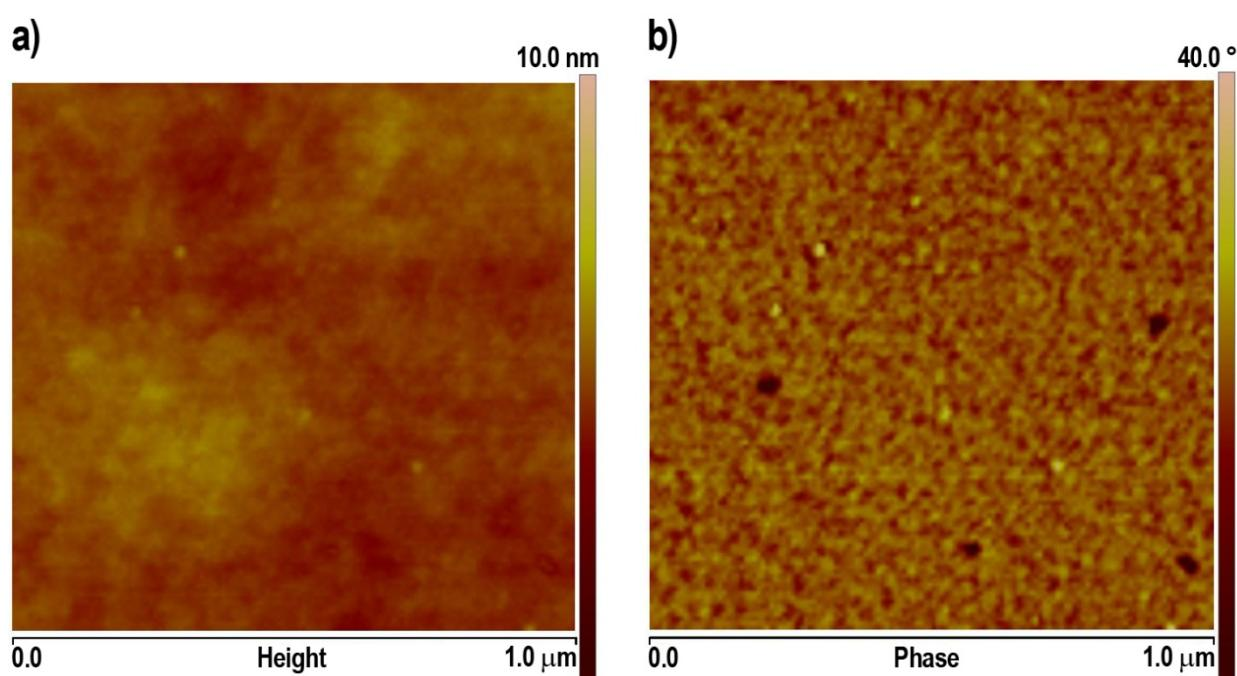
**Fig. S11.** Height (a) and phase (b) 2D TM-AFM micrographs of a thin film of iPS homopolymer (sample 7) corresponding to the 3D micrographs in Figure 5f.
