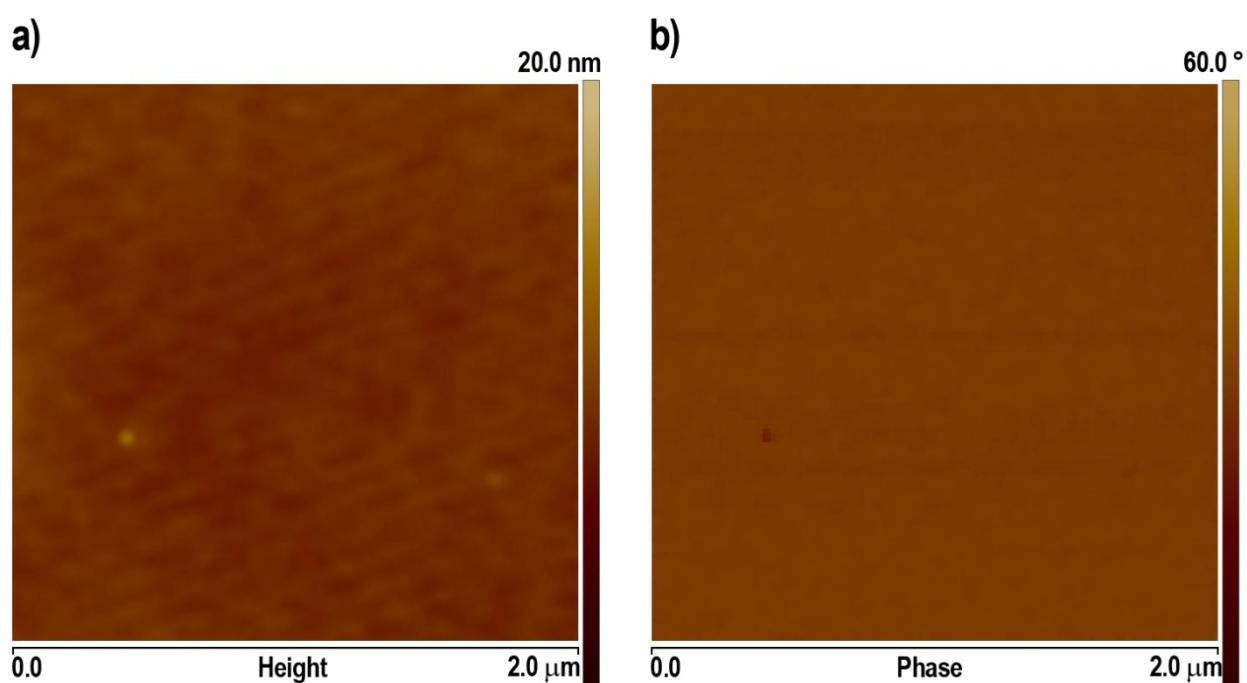
**Fig. S5.** Height (a) and phase (b) 2D TM-AFM micrographs of sample 1 of Table 1 corresponding to the 3D micrographs in Fig. 5a.
