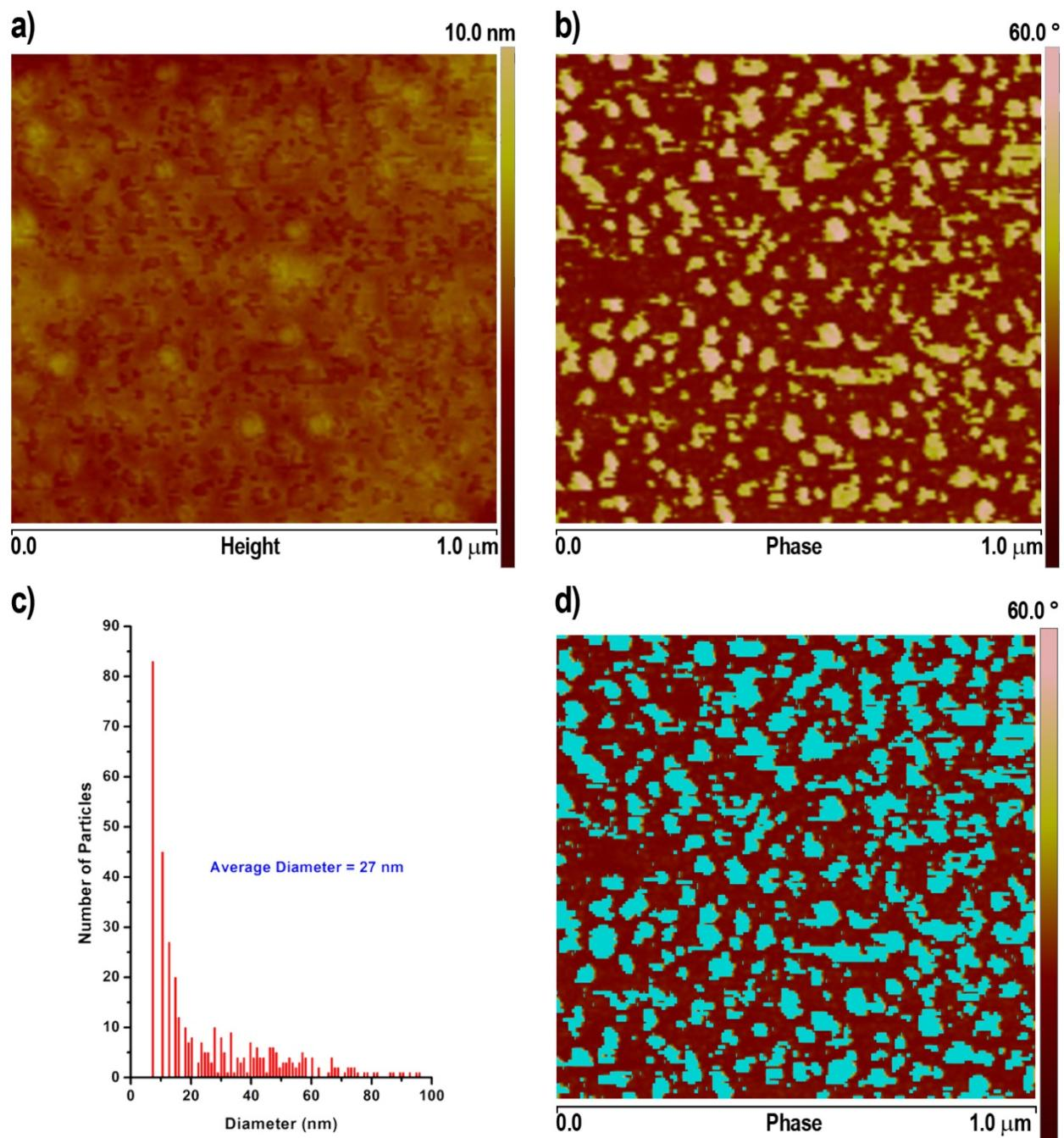
**Fig. S6.** Height (a) and phase (b) 2D TM-AFM micrographs of sample 2 of Table 1 corresponding to the 3D micrographs in Fig. 5b. Dimension distribution analysis (c) of iPS domains in Figure (b) performed with Nanoscope Analysis v1.40 r2sr1 software from Bruker as shown in Figure (d).
