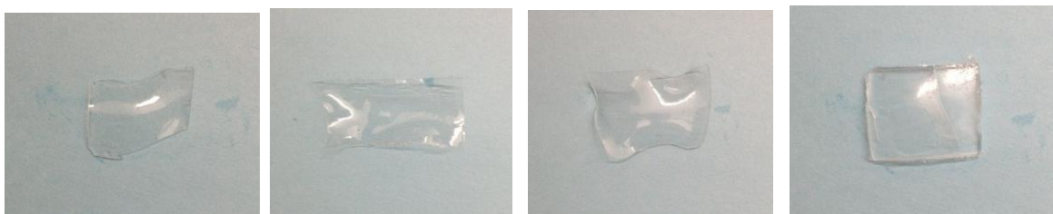
Figure S3. Photos of film samples of the products of 100% PEODMA between two glass slides with the gap between the slides sealed and aluminum foil as the spacer of 4, 8, 16, and 32 layers (from left to right) thermally crosslinked at 70 °C.
