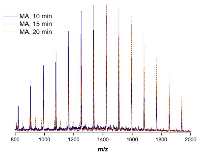
**Figure S6:** Full ESI-MS spectra of pMA (target  $M_n = 2000 \text{ g} \cdot \text{mol}^{-1}$ ) obtained by UV-induced copper-mediated radical polymerization at residence times of 10, 15 and 20 minutes in the milli-flow reactor
