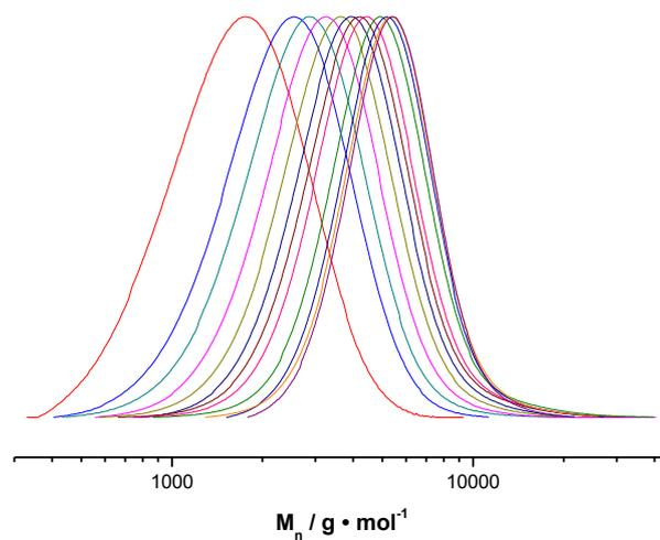
**Figure S5:** Molecular weight distributions with increasing residence time in the milli-flow reactor during a UV-induced copper-mediated radical polymerization of MA (target  $M_n = 9800 \text{ g} \cdot \text{mol}^{-1}$ ).
