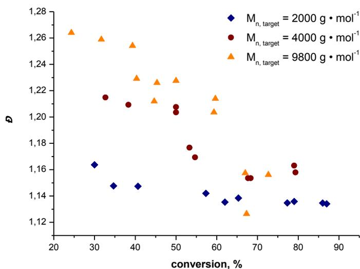
**Figure S2:** Decrease of the dispersity with monomer conversion of MA polymerizations in a milli-flow reactor via UV-induced copper-mediated radical polymerization, with target  $M_n = 2000$  (◆), 4000 (●) and 9800 (▲)  $\text{g} \cdot \text{mol}^{-1}$ .
