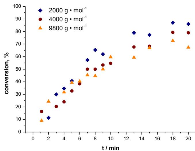
**Figure S1:** Evolution of monomer conversion with reaction time of UV-induced copper-mediated radical polymerization of MA in the milli-flow reactor with target  $M_n = 2000$  (◆), 4000 (●) and 9800 (▲)  $\text{g} \cdot \text{mol}^{-1}$ .
