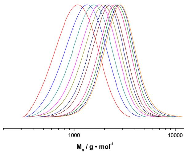
**Figure S4:** Molecular weight distributions with increasing residence time in the milli-flow reactor during a UV-induced copper-mediated radical polymerization of MA (target  $M_n = 4000 \text{ g} \cdot \text{mol}^{-1}$ )
