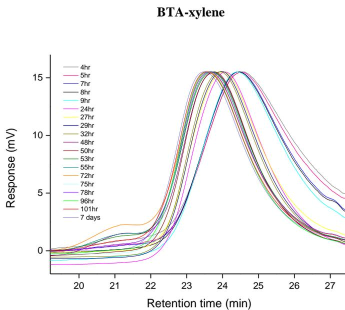
Figure S4. GPC traces during the RAFT polymerization of CB using TBTA in xylene.
