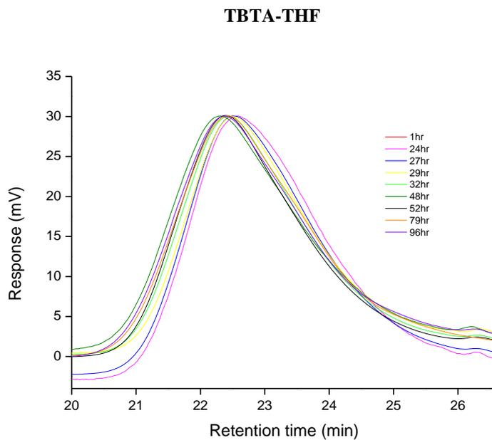
Figure S8. GPC traces during the RAFT polymerization of CB using TBTA in THF.
