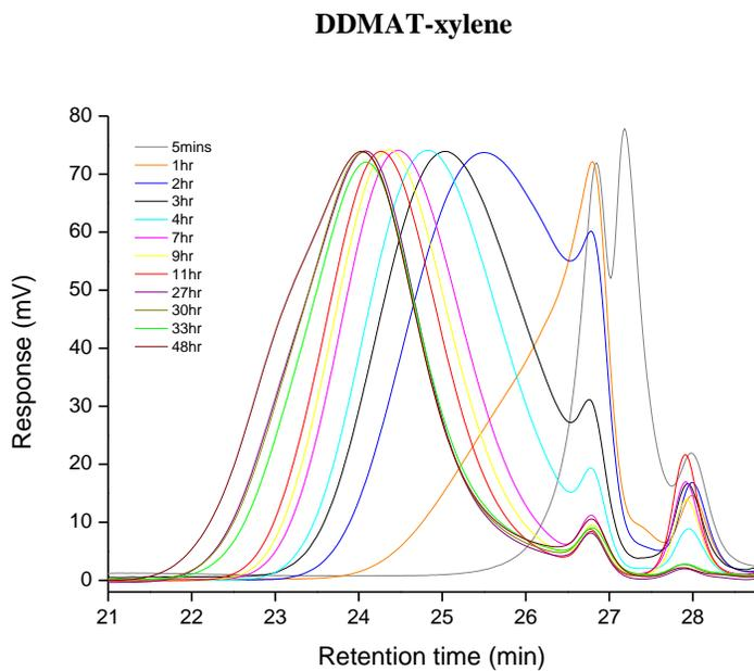
Figure S3. GPC traces during the RAFT polymerization of CB using DDMAT in xylene.
