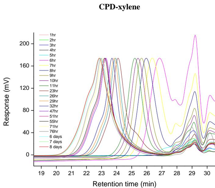
Figure S2. GPC traces during the RAFT polymerization of CB using CPD in xylene.
