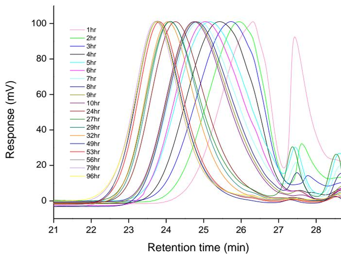
Figure S7. GPC traces during the RAFT polymerization of CB using DDMAT in THF.
