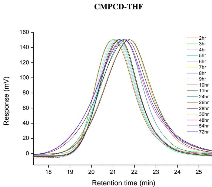
Figure S5. GPC traces during the RAFT polymerization of CB using CMPCD in THF.
