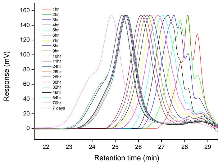
Figure S6. GPC traces during the RAFT polymerization of CB using CPD in THF.
