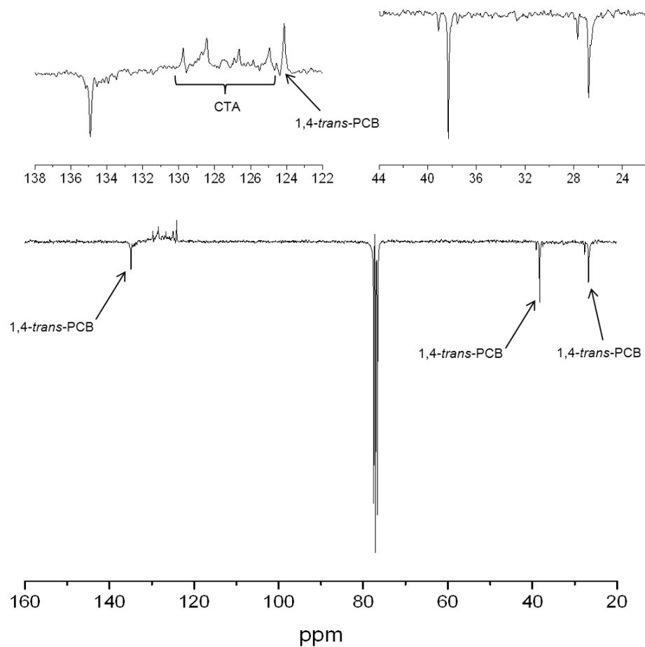
Figure S11. PENDANT <sup>13</sup>C NMR spectrum of PCB synthesized using CPD. The following analytical data correspond to the main 1,4-*trans* isomer, with remaining peaks arising from the minor isomers and CTA chain-ends, (75 MHz, CDCl<sub>3</sub>, δ ppm): reference CDCl<sub>3</sub> = 77.17 ppm, δ = 134.86 (—CH<sub>2</sub>C(Cl)C(H)CH<sub>2</sub>—), 124.08(—CH<sub>2</sub>C(Cl)C(H)CH<sub>2</sub>—), 38.29 (—CH<sub>2</sub>C(Cl)C(H)CH<sub>2</sub>—), 26.75 (—CH<sub>2</sub>C(Cl)C(H)CH<sub>2</sub>—).
