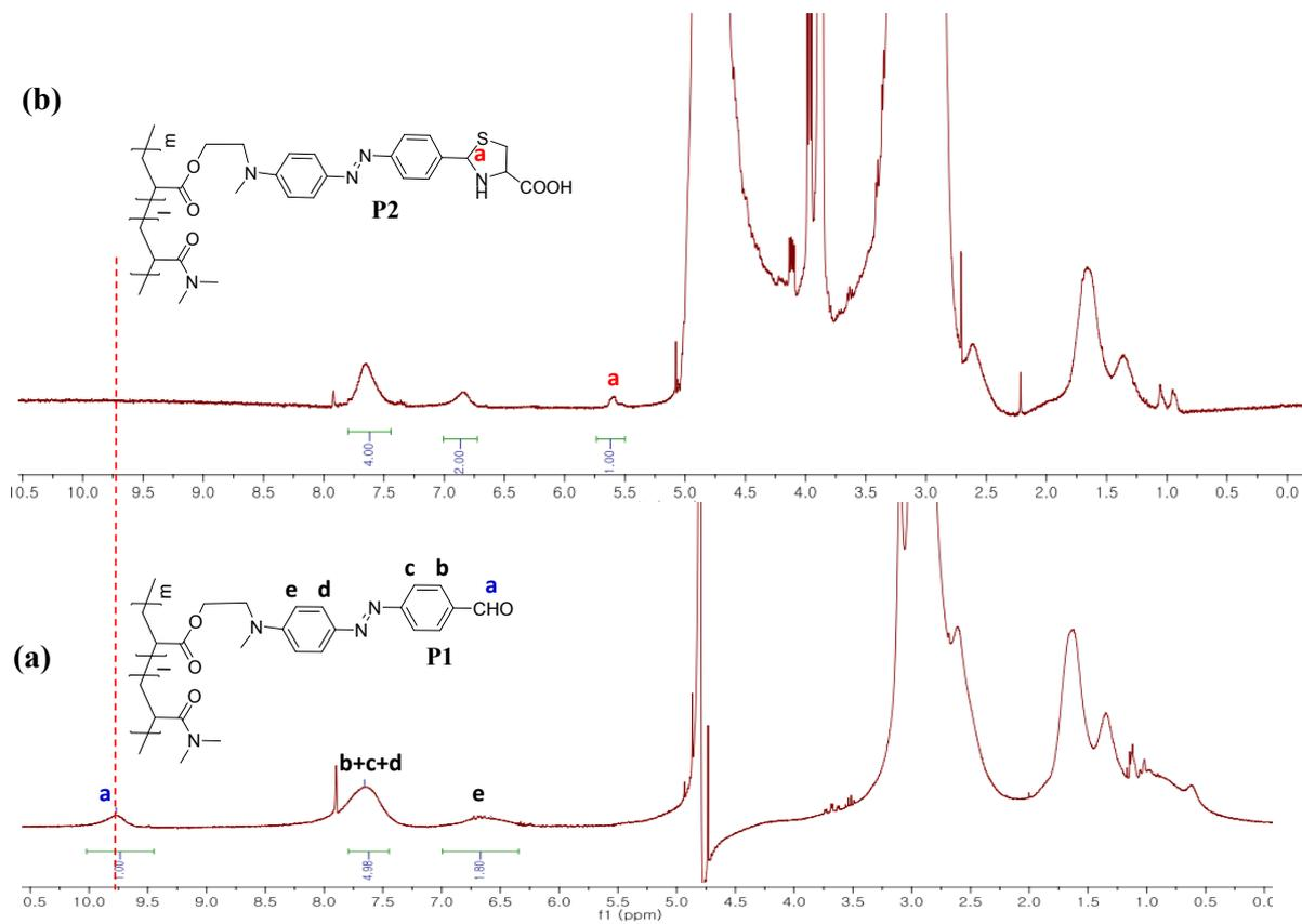
**Figure S2.**  $^1\text{H-NMR}$  spectra (a) the polymer (P1) and (b) P1 with cysteine (P2) at 25 °C in  $\text{D}_2\text{O}$ .
