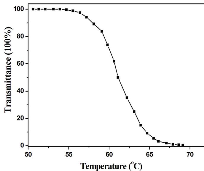
**Figure S9:** The plot of percent transmission vs temperature of polymer P1.
