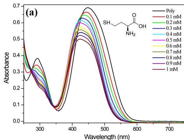
**Figure S3:** UV-Vis absorption spectra of P1 ( $2.5 \times 10^{-4} M$ ) with various concentrations of (a) homocysteine.
