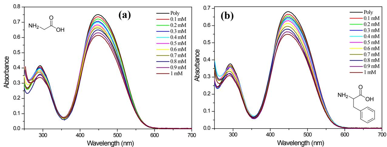
**Figure S7:** UV-Vis absorption spectra of ( $2.5 \times 10^{-4} M$ ) with various concentrations of (a) glycine and (b) phenylalanine.
