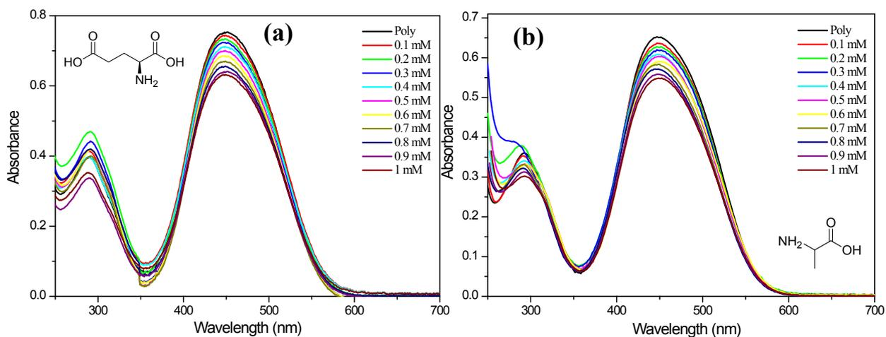
**Figure S5:** UV-Vis absorption spectra of ( $2.5 \times 10^{-4} M$ ) with various concentrations of (a) glutamic acid and (b) alanine.
