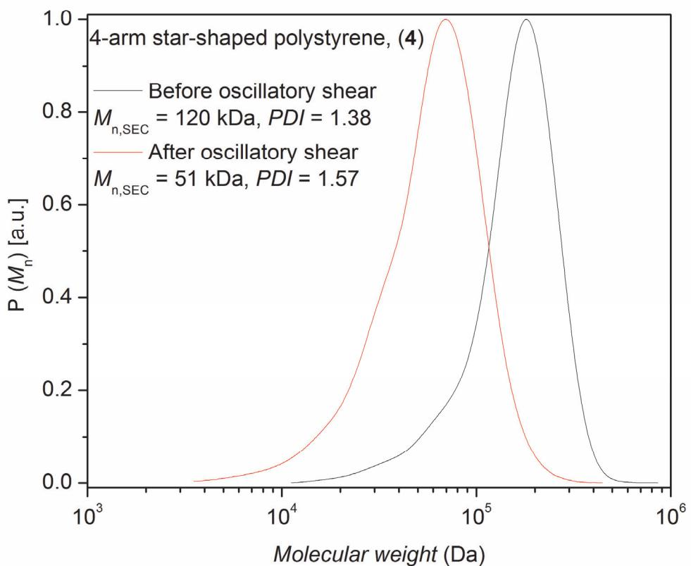
**Figure S6.** SEC trace of the trithiocarbonate core-functional 4-arm star-shaped polystyrene (4) before and after applying oscillatory shear with  $\omega/2\pi = 0.05 \text{ Hz}$  and  $\gamma_0 = 0.25$  strain amplitude at  $180^\circ \text{C}$  in a nitrogen atmosphere.
