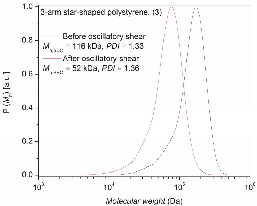
**Figure S5.** SEC trace of the trithiocarbonate core-functional 3-arm star-shaped polystyrene (3) before and after 8 hours applying oscillatory shear with  $\omega/2\pi = 0.05$  Hz and  $\gamma_0 = 0.25$  strain amplitude at 180 °C in a nitrogen atmosphere via DRI detector.
