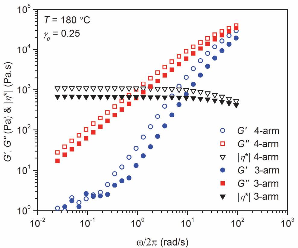
**Figure S7.** Dynamic frequency sweep test of star polystyrenes at the end of dynamic time sweep test after 8 hours (refer to Figure 8 in the main text) in rheometer.
