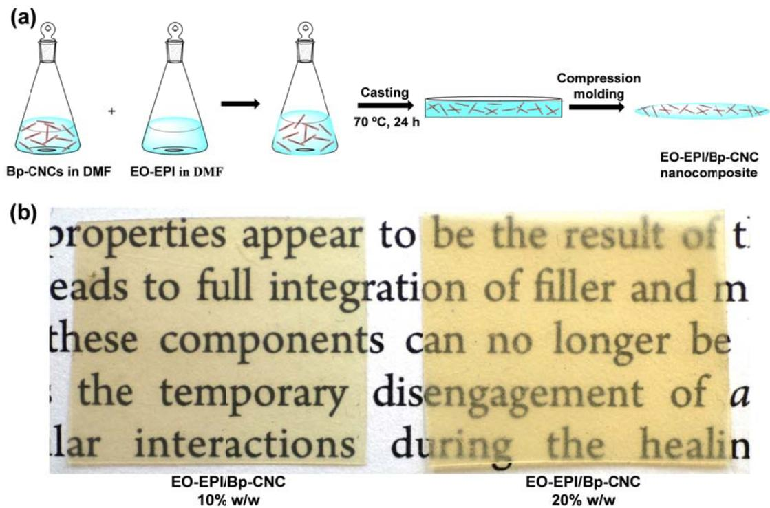
**SI-Fig. 6.** (a) Schematic representation of the process used to prepare EO-EPI/Bp-CNC nanocomposite films. (b) Pictures of compression-molded films of the nanocomposites.
