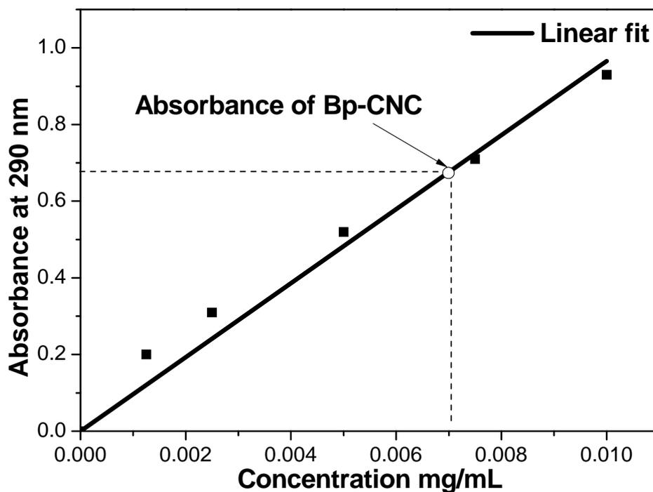
**SI-Fig. 4.** Plot showing the absorbance at 290 nm of Bp-NCO solutions as a function of Bp-NCO content (black, filled squares) and of a 125 µg/mL Bp-CNC dispersion (black, open circle). The data were used to determine the level of functionalization of Bp-CNCs.
