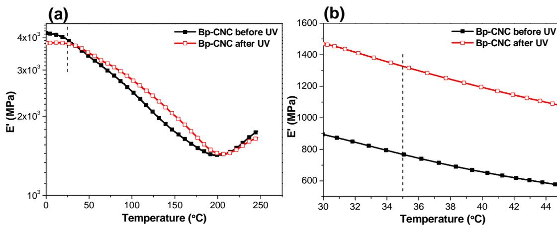
**SI-Fig. 5.** Dynamic mechanical analysis (DMA) traces of neat Bp-CNC films in the dry (a) and water-swollen (b) state, before (black curves) and after (red curves) exposure to UV light (302 nm, 8 W, 120 min, RT). Shown are plots of the storage modulus  $E'$  against temperature (note: in (a) Y axis is logarithmic and in (b) it is linear).
