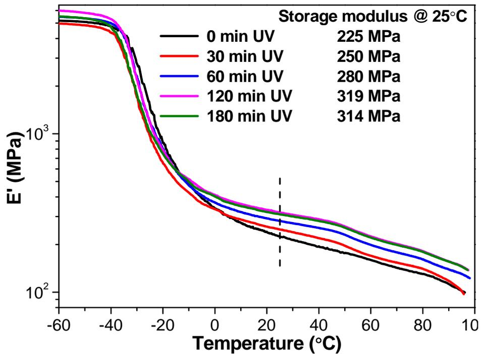
**SI-Fig. 10.** Dynamic mechanical analysis (DMA) traces of films of nanocomposites of EO-EPI and 10% w/w Bp-CNC as a function of UV irradiation time (302 nm, 8 W, RT). Shown are plots of the storage modulus  $E'$  against temperature.
