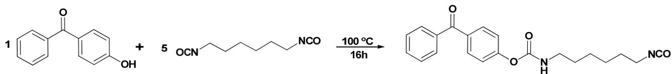
**SI-Scheme 1.** Reaction of 4-hydroxybenzophenone with hexamethylene diisocyanate.
