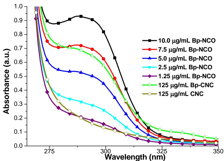
**SI-Fig. 3.** UV-Vis absorption spectra of dispersions of unmodified CNCs, Bp-CNC (125  $\mu\text{g/mL}$ ) in DMF and solutions of Bp-NCO in DMF (concentration = 1.25-10  $\mu\text{g/mL}$ ). As seen from the spectra, the Bp-CNC and Bp-NCO shows an absorbance with maximum around 290 nm, which is characteristic of the benzophenone derivative; this absorbance peak was absent in the spectrum of the unmodified CNCs.
