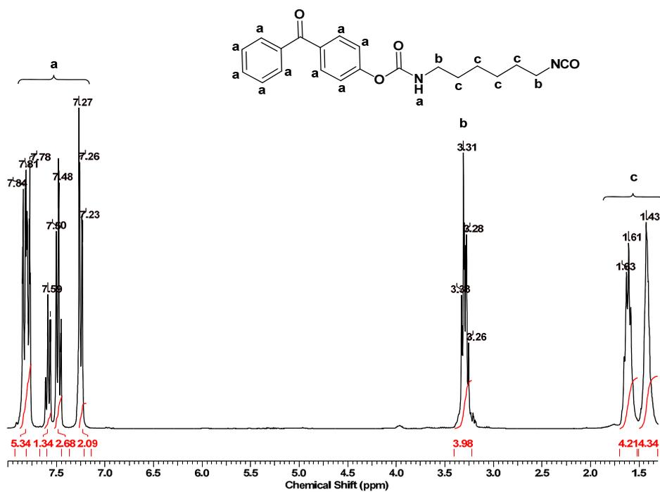
**SI-Fig. 1.**  $^1\text{H-NMR}$  spectrum of 4-benzoylphenyl (6-isocyanatohexyl) carbamate (Bp-NCO) in  $\text{CDCl}_3$ .
