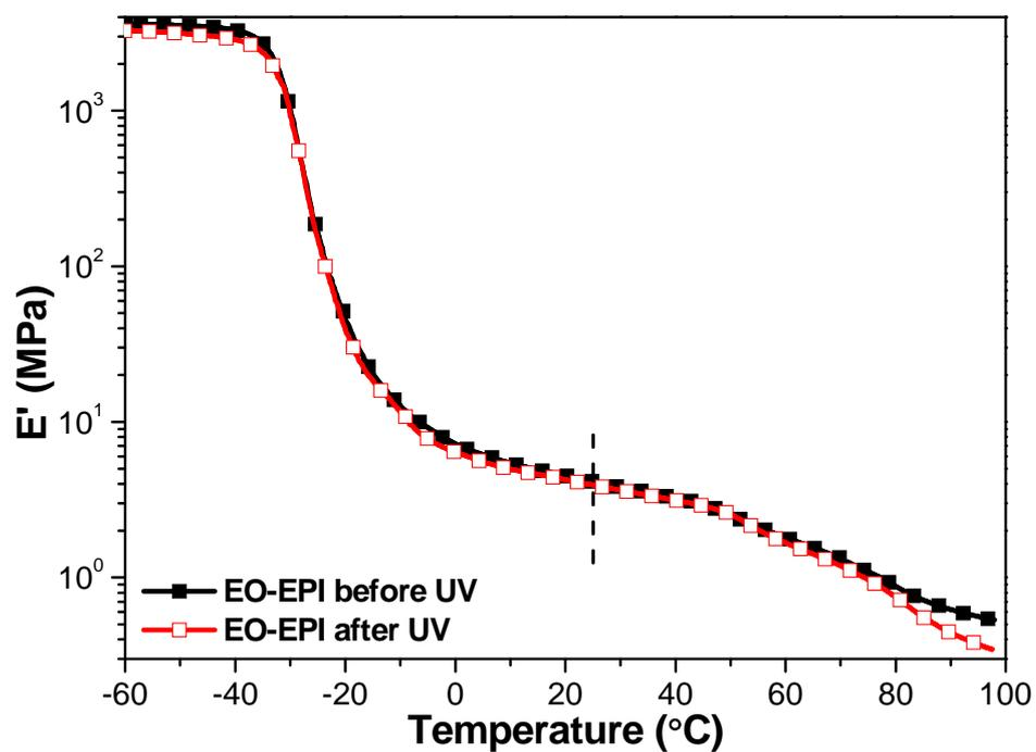
**SI-Fig. 9.** Dynamic mechanical analysis (DMA) traces of films of the neat EO-EPI before (black squares) and after (red squares) UV exposure (302 nm, 8 W, 120 min, RT). Shown are plots of the storage modulus  $E'$  against temperature.
