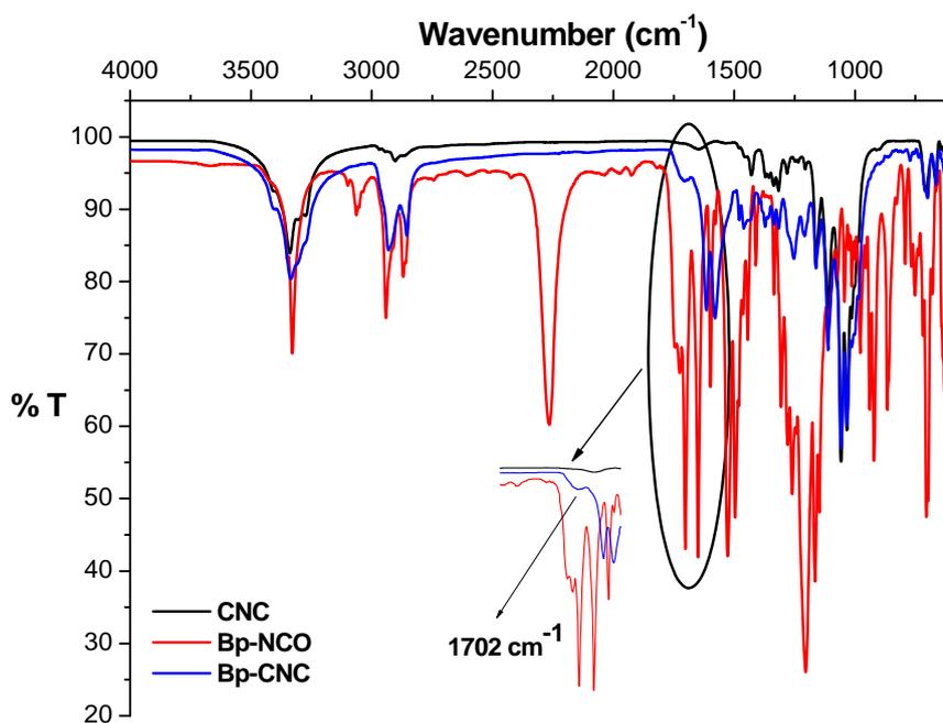
**SI-Fig. 2.** ATR FT-IR spectra of unmodified CNCs, Bp-NCO, and Bp-CNCs. The spectrum of Bp-CNCs shows a characteristic peak at  $1702\text{ cm}^{-1}$ , which corresponds to the urethane linkage after the reaction with Bp-NCO and is not observed in the spectrum of the neat CNCs. The spectrum also shows an increased transmission in the region of  $2800\text{-}2950\text{ cm}^{-1}$ , due to alkyl chain vibrations.
