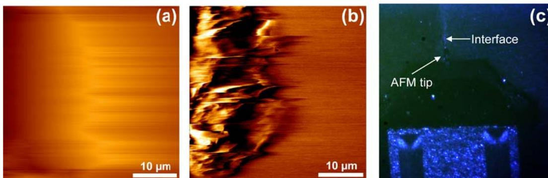
**SI-Fig. 8.** Atomic force microscopy (AFM) images in height (a) and amplitude (b) of EO-EPI/Bp-CNC 10% w/w nanocomposite mode, as well as the corresponding cantilever AFM tip image (c) at the interface of soft and stiff segment. Height image was not evident to differentiate the interface between the stiff and soft state while, amplitude image clearly shows the difference in morphology in stiff segment (left part) and soft segment (right part).
