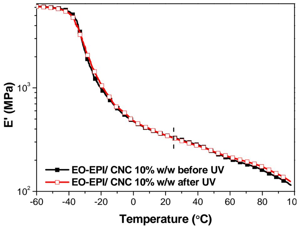
**SI-Fig. 11.** Dynamic mechanical analysis (DMA) traces of films of nanocomposites of EO-EPI and 10% unmodified CNCs, before (black squares) and after (red squares) exposure to UV light (302 nm, 8 W, 120 min, RT). Shown are plots of the storage modulus  $E'$  against temperature.
