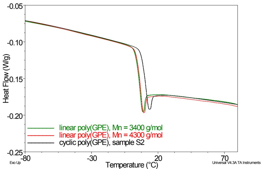
**Figure S6.** DSC profiles of cyclic and linear poly(GPE) specimens measured during heating at a rate of 10 °C/min.
