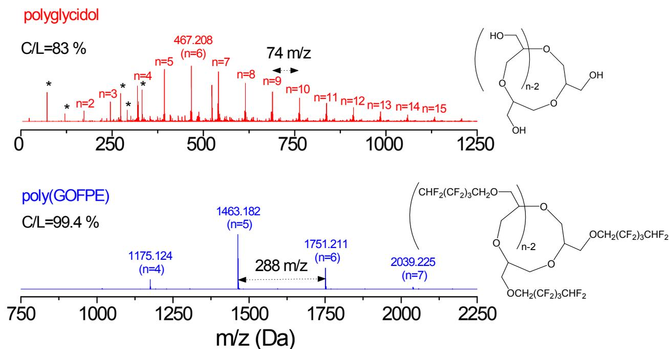
**Figure S7.** MALDI-TOF spectra of cyclic poly(glycidol) and cyclic poly(GOFPE). C/L values are included. \*Signals coming from the matrix.
