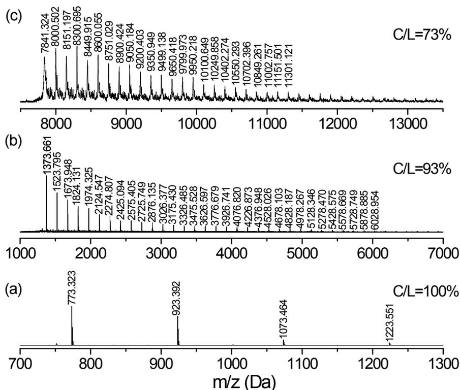
**Figure S4.** MALDI-TOF spectra of sample B in the low (a), medium (b) and high (c) molecular weight ranges. To acquire spectra (b) and (c), the ions below 1300 Da and 8000 Da were deflected. Spectra (a) and (b) were obtained by using NaI as the cationic ionization agent and detection in positive reflectron mode, as detailed in the experimental section. Instead, spectrum (c) was obtained by
