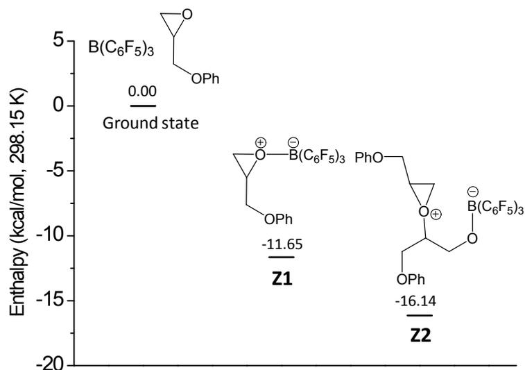
**Figure S5.** Enthalpy from DFT calculations for the zwitterionic intermediates Z1 and Z2 respect to free borane and GPE.
