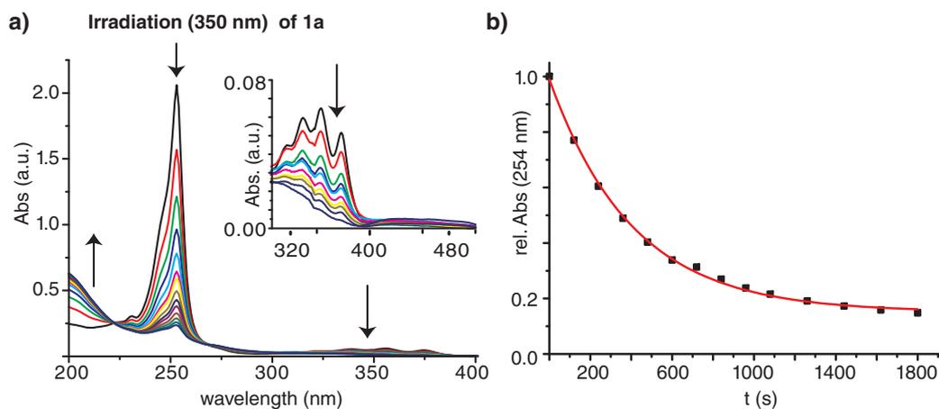
**Figure S12:** a) UV/vis spectra for **1a** (10  $\mu$ M in water) upon photoirradiation (350 nm). b) Normalised absorbance at 254 nm as a function of irradiation time. The solid red line shows the best monoexponential fit of the kinetic data.
