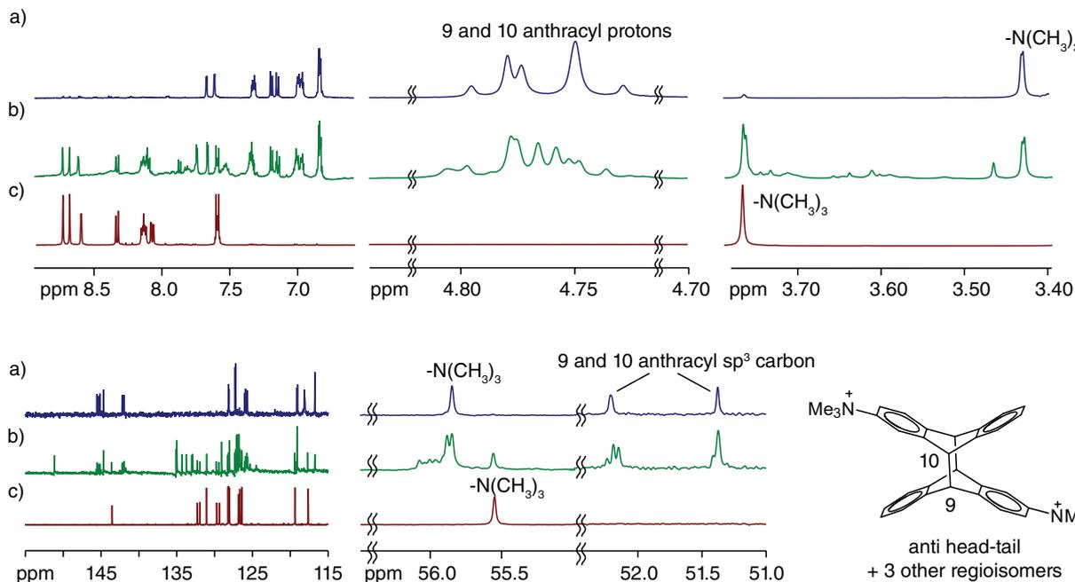
**Figure S14:** Top  $^1\text{H}$  and bottom  $^{13}\text{C}$  NMR spectra ( $d_6$ -DMSO) of a) anthracene-dimer that was prepared via photoirradiation (15 min) of a  $\text{CB}[8]\cdot\mathbf{1a}_2$  aqueous solution, followed by freeze drying and extraction of the photodimer with acetonitrile, b) a product mixture that was prepared via photoirradiation (3 h) of a  $\mathbf{1a}$  aqueous solution, followed by freeze drying, c) reference spectra for  $\mathbf{1a}$ .
