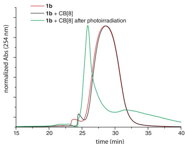
**Figure S21:** GPC elution curves (eluent: H<sub>2</sub>O) for **1b** upon addition of CB[8] and subsequent photoirradiation. The broad peak-shape is likely on account of aggregation in water and sticking to the GPC column.
