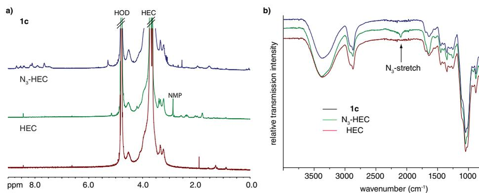
**Figure S2:** a)  $^1\text{H}$  NMR ( $\text{D}_2\text{O}$ ) spectra and b) FTIR spectra of commercial HEC (700,000 g/mol),  $\text{N}_3\text{-HEC}$  and **1c**.
