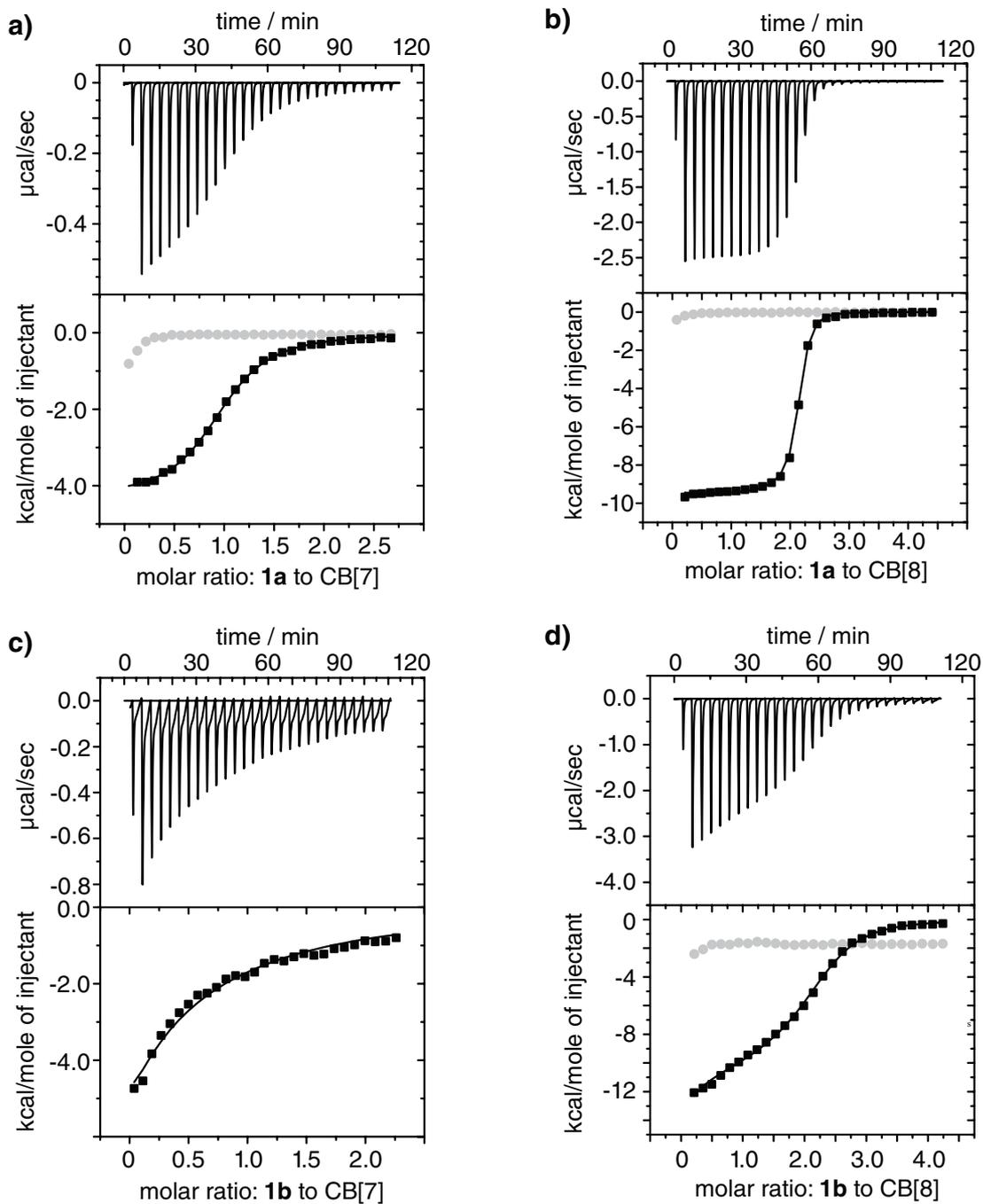
**Figure S10:** Representative isotherms for titration of a solution of **1a** or **1b** (0.5 - 1.0 mM) into an aqueous solution of CB[7] or CB[8] (40  $\mu$ M) at 25  $^{\circ}$ C. Integrated heats are shown as black squares, which were corrected for the heat of dilution (grey circles) prior to fitting of the isotherms to a 1:1 binding model in the case of CB[7] or a stepwise binding model in the case of CB[8].
