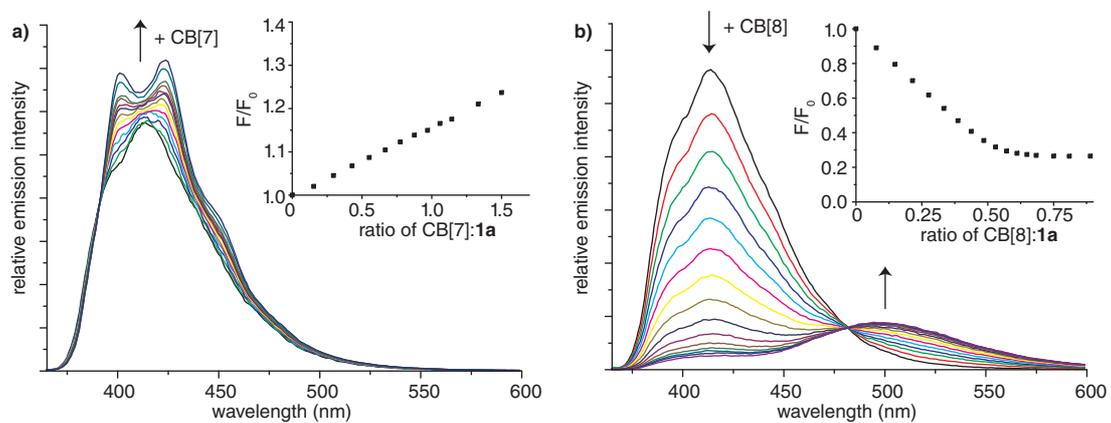
**Figure S9:** Emission spectra (356 nm excitation) for the titration of **1a** (10  $\mu$ M in water) with a) CB[7] and b) CB[8]. The inset shows the normalised total fluorescence as a function of the ratio of CB[*n*] to **1a**.
