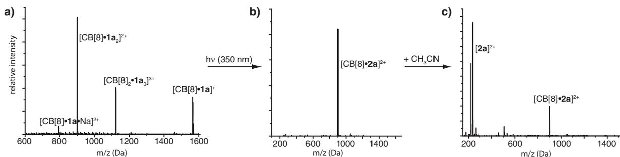
**Figure S15:** ESI-MS spectra of a 1:2 solution of  $\text{CB}[8]$  and  $\mathbf{1a}$  in water a) prior to and b) after photoirradiation for 15 min. c) Acetonitrile was added to the photoirradiated mixture to decomplex the ternary  $\text{CB}[8]$  complex and the ESI-MS spectrum was measured. Absolute charges were assigned through analysis of the isotopic pattern.
