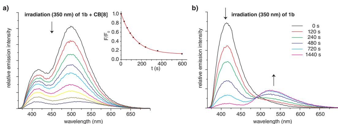
**Figure S20:** Emission spectra (356 nm excitation) upon photoirradiation (350 nm) of **1b** ( $10 \mu\text{M}$  in water) in a) the presence of 0.5 equiv. of CB[8] and b) the absence of the host. The inset shows the normalised total fluorescence as a function of the irradiation time. The solid red line shows the best monoexponential fit of the kinetic data.
