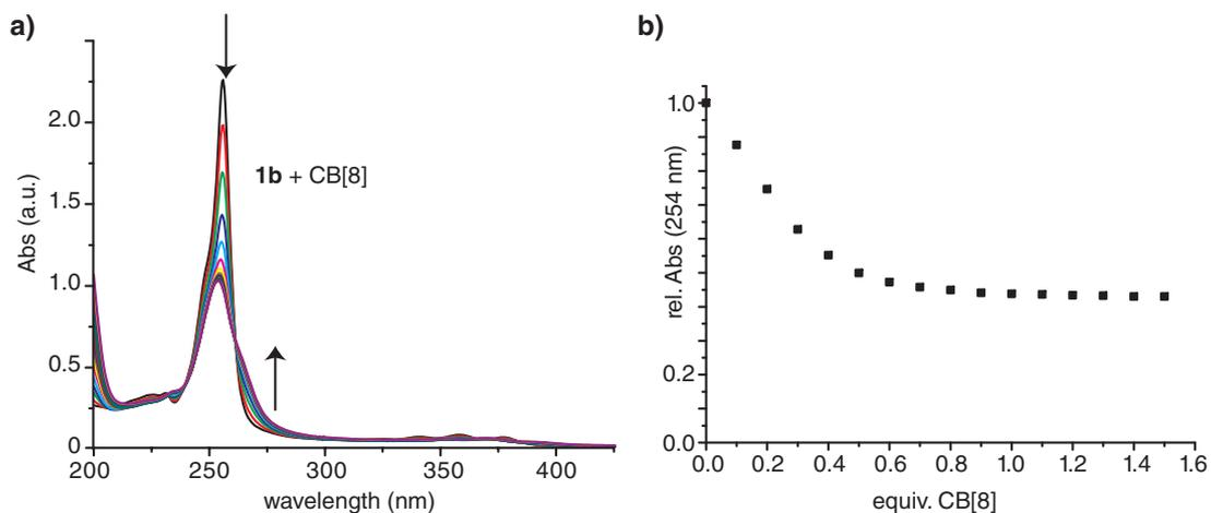
**Figure S17:** a) UV/vis spectra for the titration of **1b** (10 μM in water) with CB[8]. b) Normalised absorbance at 254 nm as a function of the CB[8] equivalents.
