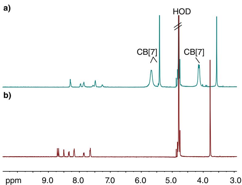
**Figure S7:**  $^1\text{H}$  NMR spectra ( $\text{D}_2\text{O}$ ) of **1a** (0.5 mM) in a) the presence of 1 equiv. of CB[7] and b) absence of the host.
