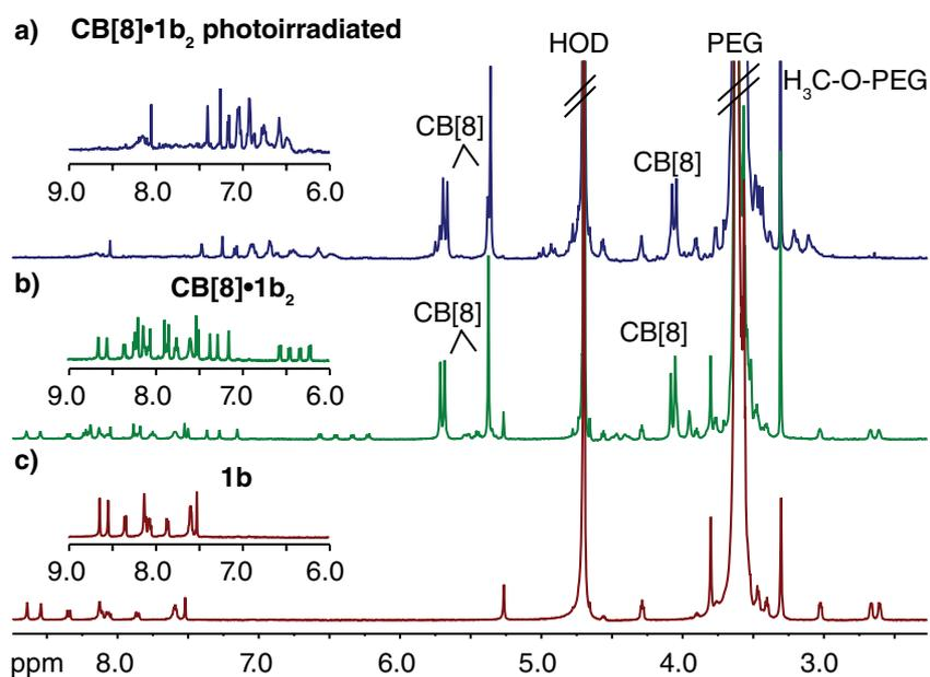
**Figure S22:** <sup>1</sup>H NMR spectra (D<sub>2</sub>O) of **1b** (0.5 mM) in the presence of 0.5 equiv CB[8] a) after photoirradiation for 30 min and b) prior to photoirradiation. c) <sup>1</sup>H NMR spectra (D<sub>2</sub>O) of **1b** (0.5 mM) in the absence of the host. The insets show the enlarged aromatic peak region.
