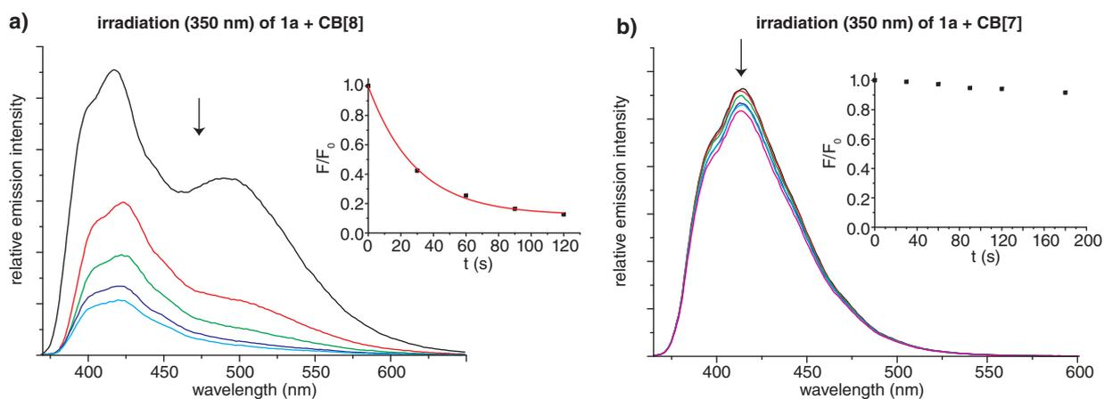
**Figure S11:** Emission spectra (356 nm excitation) upon photoirradiation (350 nm) of **1a** (10  $\mu$ M in water) in the presence of a) 0.5 equiv. of CB[8] and b) 1 equiv. of CB[7]. The inset shows the normalised total fluorescence as a function of the irradiation time. The solid red line shows the best monoexponential fit of the kinetic data.
