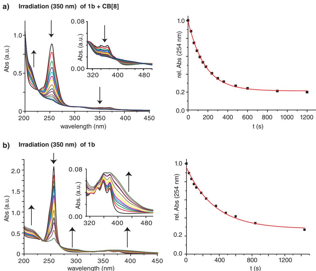
**Figure S19:** UV/vis spectra for **1b** ( $10 \mu\text{M}$  in water) upon photoirradiation (350 nm) in a) the presence of 0.5 equiv. CB[8] and b) in the absence of the host. The plot on the right shows the normalised absorbance at 254 nm as a function of irradiation time. The solid red line shows the best monoexponential fit of the kinetic data.
