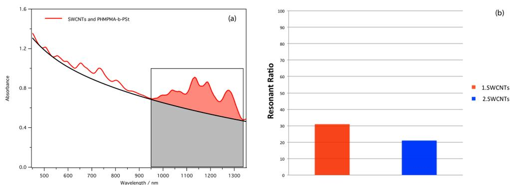
**Fig. S4.** a) Absorption spectrum of **1.SWCNT** with the resonant area (red) and non-resonant background (grey); b) Comparison between the resonant ratio of **1.SWCNT** (red) and **2.SWCNT** (blue).
