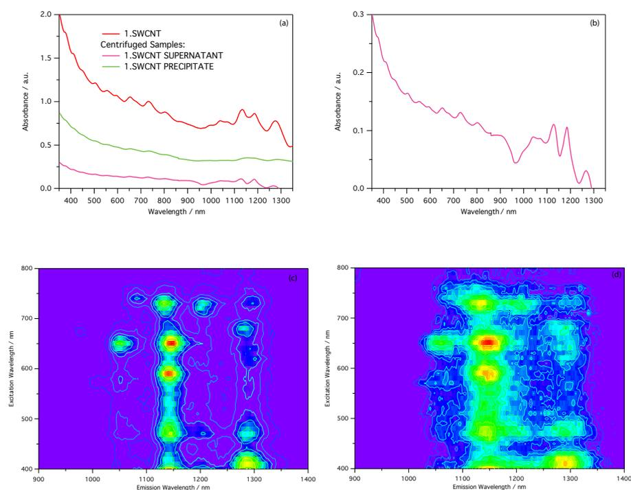
**Fig. S5.** a) Comparison between the absorption spectra of **1.SWCNT** as centrifuged and uncentrifuged samples. For the latter are reported both the spectra of the supernatant and of the precipitate. b) Magnification of the highly resolved and background free absorption spectra of the supernatant. (c) and (d) are the photoluminescence maps of the centrifuged samples of **1.SWCNT** as, respectively, supernatant and precipitate.
