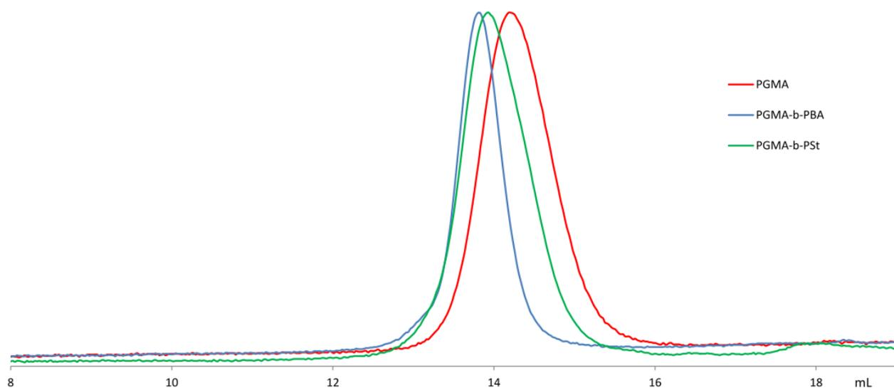
**Fig. S3.** GPC traces of PGMA macroRAFT (red line), PGMA-*b*-PMMA (green line), PGMA-*b*-PBA (blue line), PGMA-*b*-PSt (yellow line).
