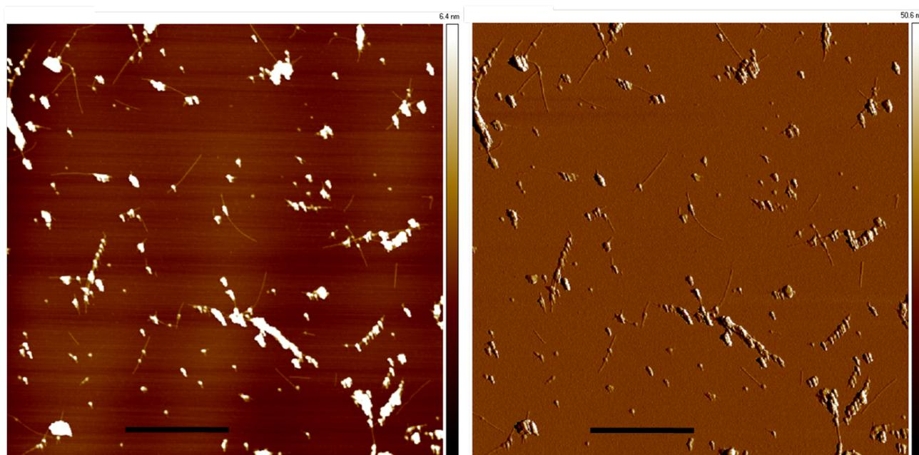
**Fig. S6.** AFM peak force mode of height (left) and peak force error (right) images of **1.SWCNT** deposited on mica supports after centrifugation (supernatant fraction), deposited on mica. Scale bars are 1  $\mu\text{m}$  in length.
