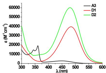
**Figure S3.** UV-vis absorption spectra of A3, D1 and D2 in dichloromethane.
