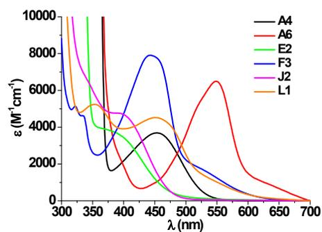
**Figure S5.** UV-vis absorption spectra of A4, A6, E2, F3, J2 and L1 in dichloromethane.
