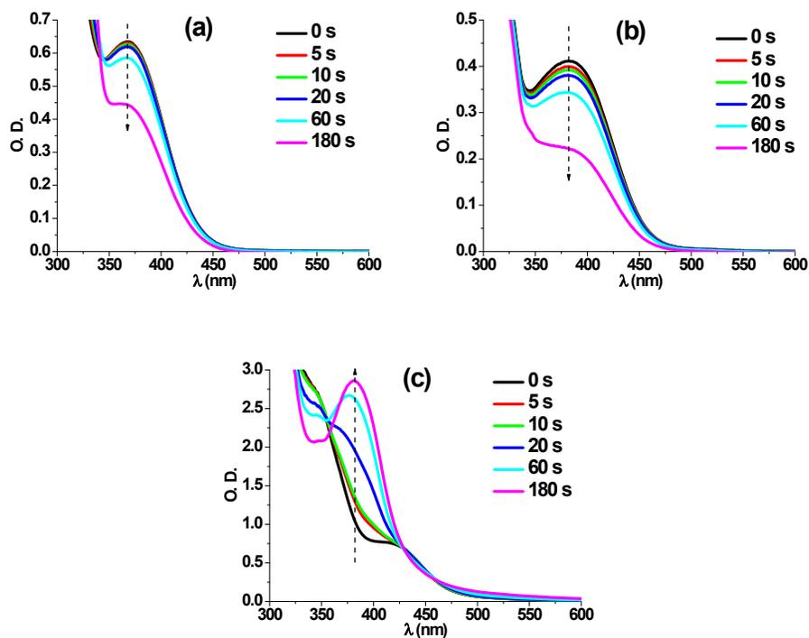
**Figure S8.** Steady state photolysis of (a) B2, (b) F2, and (c) K2 in the presence of Iod ( $[Iod] = 2.2 \text{ mM}$ ) in dichloromethane upon the laser diode at 405 nm exposure; UV-vis spectra recorded at different irradiation time.
