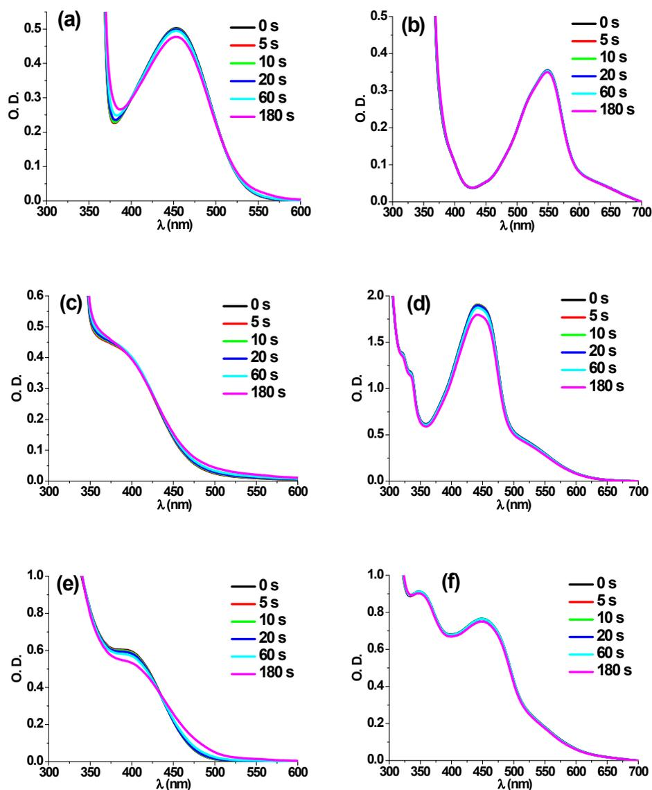
**Figure S6.** Steady state photolysis of (a) A4, (b) A6, (c) E2, (d) F3, (e) J2, and (f) L1 in the presence of Iod ( $[Iod] = 2.2 \text{ mM}$ ) in dichloromethane upon the visible light exposure; UV-vis spectra recorded at different irradiation time; A4, A6, F3, and L1 with the halogen lamp exposure; E2, and J2 with the laser diode at 405 nm exposure.
