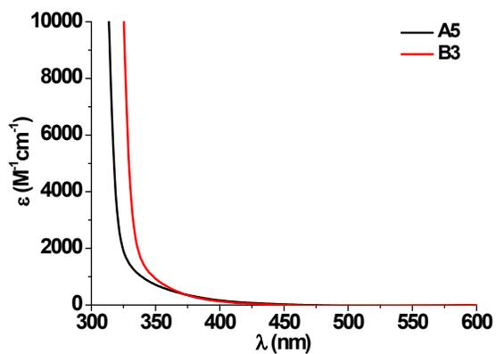
**Figure S2.** UV-vis absorption spectra of A5 and B3 in acetonitrile.
