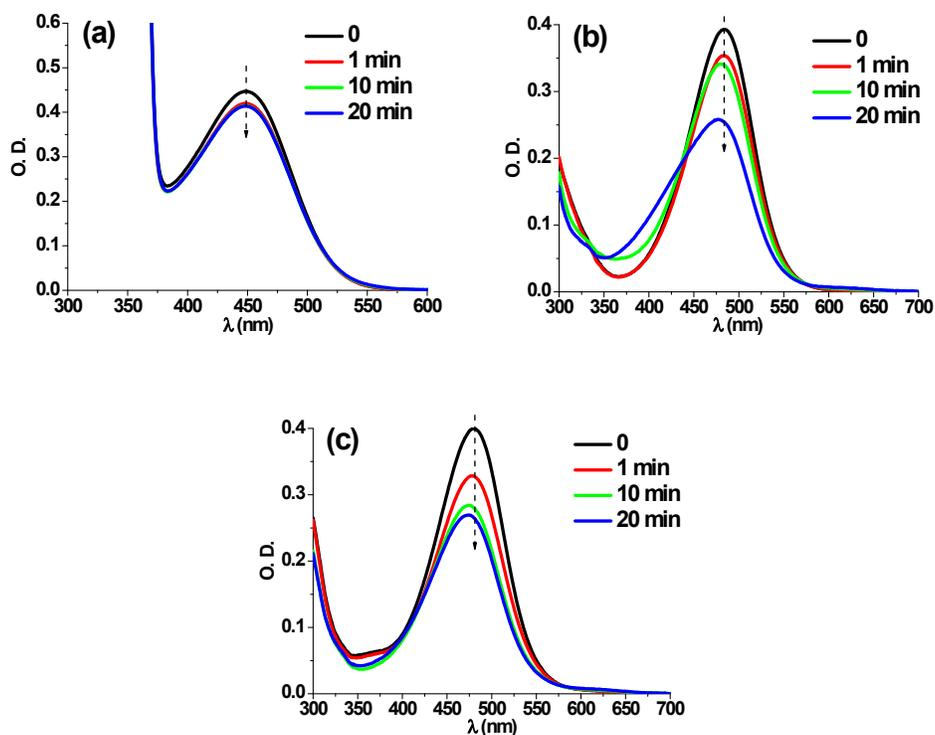
**Figure S4.** UV-vis spectra of (a) A3, (b) D1 and (c) D2 in dichloromethane after different irradiation time (halogen lamp).
