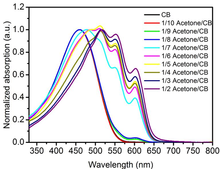
**Figure S1.** UV-Vis absorption spectra of **P3HT-*b*-P3IOAT** in chlorobenzene (10 mg/mL) with addition of various amounts of acetone (vol./vol.) and aged at room temperature for 14 h. All spectra were taken by diluting corresponding original solutions with identical mixed solvents to a final **P3HT-*b*-P3IOAT** concentration of 0.025 mg/mL.
